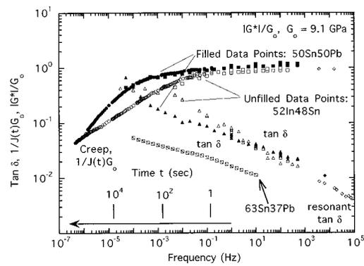
FIG. 3. Stiffness and  $\tan \delta$  vs frequency for wire 50Sn50Pb and cast 52In48Sn at 21 °C (shear modulus,  $G_0=9.1$  GPa for 50Sn50Pb at 1 Hz, 21 °C).  $\tan \delta$  vs frequency for 63Sn37Pb following Woirgard *et al.* shown for comparison.
