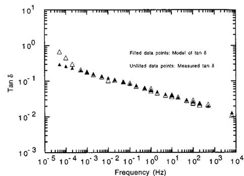
FIG. 6. Comparison of experimental results and  $\tan \delta$  model for 50Sn50Pb.
