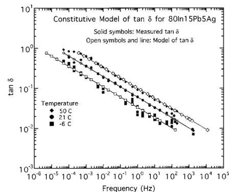
FIG. 4. Comparison of experimental results and shifted  $\tan \delta$  based on time-temperature superposition model for 80In15Pb5Ag at  $-6$ ,  $21$ , and  $50$  °C.
