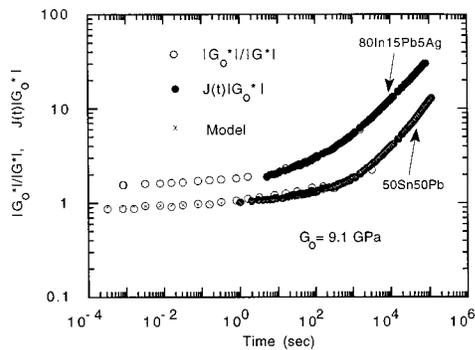
FIG. 7. Comparison of experimental results and the creep compliance model for 50Sn50Pb at 21 °C and 80In15Pb5Ag at 21 °C, both normalized to  $G_0 = 9.1$  GPa.
