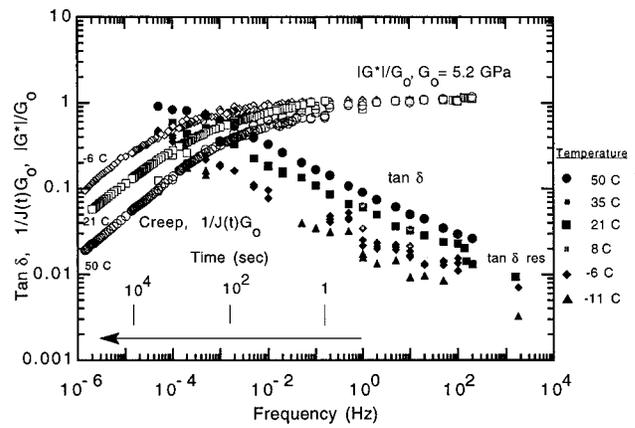
FIG. 2. Stiffness and  $\tan \delta$  vs frequency and temperature for 80In15Pb5Ag (shear modulus,  $G_0=5.2\text{ GPa}$  at 1 Hz,  $21\text{ }^\circ\text{C}$ ).
