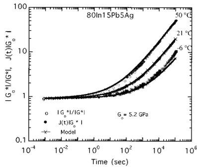
FIG. 5. Comparison of creep and dynamic modulus results and the creep compliance model for 80In15Pb5Ag at  $-6$ ,  $21$ , and  $50$  °C.
