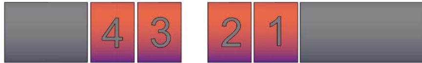
Figure 16. Drawing showing the sectioning for cross-sectional imaging and RCT of Zr-alloy tubes after the reflood tests. Sections 1-4 are numbered for.
