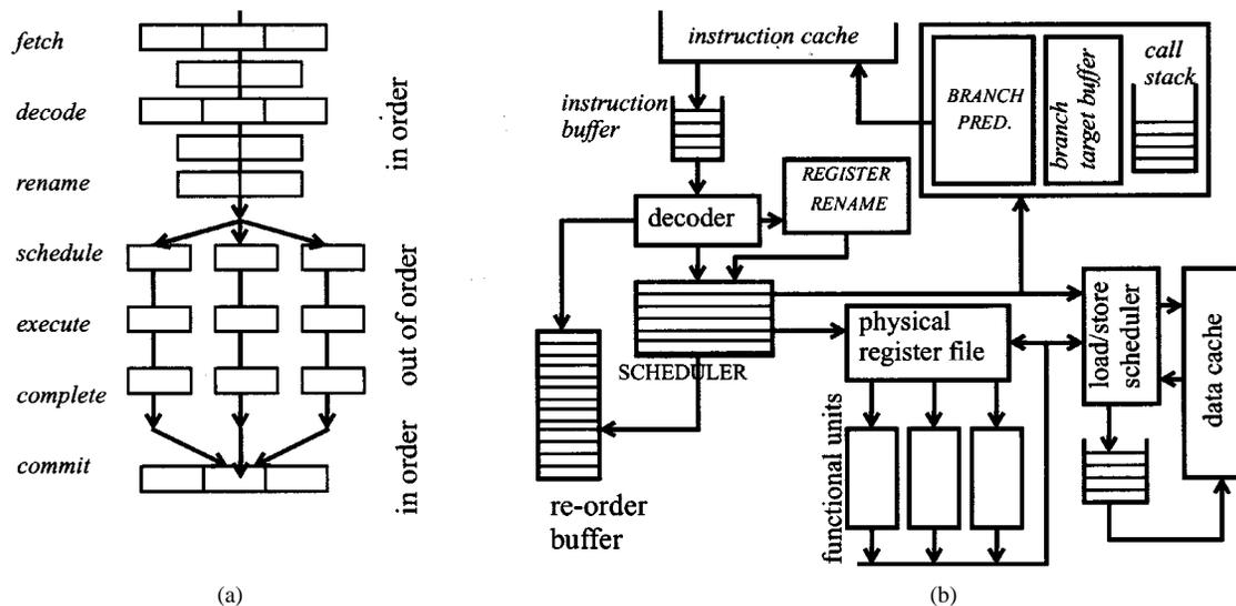
**Fig. 8.** Modern high-performance processor. (a) How execution progresses. Instructions are fetched, decoded, and renamed in program order. Multiple instructions are typically processed per cycle. Instructions are allowed to execute and complete in any permissible order based on operand and resource availability. Instructions commit in order. (b) Internal structure.
