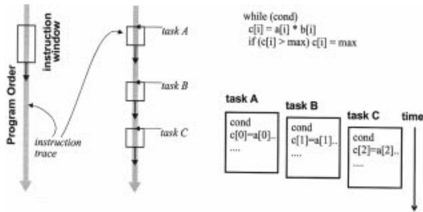
**Fig. 9.** The Multiscalar execution model. (a) Continuous, centralized instruction window (e.g., typical dynamically scheduled superscalar). (b) Multiscalar's way of building a large instruction window. (c) A loop. (d) How this loop may execute under the Multiscalar execution model.
