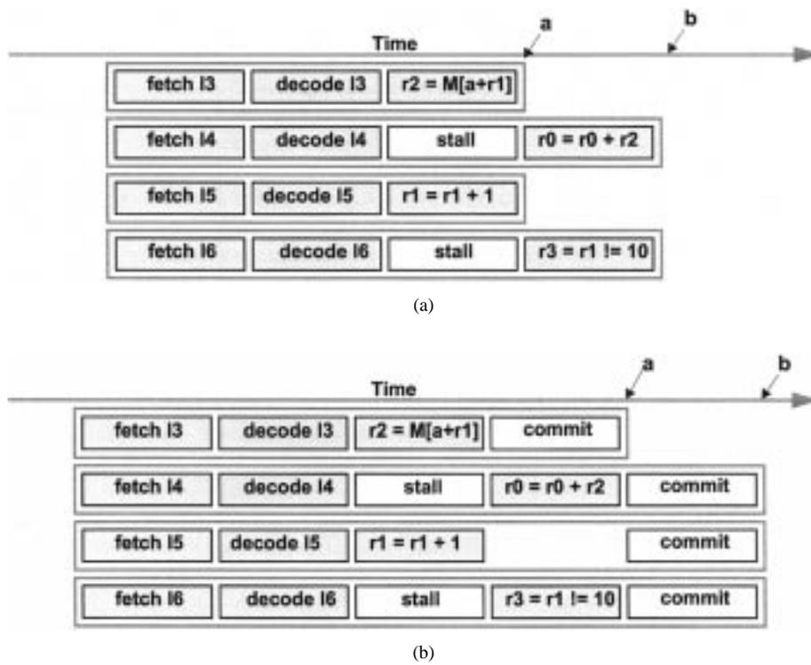
**Fig. 4.** Out-of-order execution: (a) I3 and I5 execute in parallel. I4 and I6 have to wait for I3 and I5 respectively. Nevertheless, I4 and I6 also execute in parallel. (b) Introducing a commit stage to preserve sequential semantics.
