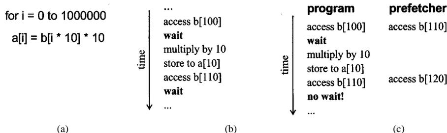
**Fig. 6.** (a) A code with regular array accesses. (b) Memory access timing without prefetching. Requests are not overlapped. (c) Prefetching requests the next array element while the previous request is still in progress. Request processing is overlapped and as a result overall throughput is increased. Notice that it still takes the same amount of time to fetch each individual array element.
