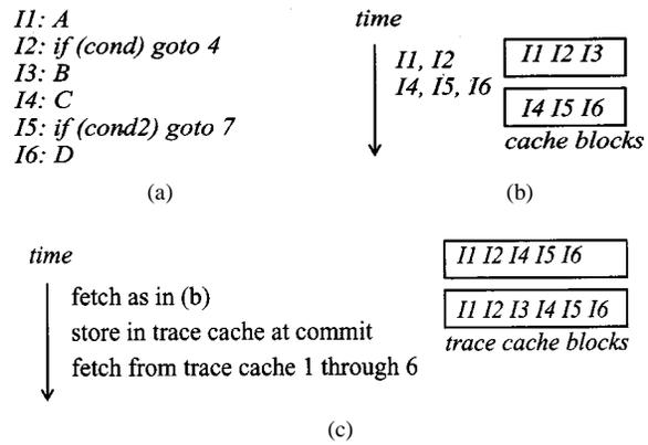
**Fig. 7.** Trace cache: predicting and fetching multibranch instruction sequences per cycle. (a) Code snippet. (b) Predicting and fetching in a conventional processor. We are limited to one prediction per cycle. Moreover, we are restricted to accesses within a single cache block. (c) Execution with a trace cache and trace cache entries.
