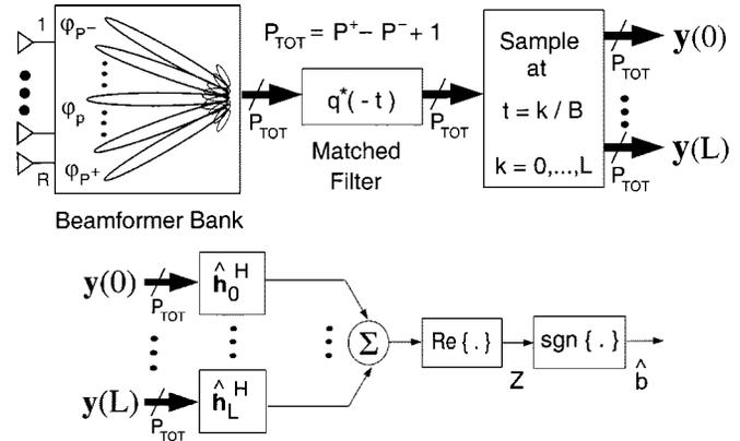
Fig. 5. Space–time RAKE receiver.
