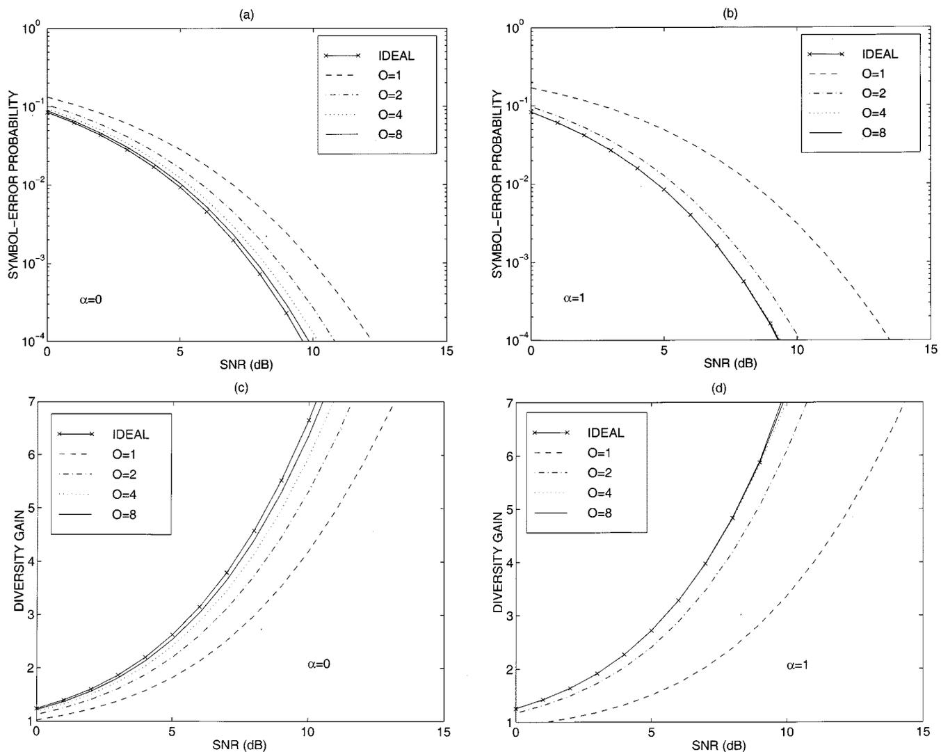
Fig. 7. Coherent space-time processing raised-cosine chip waveform: ideal versus canonical with (a)  $P_e$  for  $\alpha = 0$  (rectangular), (b)  $P_e$  for  $\alpha = 1$ , (c) diversity gain for  $\alpha = 0$ , and (d) diversity gain for  $\alpha = 1$ .
