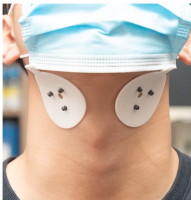
Figure 3. The placement of the electrodes
