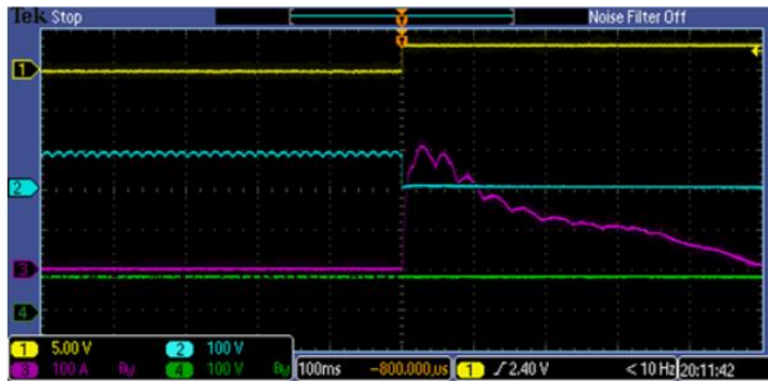
Figure 5. Ch1: Gate Signal. Ch2: DC bus voltage. Ch3: DC bus current. Ch4: Capacitor voltage.
