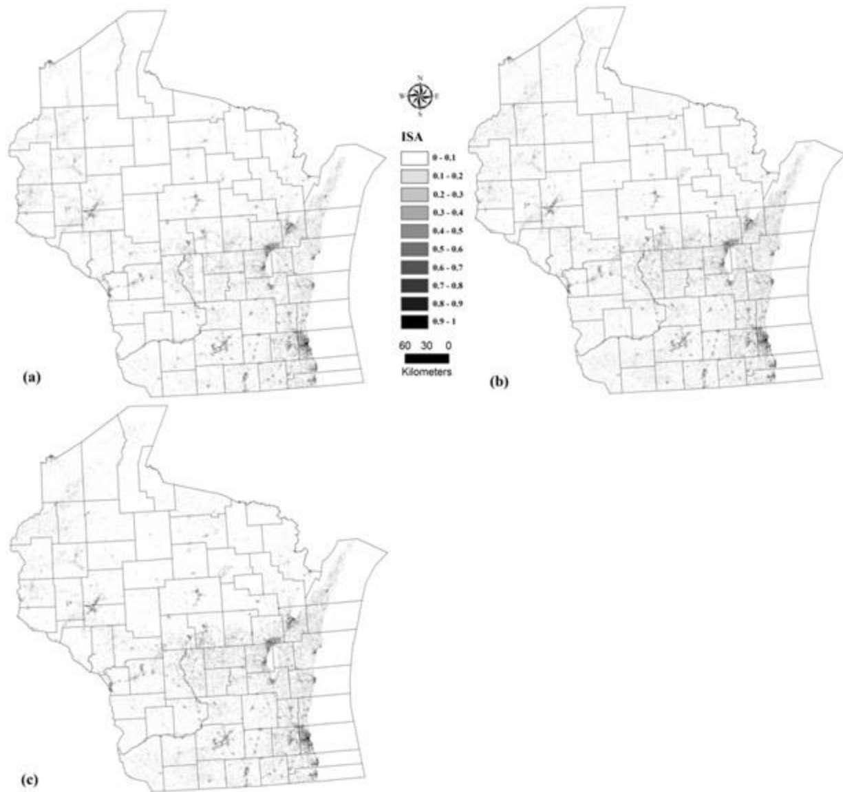
Figure 13 Impervious surfaces fraction maps generated from (a) proposed TMA method (b) simple TMA method and (c) METMA method
