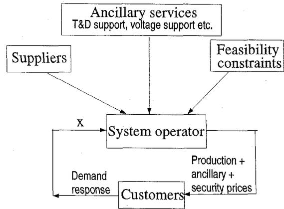
Fig. 2: Feedback process for the PoolCo model.
