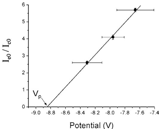
FIG. 3. Ratio of emitted to collected saturation current vs the inflection point in an electron-free sheath.
