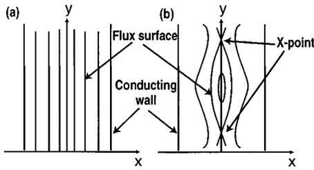
FIG. 1. Magnetic flux surfaces for two equilibria: (a) initial one-dimensional equilibrium. (b) Final two-dimensional equilibrium with island.
