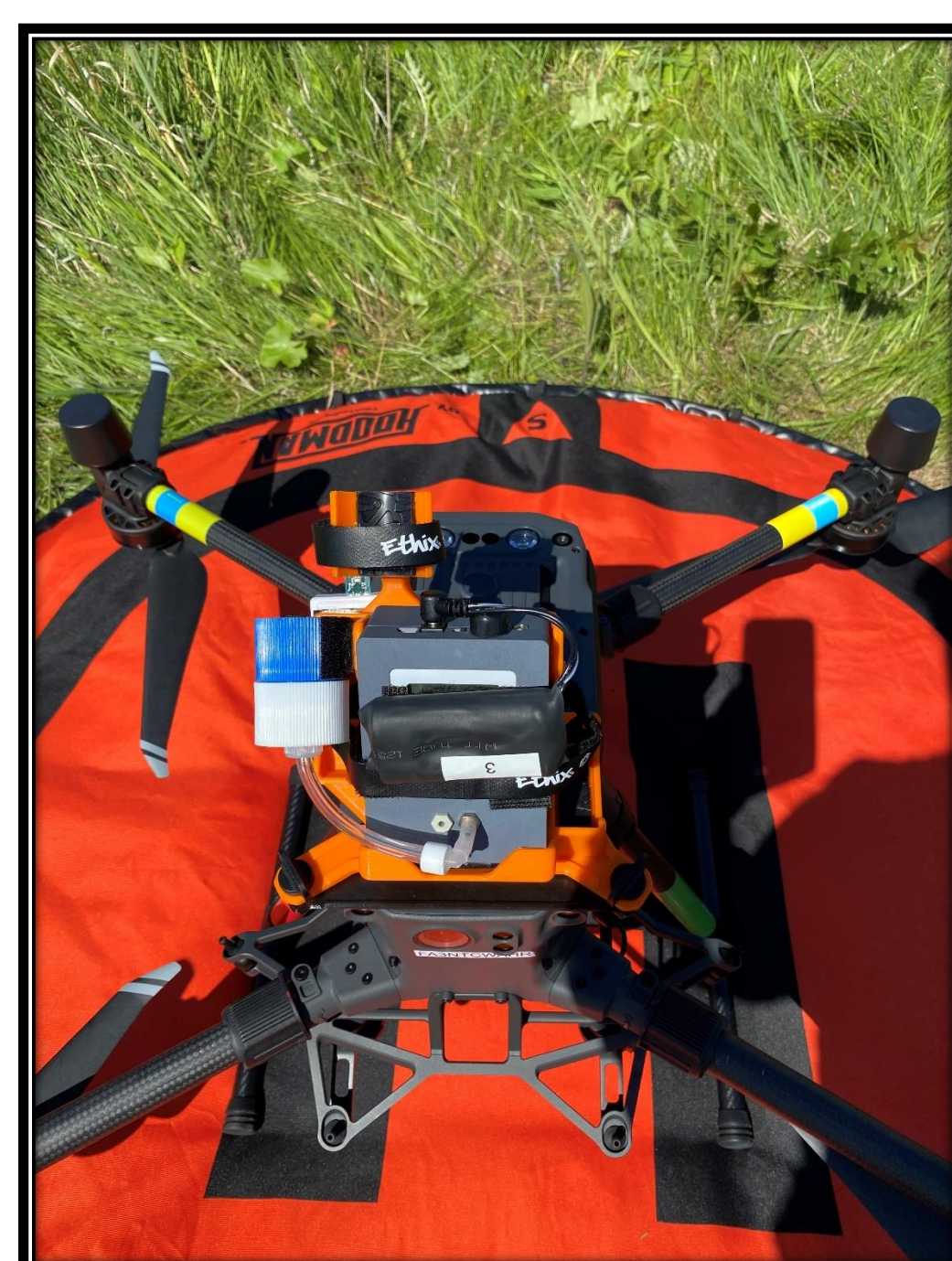
Figure 5: DJI M300 Drone equipped with a 3-d printed holder for attachment of POM device (Gray box, pictured with Blue/White filter inlet attached)
