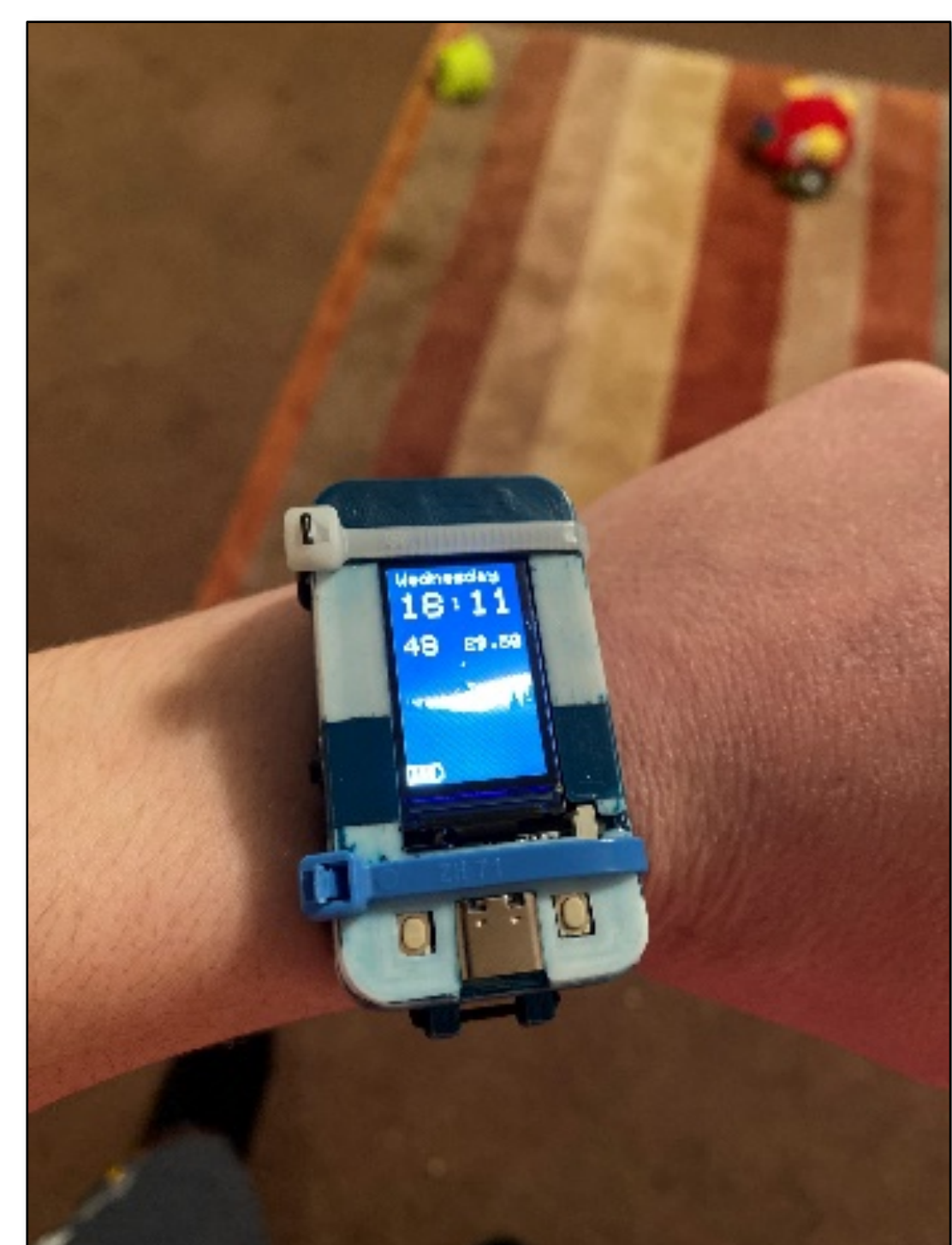
Photo of smartwatch on wrist; prior to gluing, held together by zip-ties
