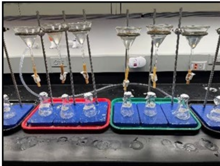
Figure 2. Density separation apparatus. Apparatus is composed of glass funnel attached to rubber tubing, with a plastic pinch clip to control flow. Apparatus is attached to ring stand and topped with glass watch glass. Photo by Sam Munk.
