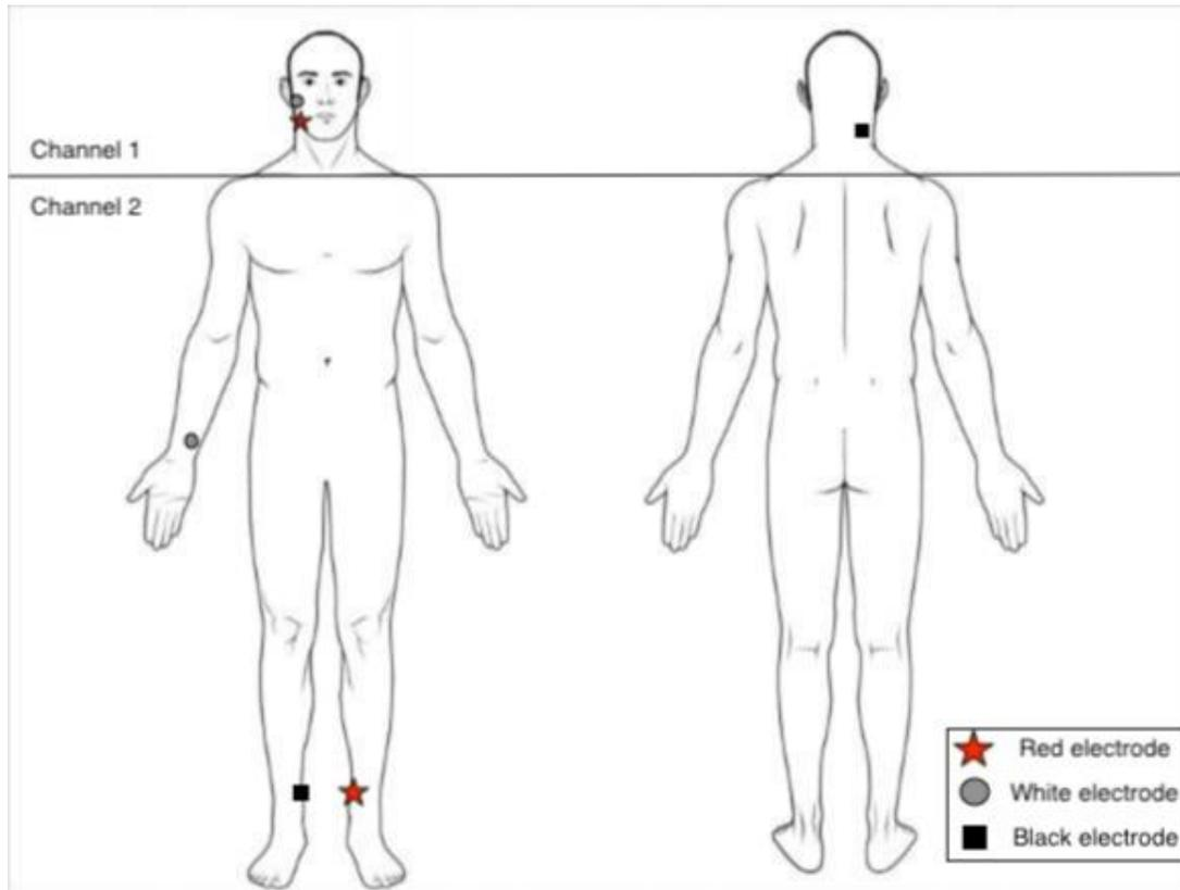
**Figure 1.** A depiction of the correct placement of electrode disks and their corresponding electrode connections. Channel 1 is related to the EMG measurements, while channel 2 is related to ECG measurements.
