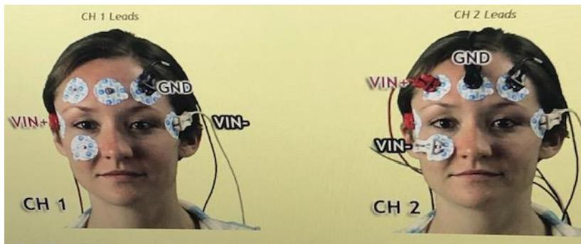
**Figure 4:** EOG electrode and channel placements on participant.
