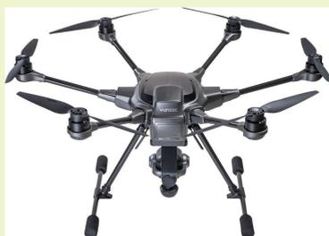
Above is a photo of the unmanned aerial system that we will be integrating the following three sensors onto. It is the Typhoon H hexacopter. The challenge will be finding enough space on Typhoon to fit all the sensors and, if need be, their battery packs. The last step of all the timelines is a full flight test. This will entail that all the sensors are on the Typhoon and collection data.
