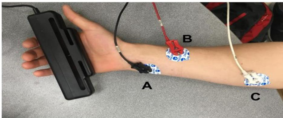
**Figure 2.** Example electrode setup for a right-handed subject. The black lead was connected to electrode A, the red to electrode B, and the white to electrode C.
