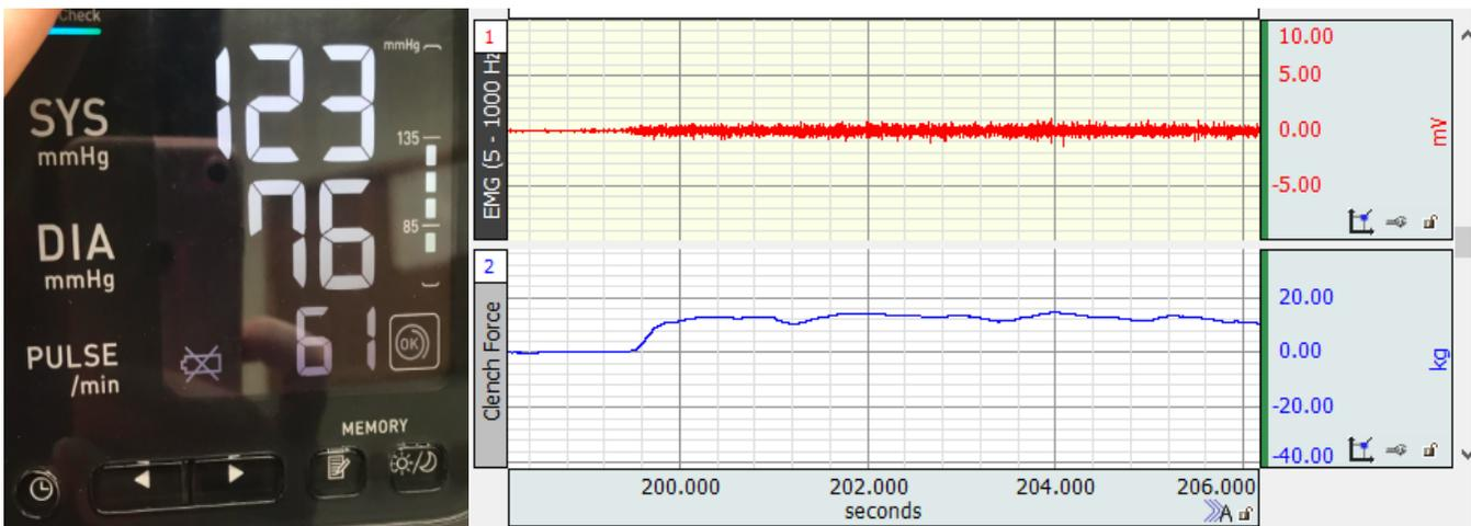
**Figure 4.** Positive control showing that each machine measures its intended metric in pilot testing. On the left, heart rate was monitored. On the right, EMG and clench force were measured during clenching.
