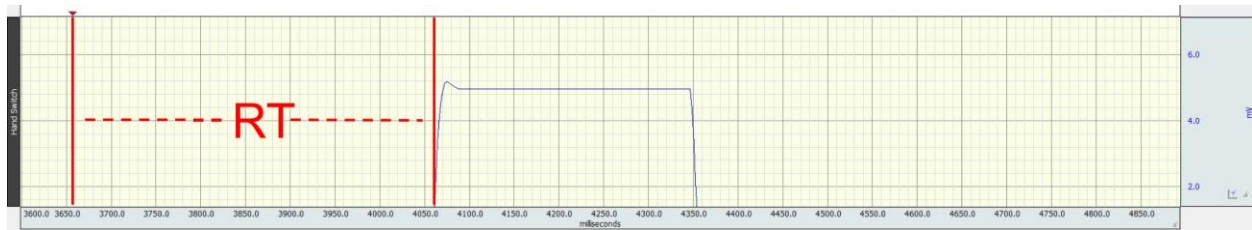
Figure 4. BIOPAC reaction time interface. Reaction time was measured as the time between the presentation of the auditory stimulus and the initial pressing of the hand switch button by the participant.
