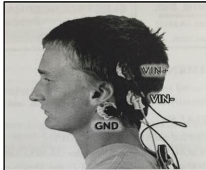
**Figure 4** The placement of the three electrodes on each participant can be seen. There were three electrodes: Vin+, Vin-, and GND. All three are placed on the participant’s head. These electrodes were used to collect theta and delta waves data via EEG.
