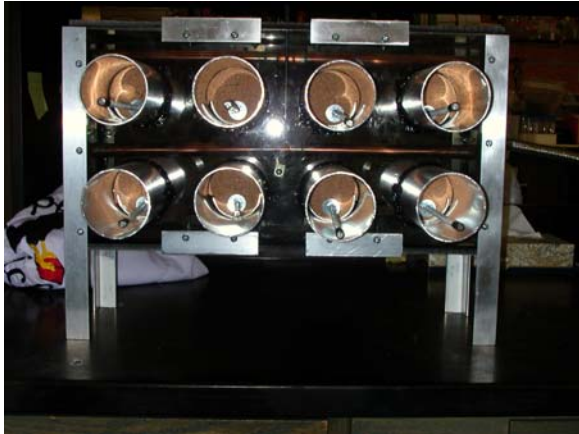
Figure 1; Front view of the feed steamer where all trials were conducted. The chamber contains individual sampling areas so samples do not contaminate each other.
