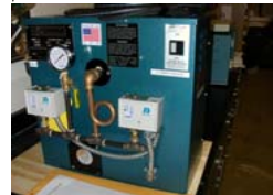
Figure 2: Electric steam generator that provided steam in all trials
