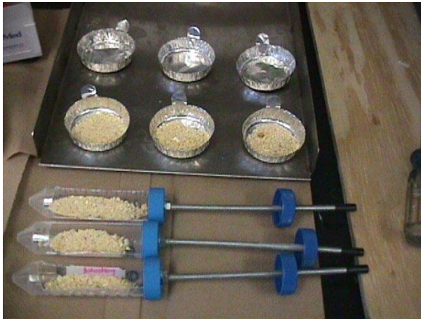
Figure 4; Individual sampling trough and freeze dry trays. Sampling troughs slide into the larger sampling trough as seen in figure 1.
