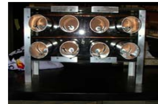
Figure 1, Engineering students collaborated with Mark Cook's lab to build a small-scale steam treatment chamber in order to develop a curve modeling Ab denaturation.
