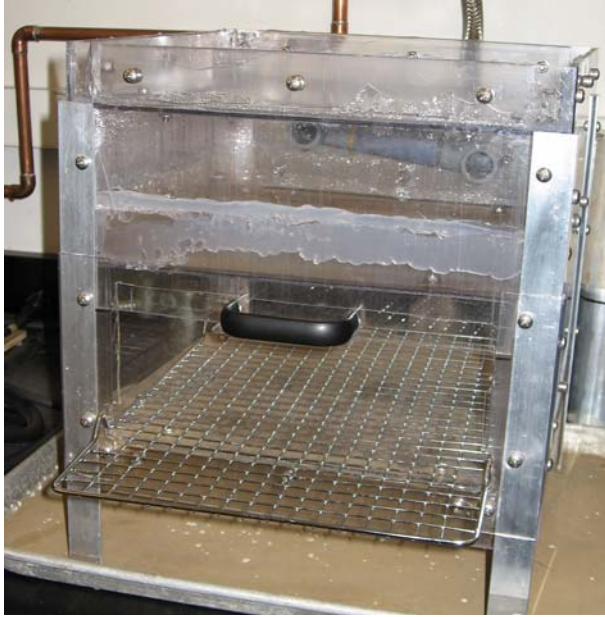
Figure 4: Close-up of steam chamber. There are two levels; steam enters the chamber in the top level and is applied evenly to samples on the lower level via holes chamber divider. This division ensures even application and prevents condensation from dripping directly onto samples during steam treatment. Samples are placed on a wire cookie sheet and slide into the bottom level for treatment.
