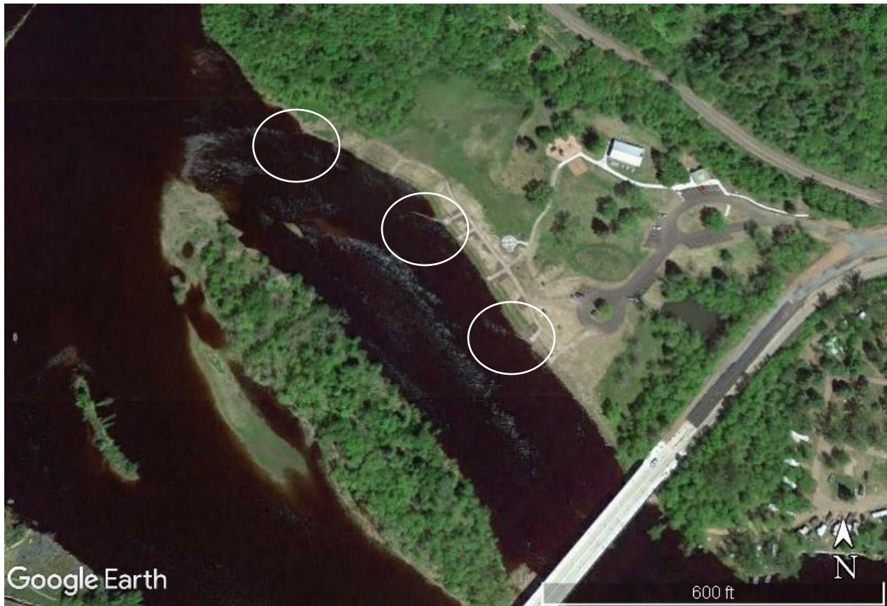
Figure 3.4. Ariel imagery depicting Chambers Grove habitat rehabilitation site on the St. Louis River near the Highway 23 bridge (bridge in photo). White circles represent areas of wing dam construction.
