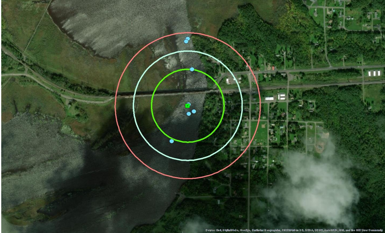
Figure 3.7. Example of mobile tracking range testing. VRTX receiver (green square) and detection points (blue circles). Green buffer is equal to 200 meters from VRTX receiver, White buffer is equal to 300 meters from receiver. Red buffer is equal to 400 meters from receiver. Sentinel tag in VRTX receiver was detected beyond 350 meters using omnidirectional hydrophone and VR-100 mobile receiver.
