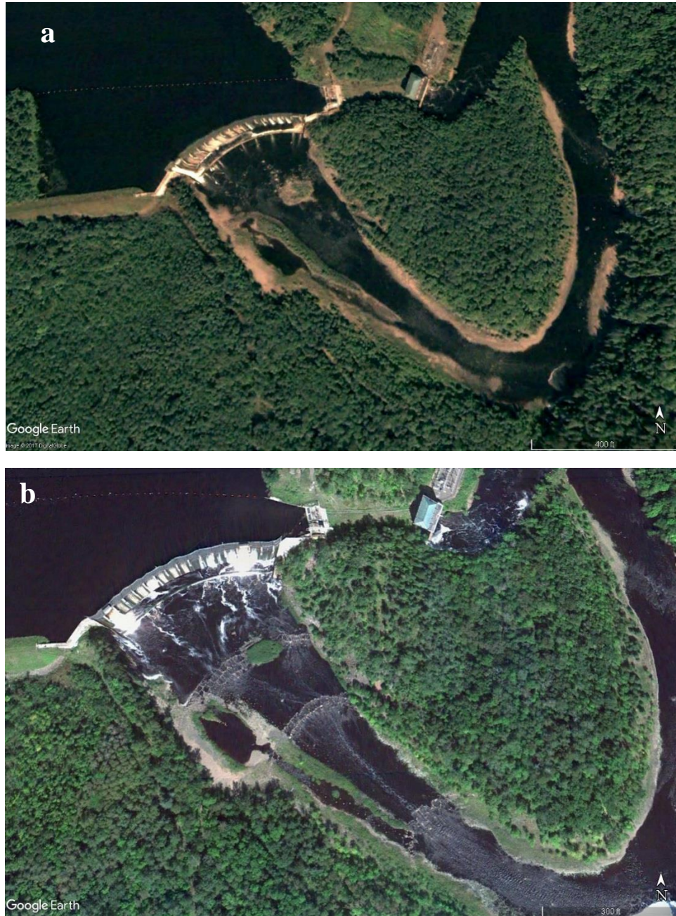
Figure 1.1. Aerial photographs of Fond Du Lac Dam on the St. Louis River pre-restoration (a) and post-restoration (b) of Lake Sturgeon Spawning habitat. Several rock weirs consisting of boulders added in 2009 to increase the area of suitable spawning habitat.
