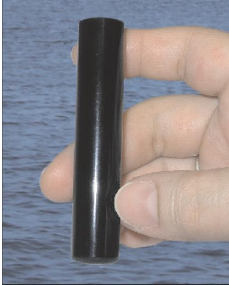
Figure 3.9. Vemco©V-16 Transmitter with a battery life of approximately 10 years and a nominal delay of 120 seconds \pm 50%. Transmitters were surgically implanted into the body cavity of Lake Sturgeon.
