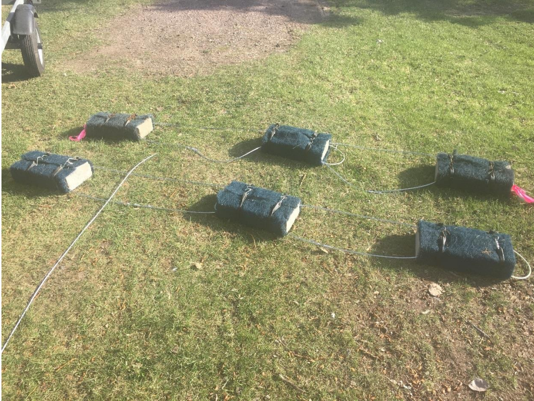
Figure 3.11. Egg mats for capturing Lake Sturgeon eggs. Egg mats consist of a cinder block wrapped with furnace filter and secured with bungee cords. Egg mats were cabled together in gangs of 2 or 3 depending on area placed.
