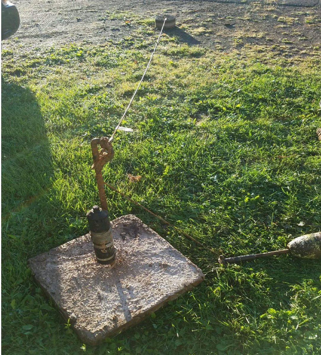
Figure 3.5. Anchor stand for placement of Vemco© VR2W acoustic receivers in the SLR and Western Lake Superior. A section of one-quarter inch steel cable, of a length equal to or slightly longer than the depth measurement at which the receiver will be placed, is connected between the anchor stand (near in photograph) and the small anchor (distant in photograph). An acoustic receiver is then mounted to the anchor stand vertically using hose clamps and duct tape.
