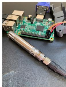
The HMP60 is a relative temperature and humidity probe
