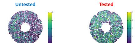
In the untested sample, each petal (the six groups the wires are divided into) has a similar amount of contact between wires.
