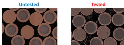
The area between the wires of the untested sample is very clear and free of debris.
