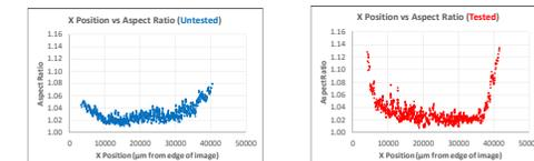
In the untested sample, the aspect ratio of the wires is slightly higher near the sides of the cable since the wires are twisted in the cable, creating a more oval cross-section for wires that are nearer to the edges of the cable.
