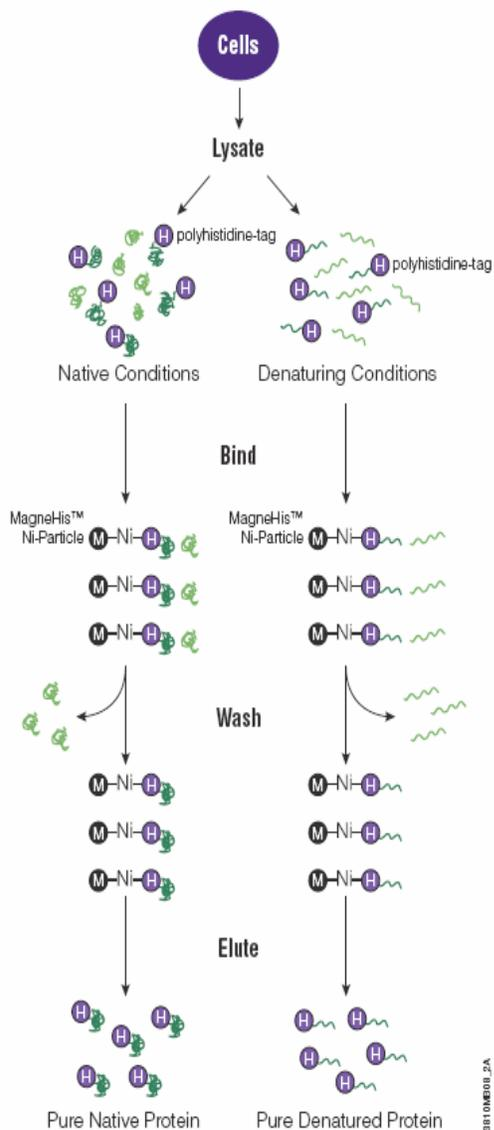
Figure 1: Diagram of Immobilized Metal Affinity Chromatography using a histidine tag and a nickel ion column (Promega Corporation, 2007).
