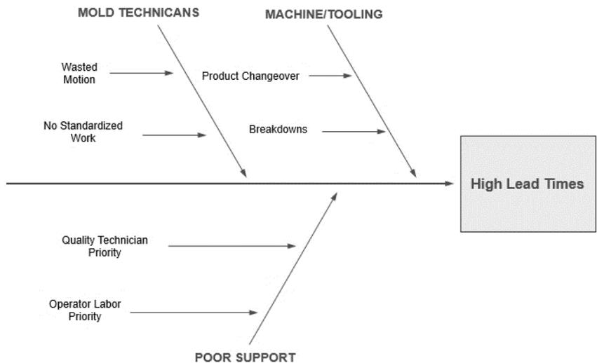
*Figure 13.* Fishbone diagram for high lead times.
