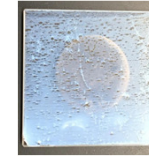
Sintered Sample that was slip casted at 800 C
