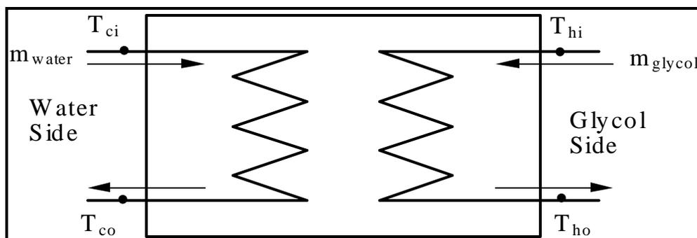
Figure 4.3.3 Heat Exchanger Energy Balance
