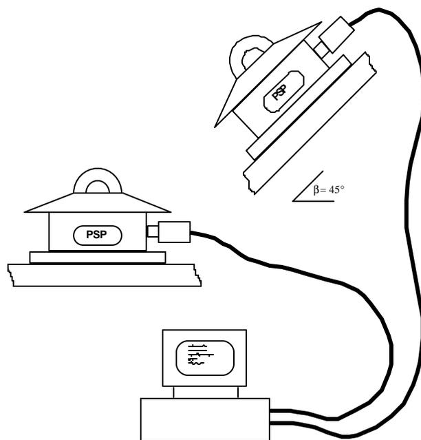
Figure 3.1.1 Solar Radiation Recording With Eppley Pyranometers
