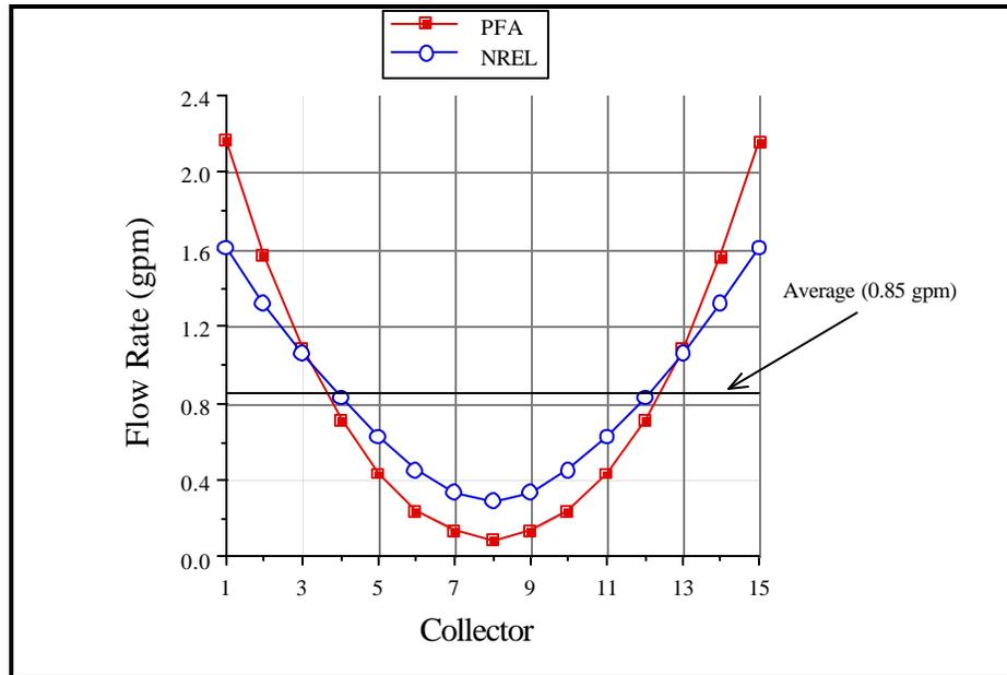
Figure 2.4.2 Flow Distribution Without Bend Loss Coefficient
