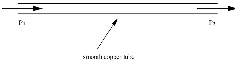
Figure 2.3.1 Pressure Drop in Copper Tube Riser
