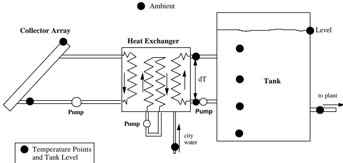
Figure 3.1.2 Plant Temperatures and Tank Level
