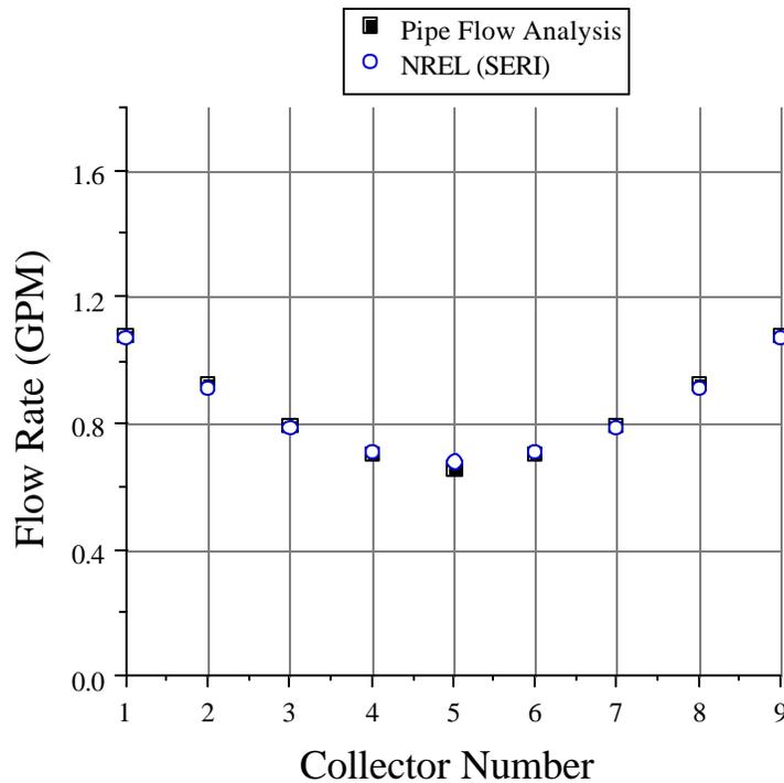
**Figure 2.4.6 Flow Distribution for 9 Collectors at Design Flow Rate**
