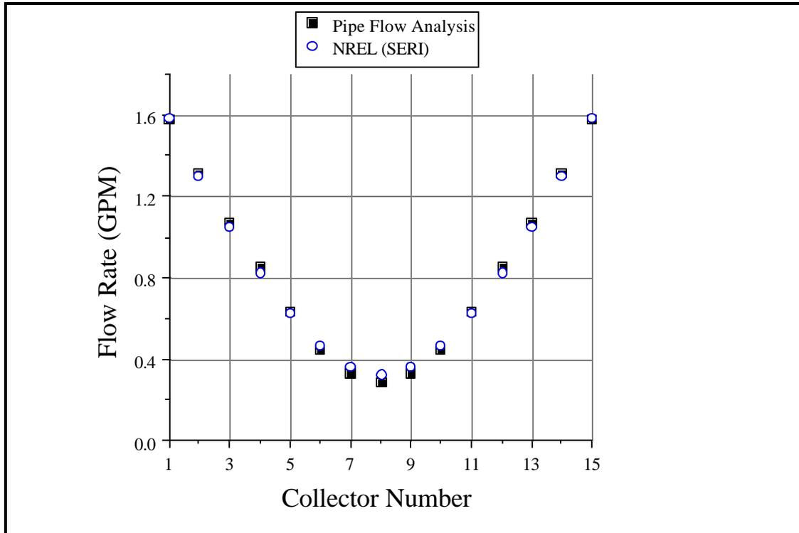
Figure 2.4.5 Flow Distribution for 15 Collectors at Design Flow Rate
