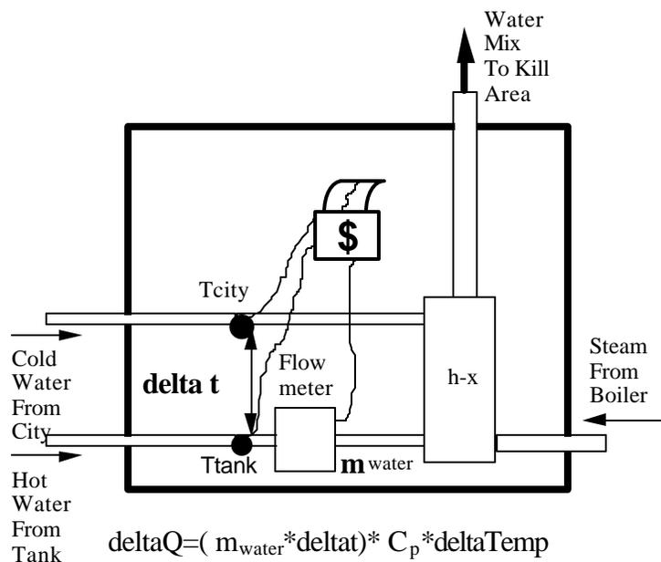
Figure 1.2.1 In Plant Energy Monitoring
