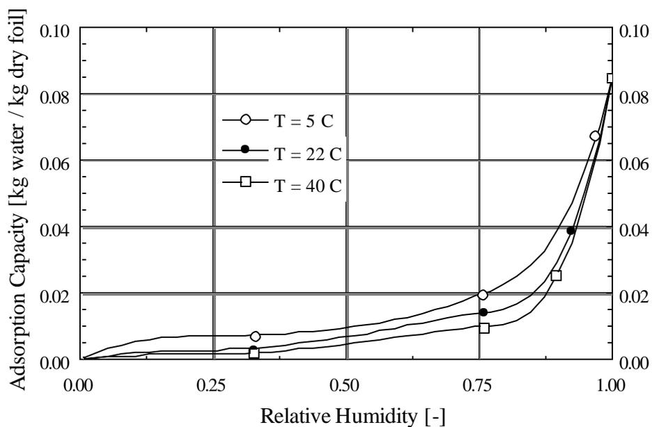
**Figure 3.3:** Equilibrium Adsorption Isotherms of Water-Based Desiccant
