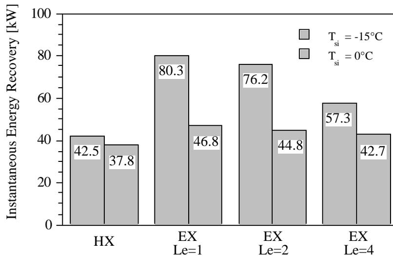
**Figure 5.14:** Total Energy Recovery of HX and EX in a Heating System
