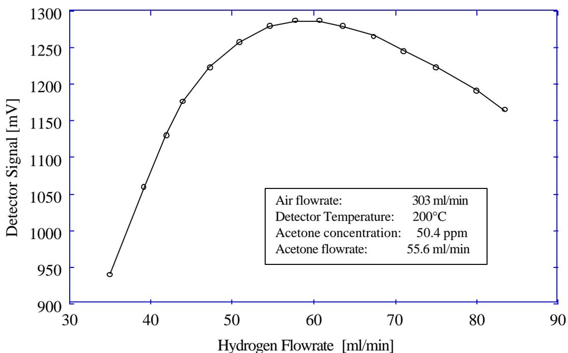
**Figure 7.7** FID Sensitivity Optimization. Adapted from Schaefer [30]
