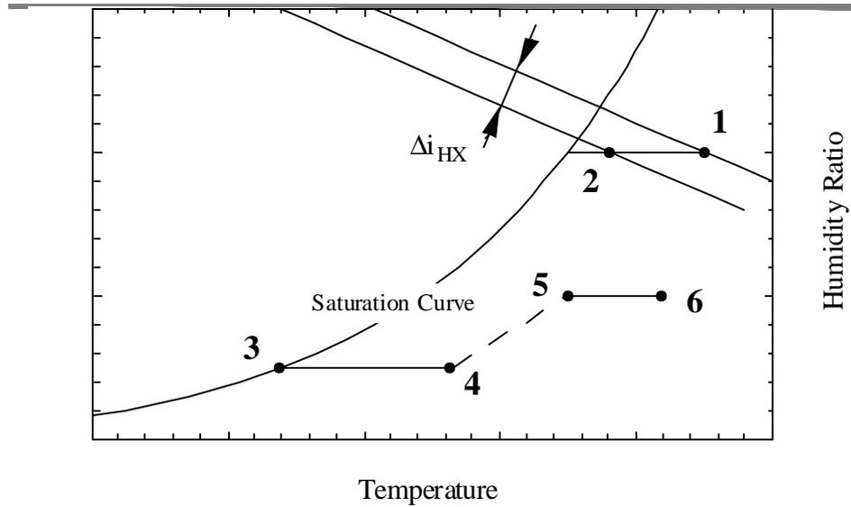
**Figure 1.4:** Air Cooling Using a Sensible Heat Exchanger
