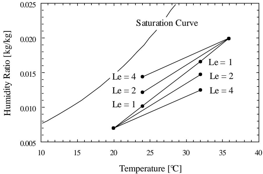
**Figure 1.8:** Enthalpy Exchanger Outlet States for Various Lewis Numbers
