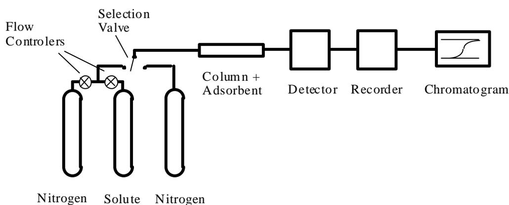
**Figure 7.1** Schematic of Gas Chromatograph System
