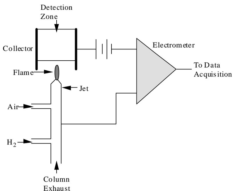
**Figure 7.6** Flame Ionization Detector. Adapted from Buffington and Wilson [7]
