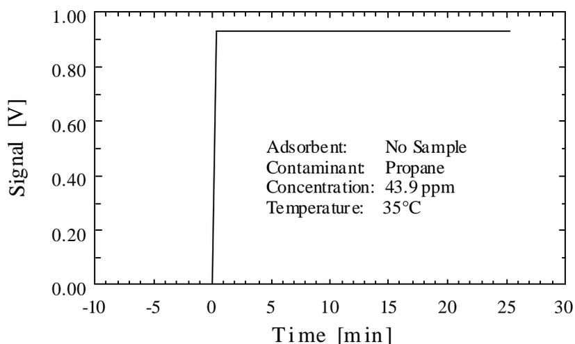
**Figure 7.9** Propane Chromatogram. No Sample
