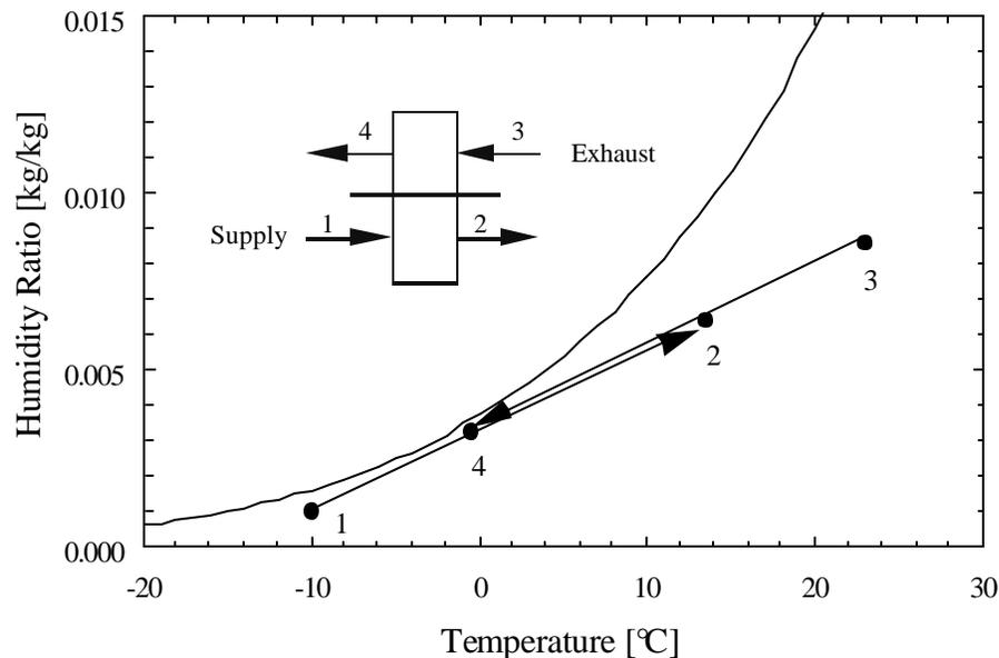
**Figure 6.4:** Enthalpy Exchanger Operation without Excess Water
