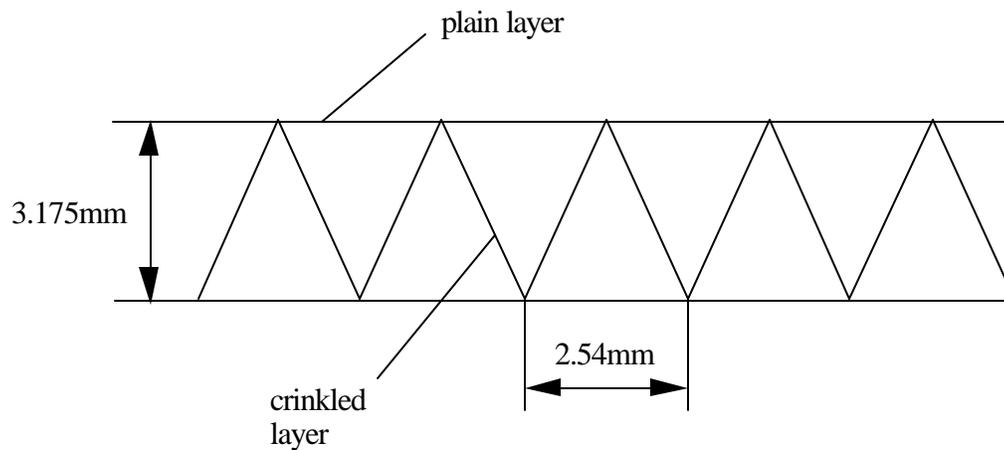
**Figure 5.6:** Cross Sectional Dimensions of the Investigated Matrix
