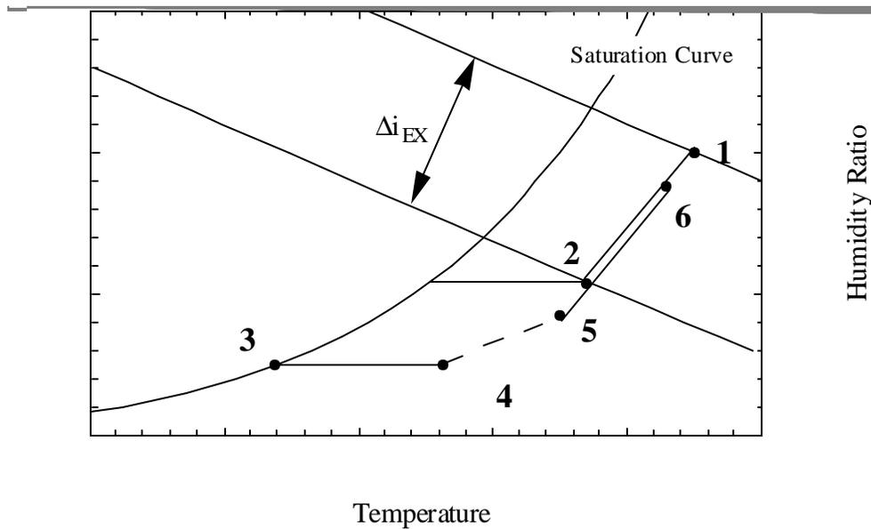
**Figure 1.5:** Air Cooling Using an Enthalpy Exchanger
