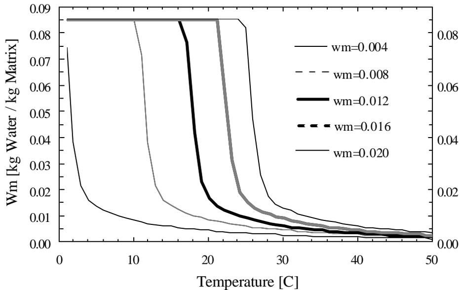
**Figure 5.1:** Water-Based Polymer: Adsorption Capacity vs. Temperature
