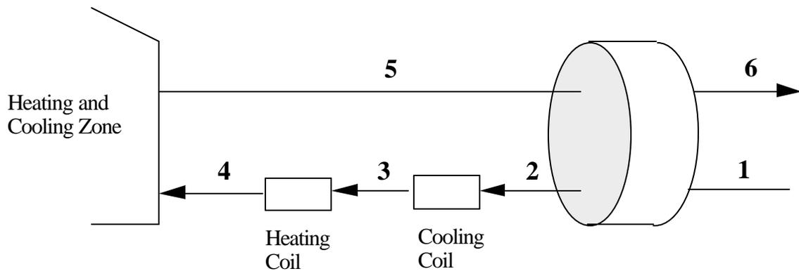
**Figure 1.3:** Air-Conditioning System with Regenerative Recovery Unit
