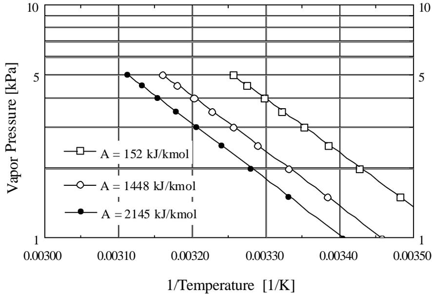
**Figure 5.5:** Van't Hoff Plots for Constant Adsorption Potentials
