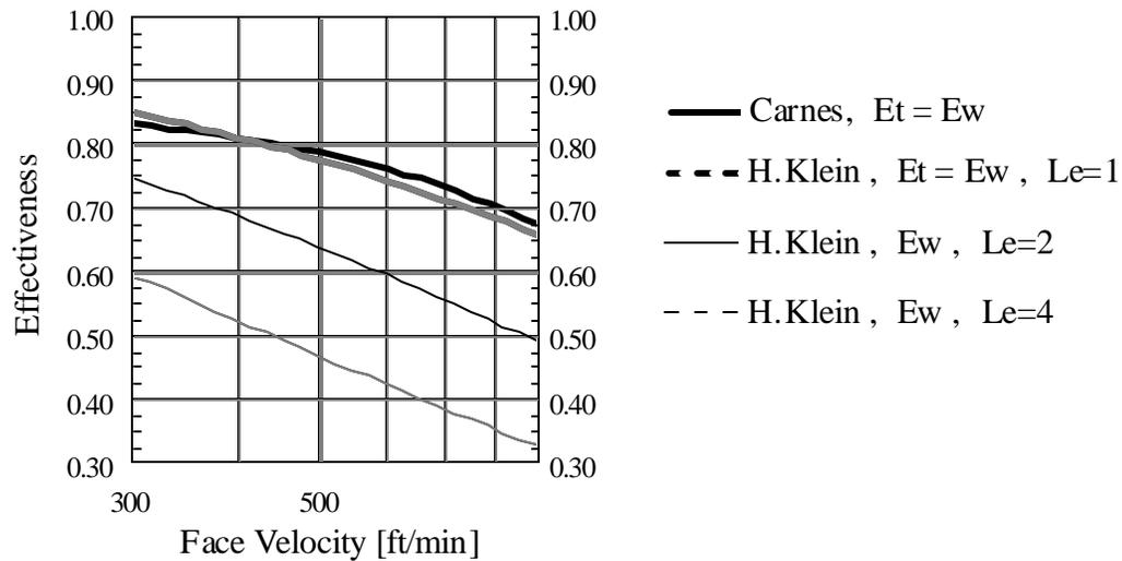
**Figure 5.7:** Heat- and Mass Transfer Effectivenesses of the Water-Based Polymer Coated Matrix
