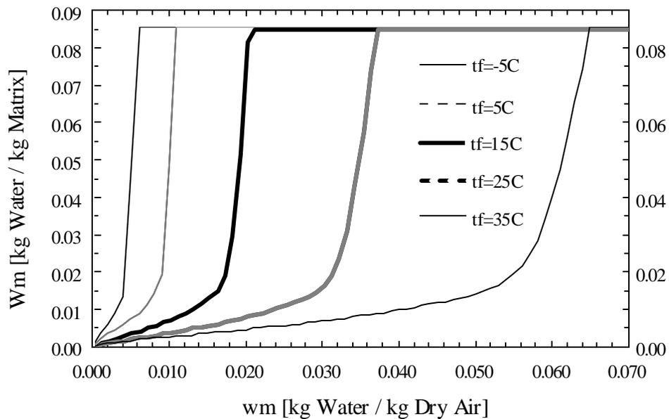
**Figure 5.3:** Water-Based Polymer: Adsorption Capacity vs. Humidity Ratio
