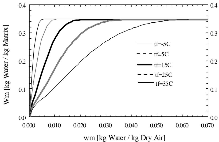
**Figure 5.4:** Silica Gel: Adsorption Capacity vs. Humidity Ratio
