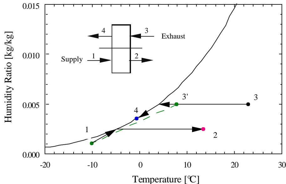
**Figure 6.1:** Heat Exchanger Operation with Exhaust Condensation
