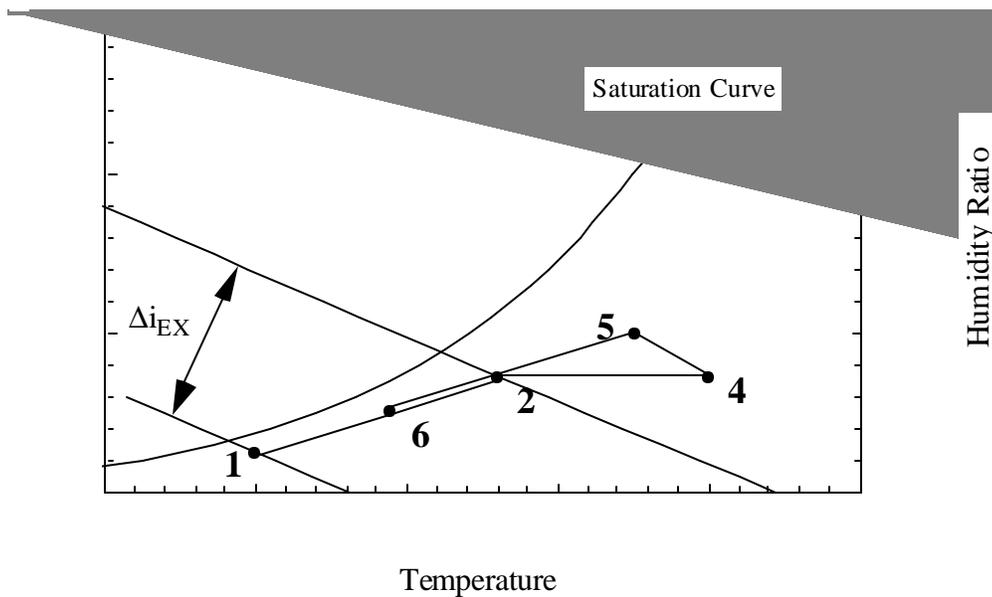
**Figure 1.7:** Air Heating Using an Enthalpy Exchanger
