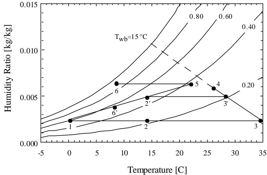
**Figure 5.13:** Psychrometric Chart for a Heating System
