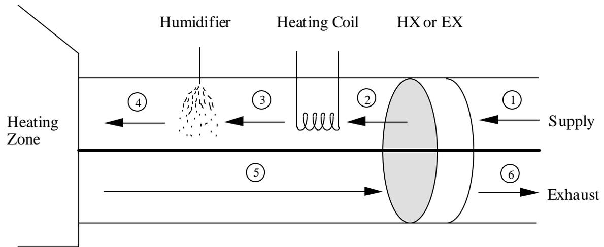
**Figure 5.12:** Schematic of a Heating System
