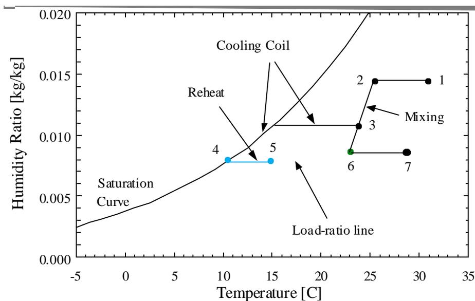
**Figure 5.10:** Single-Zone Cooling with Reheat, Exhaust Air Mixing and Sensible HX.
