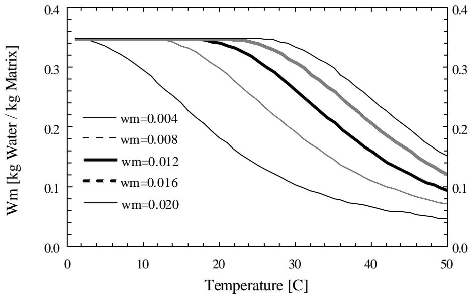
**Figure 5.2:** Silica Gel: Adsorption Capacity vs. Temperature
