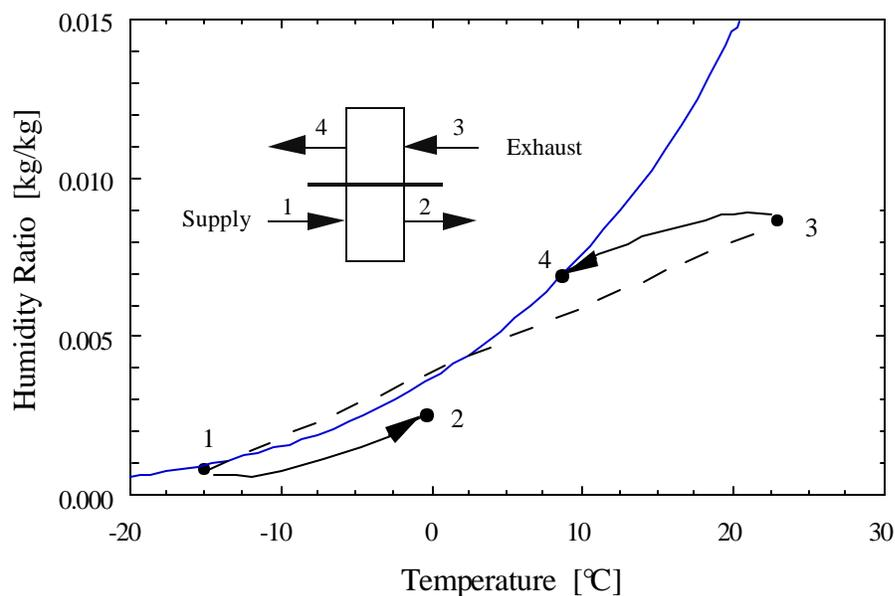
**Figure 6.5:** Enthalpy Exchanger Operation in Excess Water Conditions
