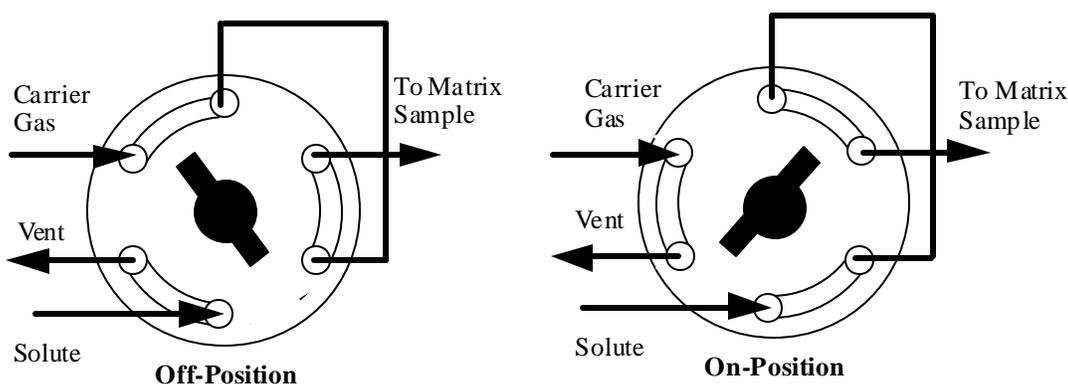
**Figure 7.5** Pneumatic Gas Stream Selection Valve. Adapted from Schaefer [30]
