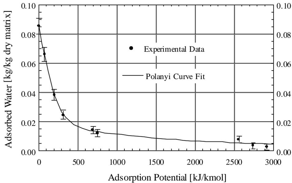
**Figure 3.4:** Experimental Data and Polanyi Curve Fit
