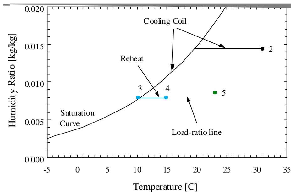
**Figure 5.8:** Single-Zone Cooling with Reheat. No Regenerator.
