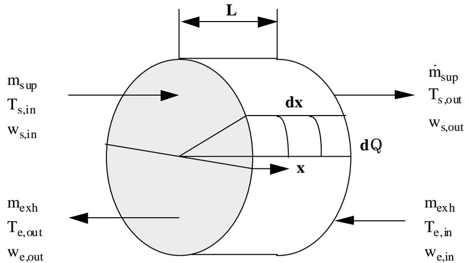
**Figure 1.1:** Matrix of a Rotary Regenerator
