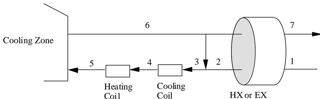
**Figure 5.9:** Air-Conditioning System with Exhaust Air Mixing
