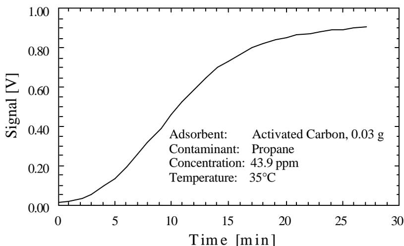
**Figure 7.11** Propane Chromatogram. Activated Carbon
