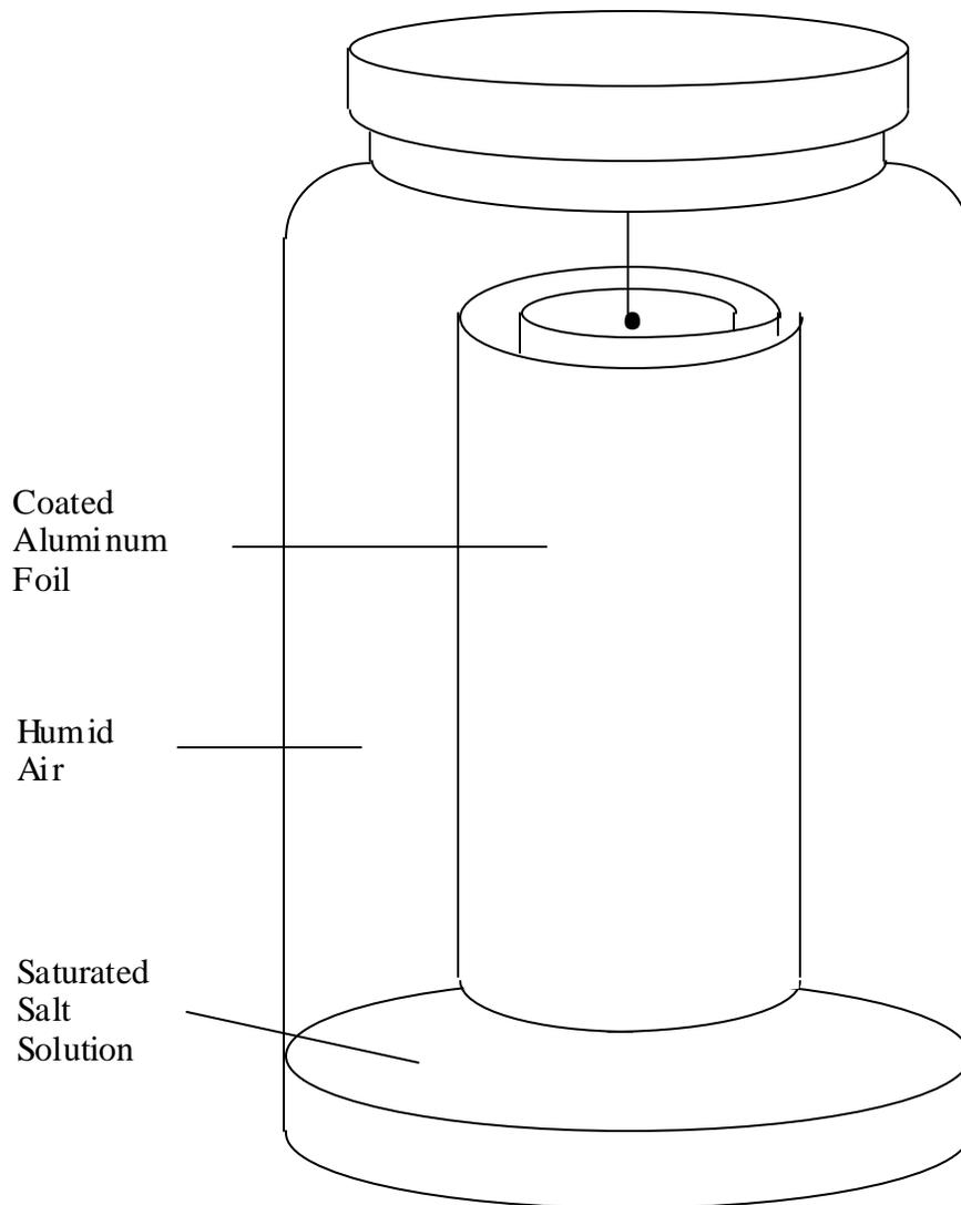
**Figure 3.1:** Experimental Setup
