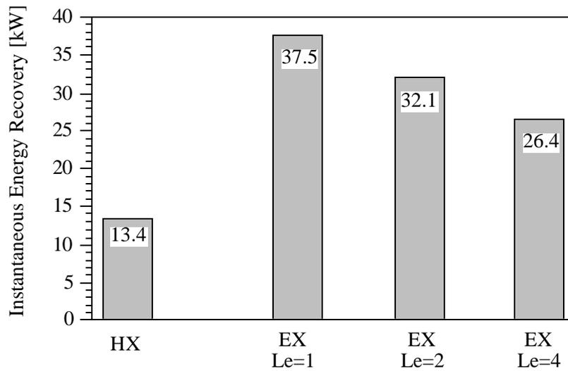
**Figure 5.11:** Total Energy Recovery of HX and EX in a Cooling System
