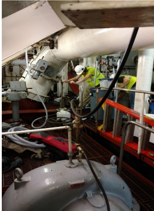
Figure 4. Photo Showing Operation of the Shipboard Sampling System On Board a Test Vessel.
