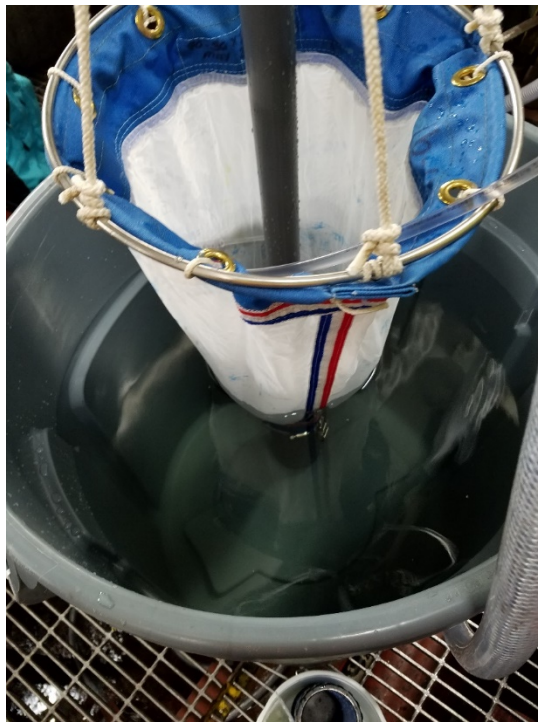
Figure 5. Photo Showing the Shipboard Sampling System's Plankton Net Component On Board a Test Vessel.
