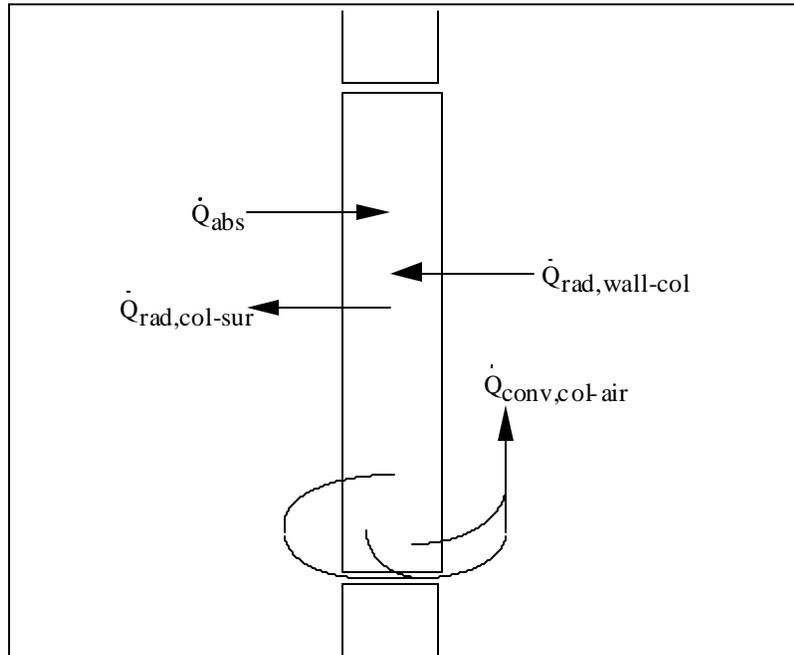
Figure 2.1.3. Energy balance on collector plate. { TC "Figure 2.1.3. Energy balance on collector plate." \l 5 }
