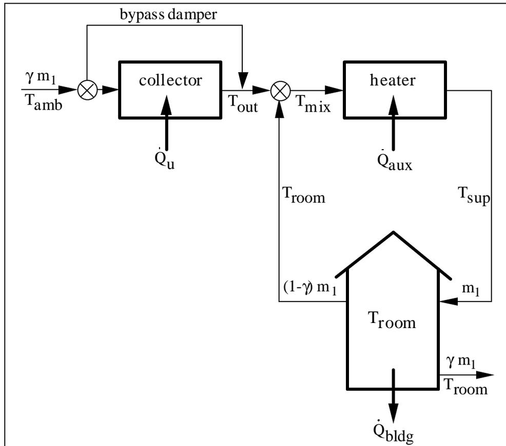
Figure 2.3.1. Basic overview of the UTC system model. { TC "Figure 2.3.1. Basic overview of the UTC system model." \ 5 }
