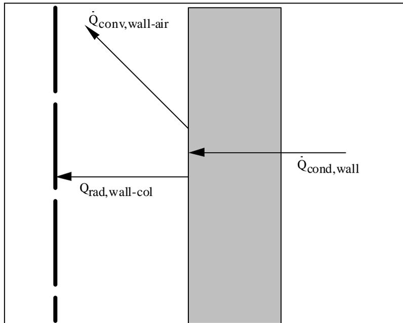
Figure 2.1.2. Energy balance on wall. { TC "Figure 2.1.2. Energy balance on wall." \l 5 }
