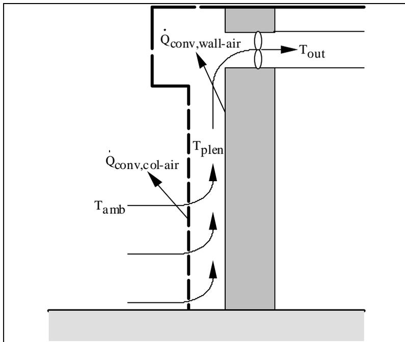
Figure 2.1.1. Energy balance on air. { TC "Figure 2.1.1. Energy balance on air." \l 5 }
