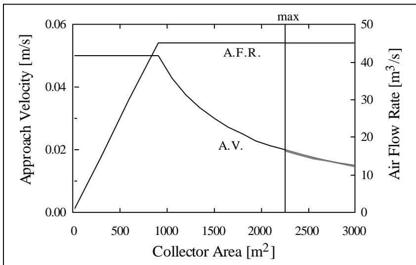
Figure 2.8.1. Approach velocity and air flow rate at  $\gamma_{\min}$ .
