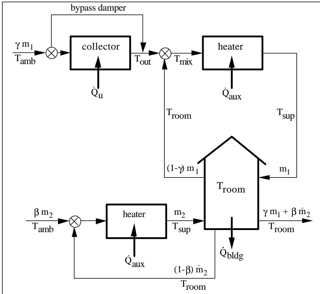
Figure 2.7.1. Complete overview of the UTC system model. { TC "Figure 2.7.1. Complete overview of the UTC system model." | 5 }
