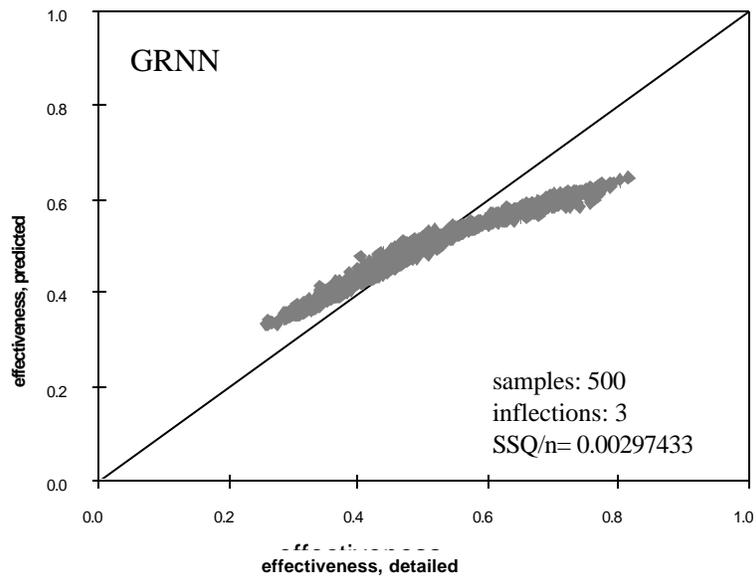
*Fig. 3.3-10 Predicted effectiveness versus effectiveness from detailed model for 999 randomly picked points for 500 unequally spaced training samples, using the approach using no additional knowledge*
