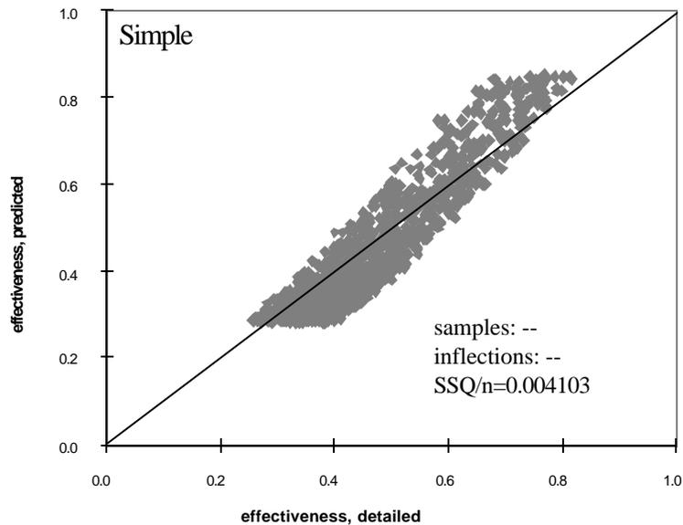
*Fig. 3.3-7 Predicted effectiveness using the simple model versus effectiveness from detailed model for 999 randomly picked points*
