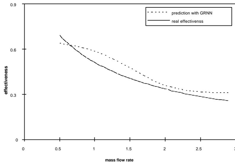
*Fig. 3.3-19 Effectiveness versus mass flow rate using 150 samples unequally spaced, allowing more wiggles, plotted for  $T_{i,water} = 360K$ ,  $T_{air} = 300K$ , velocity = 12.5m/s*
