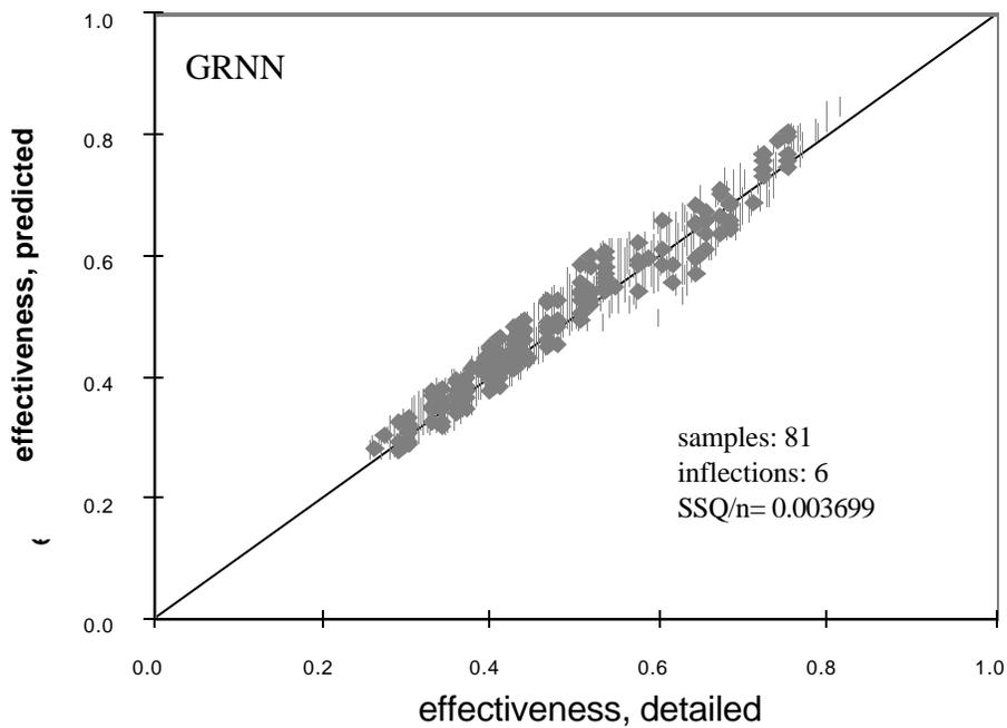
*Fig. 3.3-15 Predicted effectiveness versus effectiveness from detailed model for 999 randomly picked points for 81 equally spaced training samples, using the approach using the approach to correct the simples model, allowing 6 wiggles in the wiggle method*
