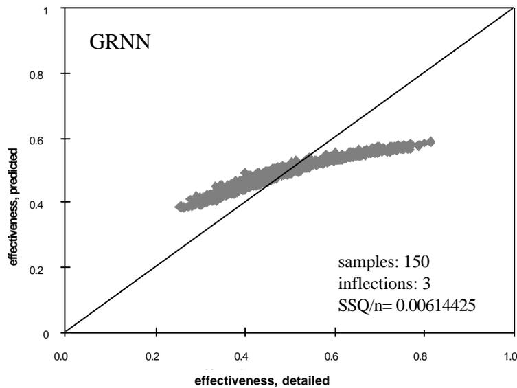
*Fig. 3.3-12 Predicted effectiveness versus effectiveness from detailed model for 999 randomly picked points for 150 unequally spaced training samples, using the approach using no additional knowledge*
