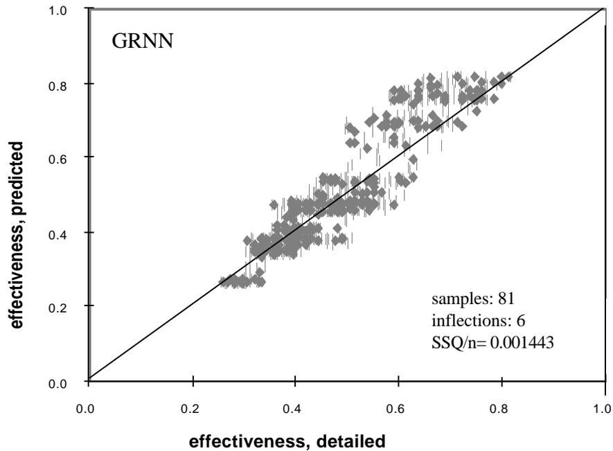
*Fig. 3.3-14 Predicted effectiveness versus effectiveness from detailed model for 999 randomly picked points for 81 equally spaced training samples, using the approach using no additional knowledge, allowing 6 wiggles in the wiggle method*
