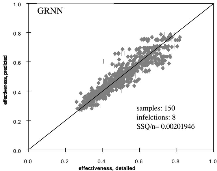
*Fig. 3.3-18 Predicted effectiveness versus effectiveness from detailed model for 999 randomly picked points for 150 unequally spaced training samples, allowing more inflections, using the approach using no additional knowledge*
