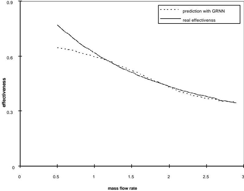
Fig. 3.3-20 Effectiveness versus mass flow rate using 150 samples unequally spaced, allowing more wiggles plotted for  $T_{in,water} = 360K$ ,  $T_{air} = 300K$ , velocity = 25m/s
