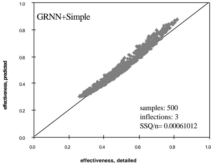
*Fig. 3.3-11 Predicted effectiveness versus effectiveness from detailed model for 999 randomly picked points for 500 unequally spaced training samples, using the approach to correct simple model*
