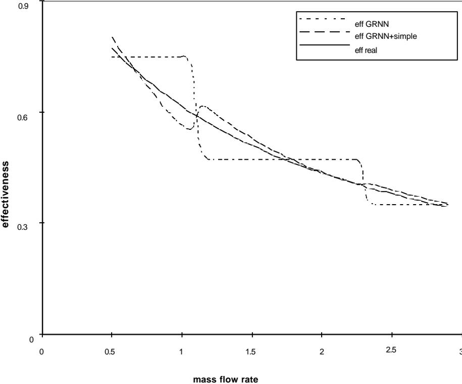
Fig. 3.3-16 Effectiveness versus mass flow rate using 81 samples equally spaced, plotted for  $T_{in,water}=360K$ ,  $T_{air}=300K$ , velocity=12.5m/s, allowing 6 inflection points in the wiggle method.
