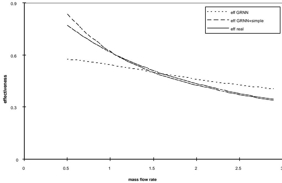
Fig. 3.3-5 Effectiveness versus mass flow rate using 150 samples unequally spaced, plotted for  $T_{in,water}=360K$ ,  $T_{air}=300K$ , velocity=12.5m/s
