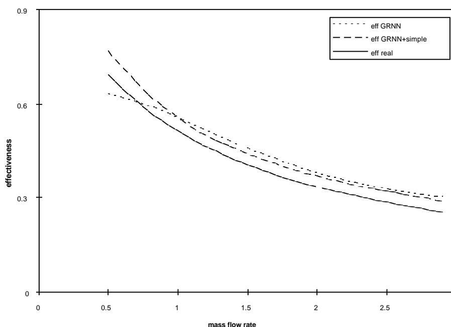
*Fig. 3.3-1 Effectiveness versus mass flow rate using 81 samples, equally spaced, plotted for  $T_{in,water}=360K$ ,  $T_{air}=300K$ , velocity=12.5m/s*
