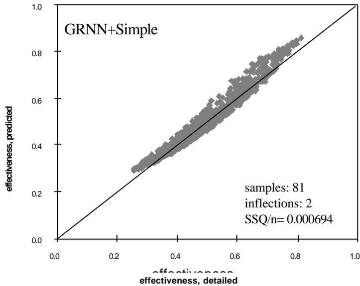
*Fig. 3.3-9 Predicted effectiveness versus effectiveness from detailed model for 999 randomly picked points for 81 equally spaced training samples, using the approach to correct simple model*
