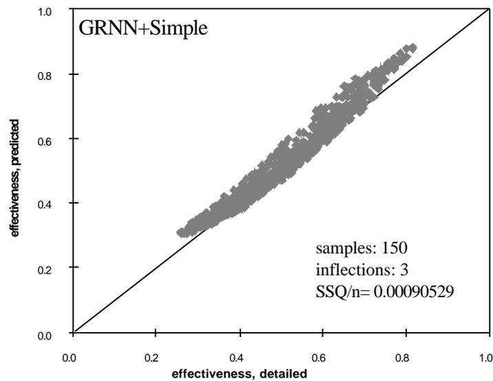
*Fig. 3.3-13 Predicted effectiveness versus effectiveness from detailed model for 999 randomly picked points for 150 unequally spaced training samples, using the approach to correct simple model*
