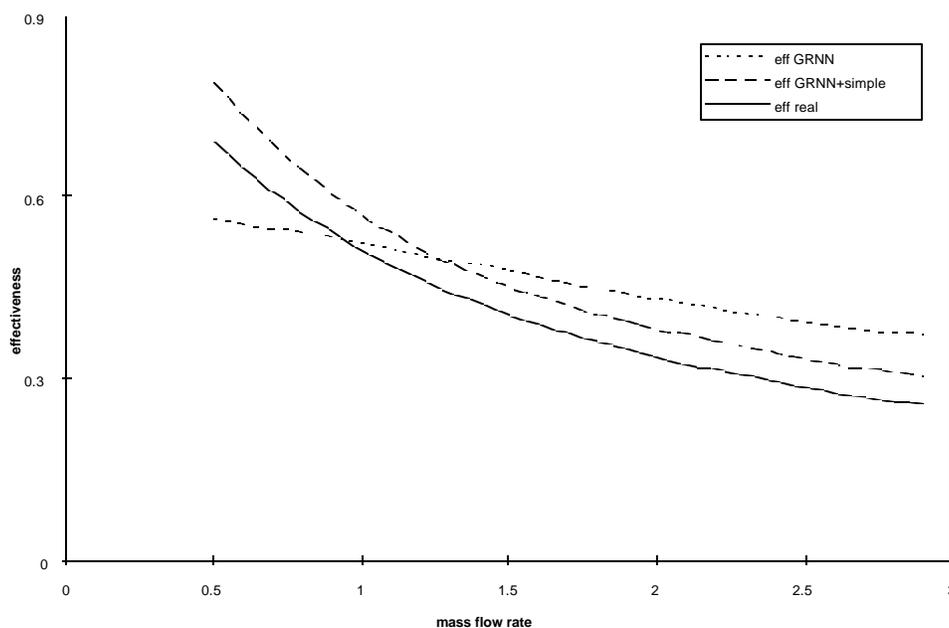
*Fig. 3.3-4 Effectiveness versus mass flow rate using 500 samples unequally spaced, plotted for  $T_{in,water}=360K$ ,  $T_{air}=300K$ , velocity=25m/s*
