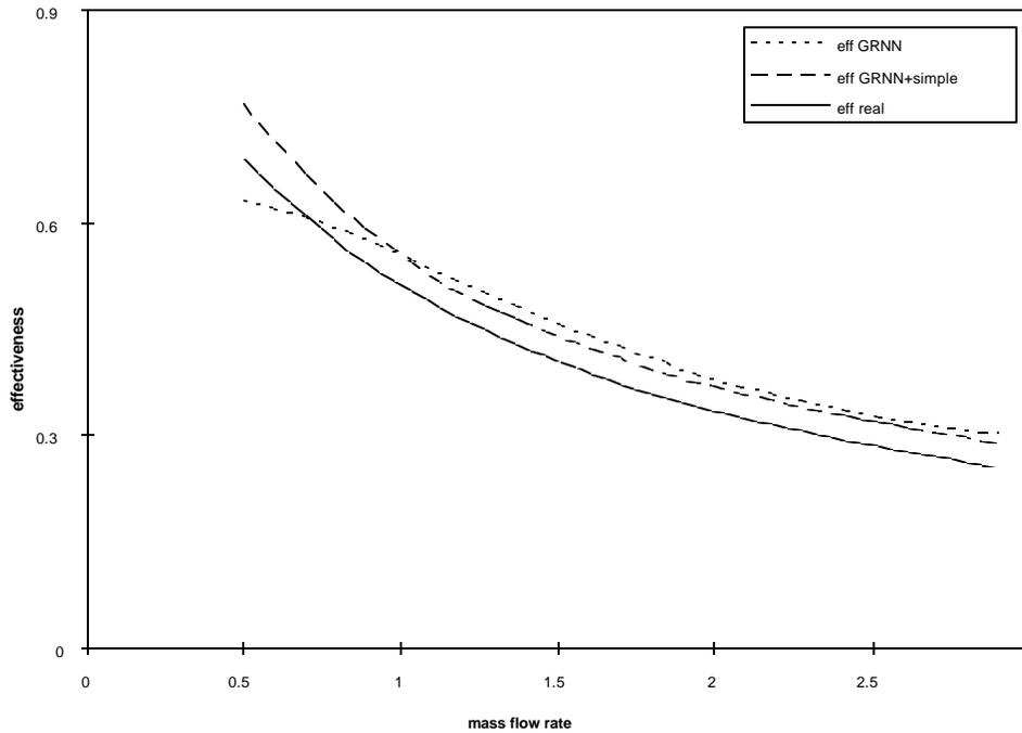
*Fig. 3.3-6 Effectiveness versus mass flow rate using 150 samples unequally spaced, plotted for  $T_{in,water}=360K$ ,  $T_{air}=300K$ , velocity=25m/s*
