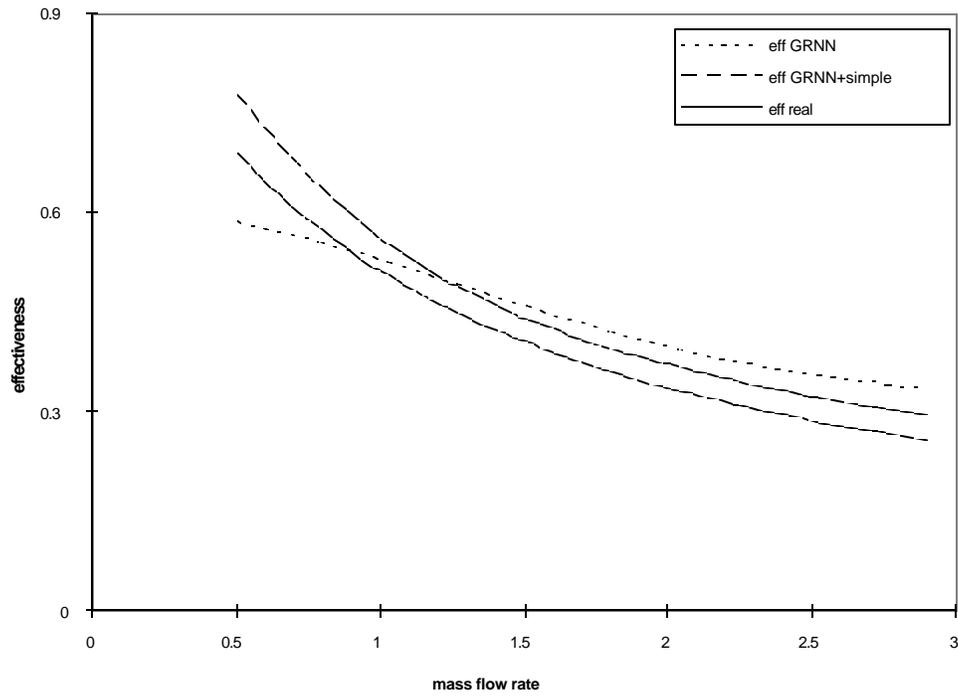
Fig. 3.3-3 Effectiveness versus mass flow rate using 500 samples unequally spaced, plotted for  $T_{in,water}=360K$ ,  $T_{air}=300K$ , velocity=12.5m/s
