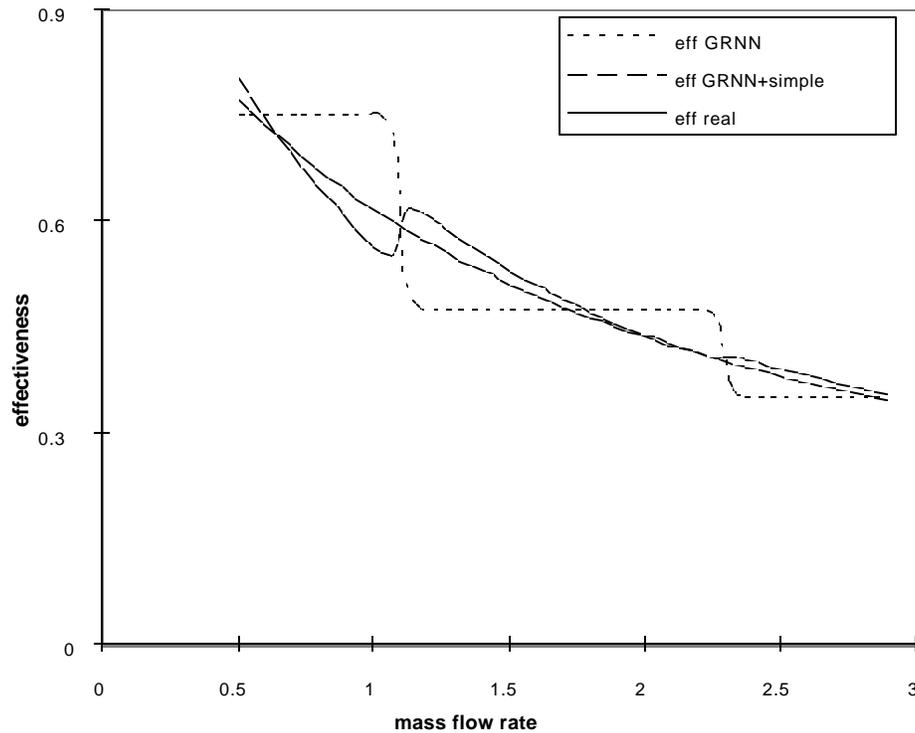
*Fig. 3.3-17 Effectiveness versus mass flow rate using 81 samples equally spaced, plotted for  $T_{in,water}=360K$ ,  $T_{air}=300K$ , velocity=25m/s, allowing 6 inflection points in the wiggle method*
