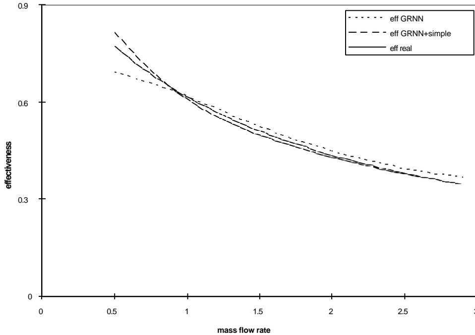
Fig. 3.3-2 Effectiveness versus mass flow rate using 81 samples equally spaced, plotted for  $T_{in,water}=360K$ ,  $T_{air}=300K$ , velocity=25m/s
