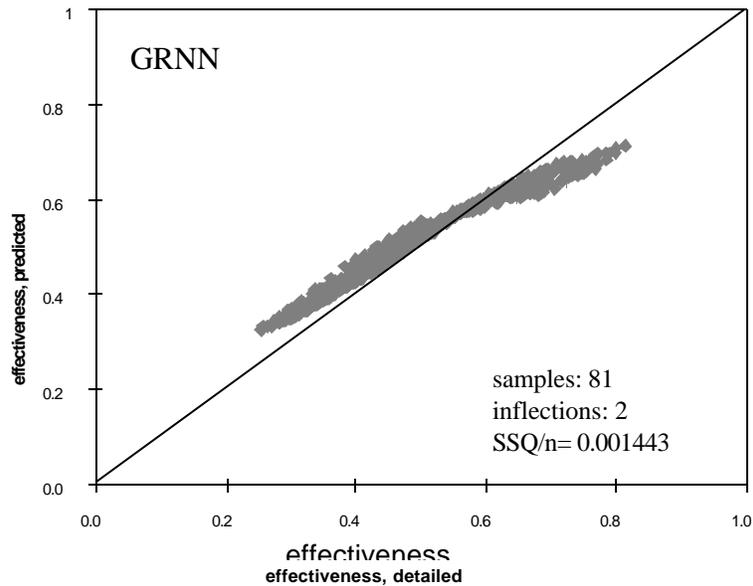
*Fig. 3.3-8 Predicted effectiveness versus effectiveness from detailed model for 999 randomly picked points for 81 equally spaced training samples, using the approach using no additional knowledge*
