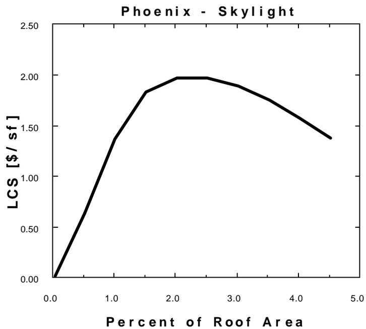
Figure 5.4 Life-cycle costs of skylights - Phoenix, Arizona;{ TC "Figure 5.4 Life-cycle costs of skylights - Phoenix, Arizona;" \ 5 }
