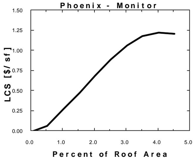
Figure 5.10 Life-cycle costs of monitors - Phoenix, Arizona;{ TC "Figure 5.10 Life-cycle costs of monitors - Phoenix, Arizona;" \ 5 }
