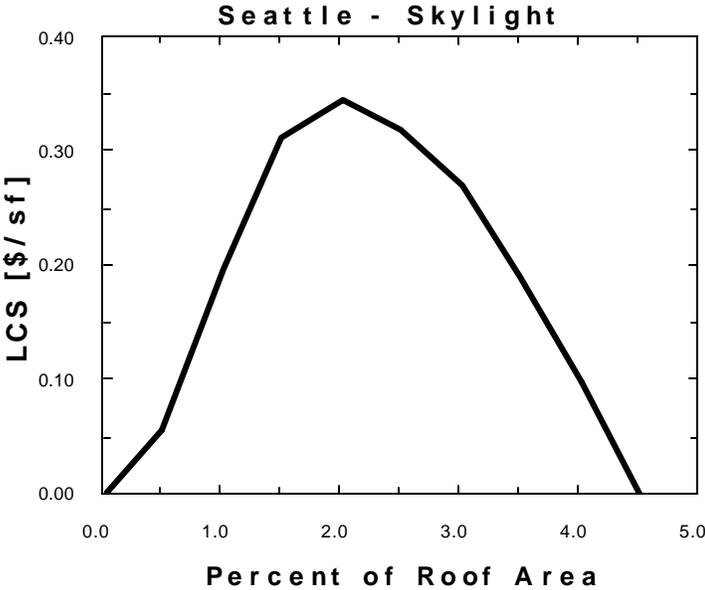
Figure 5.5 Life-cycle costs of skylights - Seattle, Washington;{ TC "Figure 5.5 Life-cycle costs of skylights - Seattle, Washington;" \ 5 }
