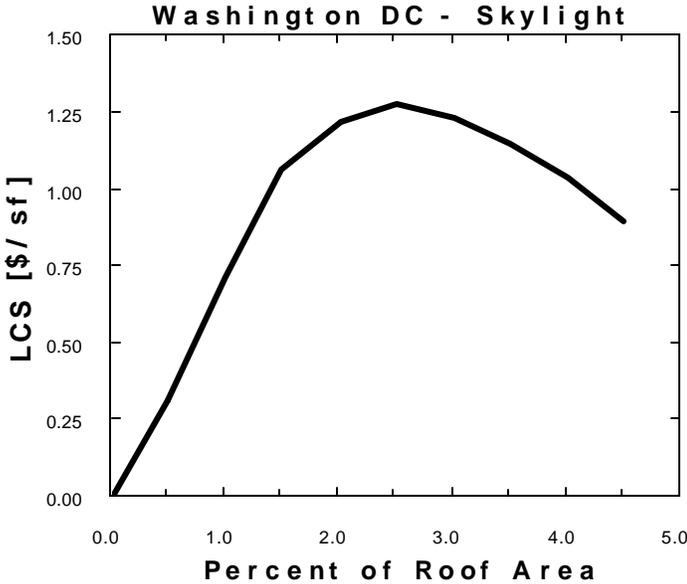
Figure 5.6 Life-cycle costs of skylights - Washington, DC;{ TC "Figure 5.6 Life-cycle costs of skylights - Washington, DC;" \ 5 }
