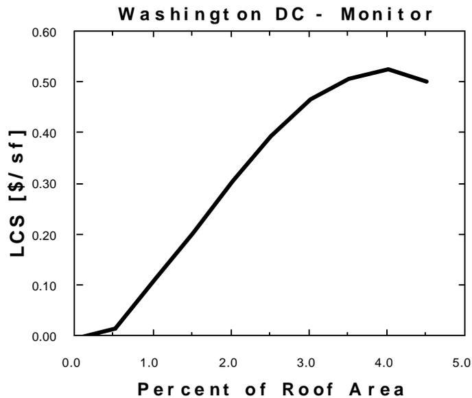
Figure 5.11 Life-cycle costs of monitors - Washington, DC;{ TC "Figure 5.11 Life-cycle costs of monitors - Washington, DC;" \l 5 }
