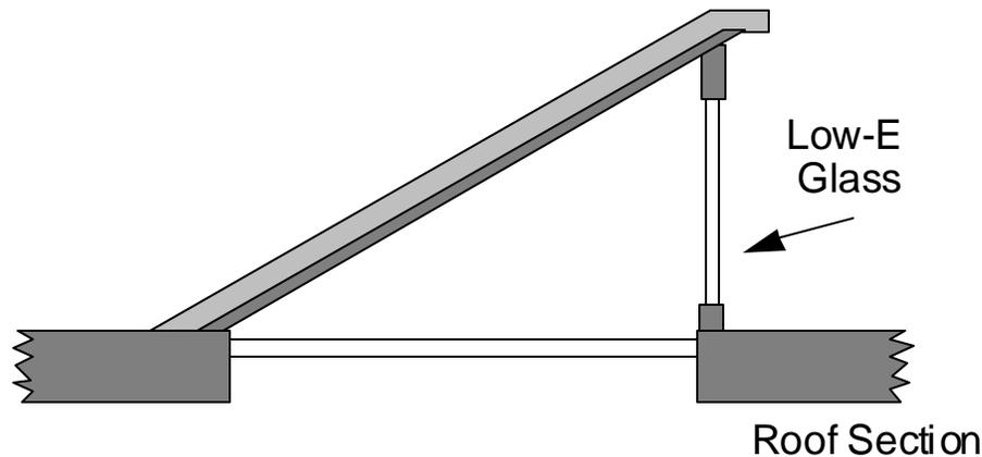
Figure 5.1 Sawtooth roof monitor. { TC "Figure 5.1 Sawtooth roof monitor." \ 5 }
