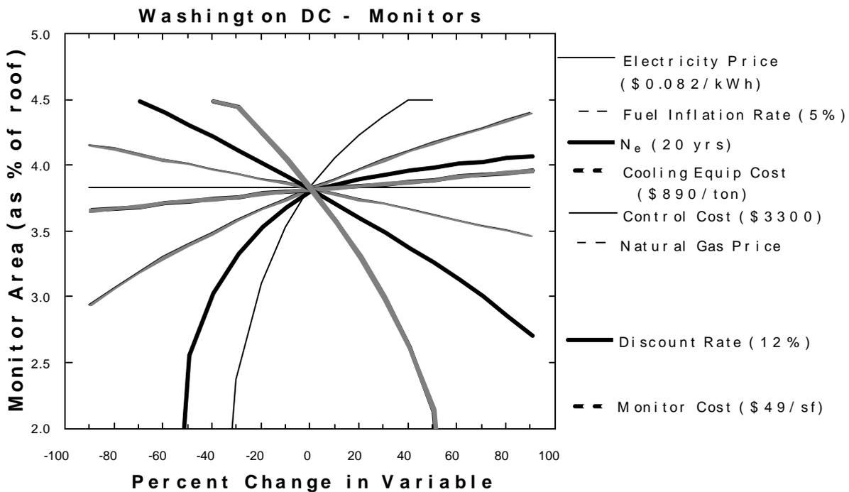
Figure 5.13 Sensitivity analysis of monitors - Washington, DC{ TC "Figure 5.13 Sensitivity analysis of monitors - Washington, DC" \15 }
