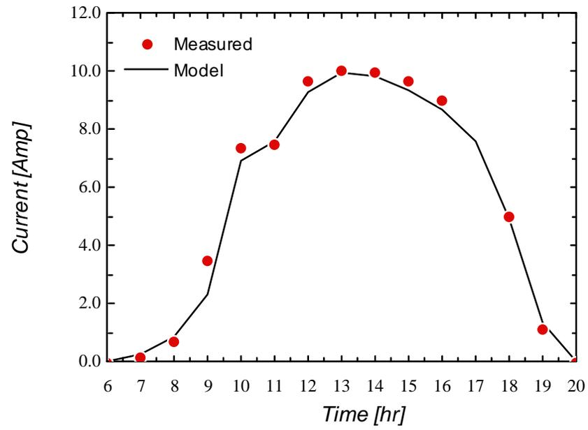
**Figure 3.4.4** Current of FSEC PV pumping system as a function of time. Data measured on August 23rd, 1987. Data reported by FSEC.
