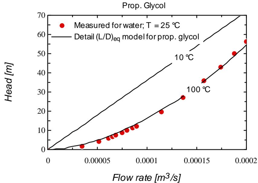
**Figure 3.1.8** Simulated  $H-Q$  curves of an SDHW system at two collector fluid temperatures compared to the measure  $H-Q$  data for water. The collector fluid is propylene glycol mixture.
