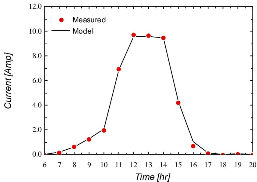
**Figure 3.4.12** Current of FSEC PV pumping system as a function of time. Data measured on September 5th, 1987. Data reported by FSEC.
