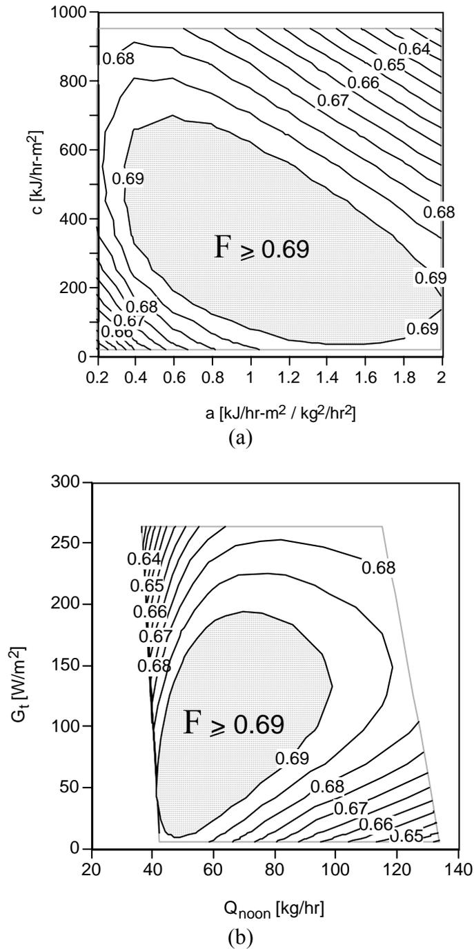
**Figure 5.1.7** (a) Contour plot of the annual solar fraction of the base system as a function of the parameters  $a$  and  $c$ . (b) Contour plot of the annual solar fraction of the base system as a function of the parameters  $Q_{noon}$  and  $G_t$ . The value of the parameter  $b$  for both is set to zero.
