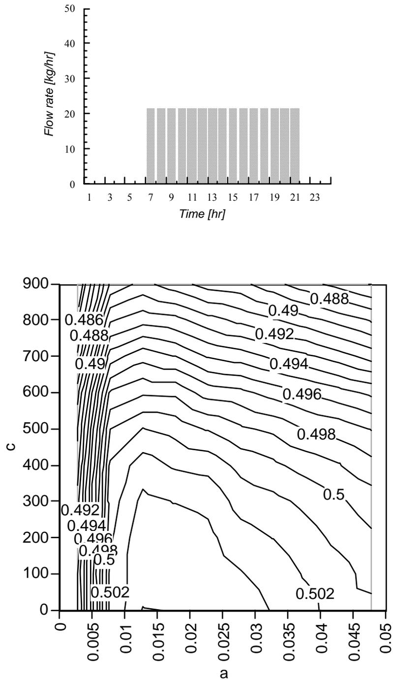
**Figure 6.1.11** The standard load profile and the resulting contour plot of the annual solar fraction of the base system as a function of the parameters  $a$  and  $c$ .
