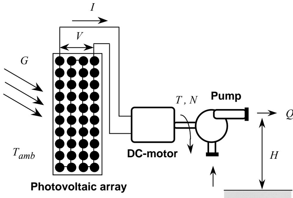
**Figure 1.2.1** Schematic drawing of a direct-coupled PV pumping system.
