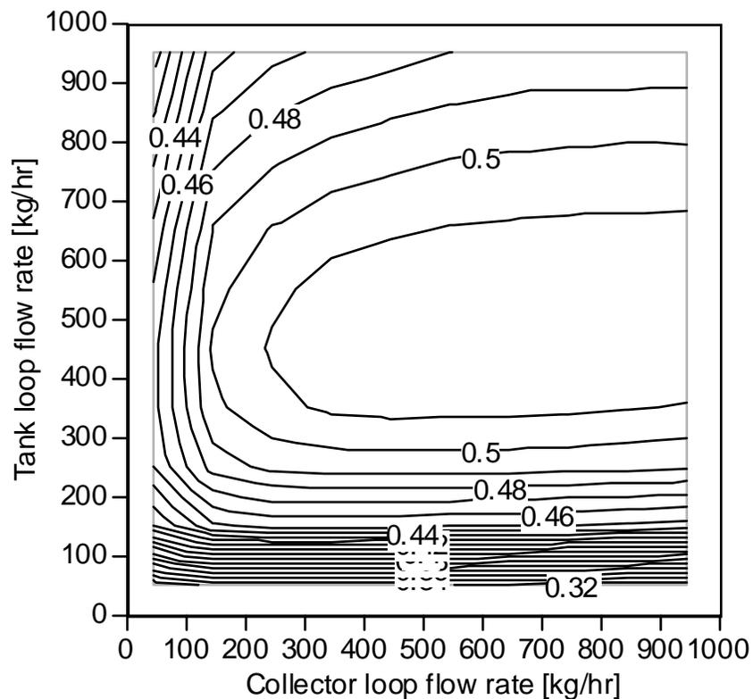
**Figure 6.1.2** Contour plot of the annual solar fraction as a function of the constant collector loop flow rate and the constant tank loop flow rate.
