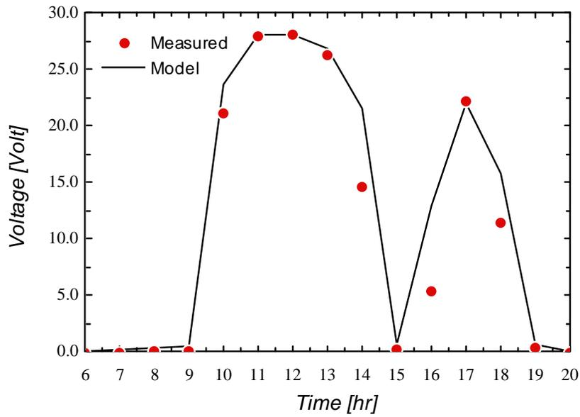
**Figure 3.4.15** Voltage of FSEC PV pumping system as a function of time. Data measured on September 7th, 1987. Data reported by FSEC.
