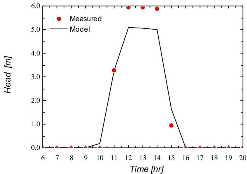
**Figure 3.4.10** Head of FSEC PV pumping system as a function of time. Data measured on September 5th, 1987. Data reported by FSEC.
