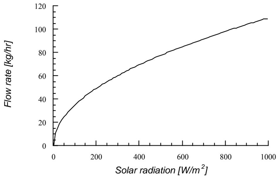
**Figure 6.2.2** The optimum flow rate profile found in phase one.
