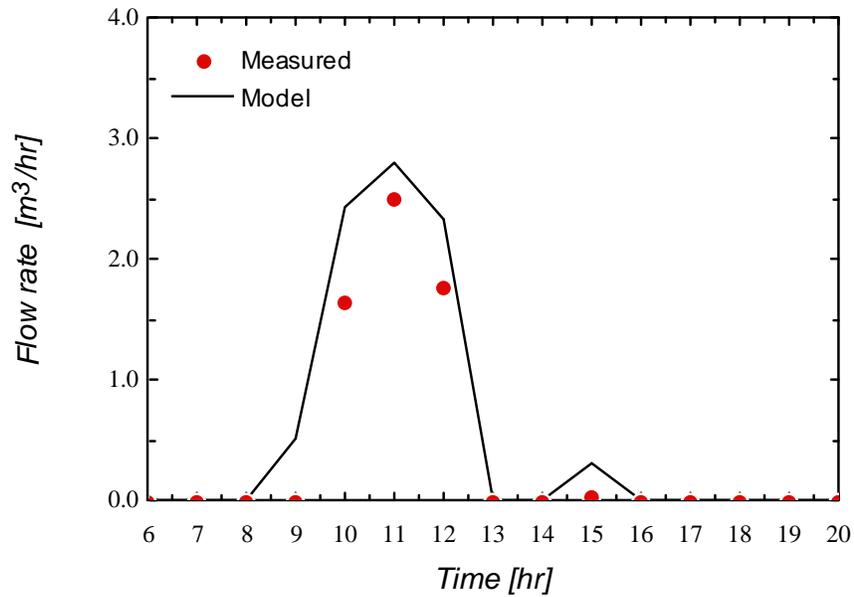
**Figure 3.4.5** Flow rate of FSEC PV pumping system as a function of time. Data measured on September 3rd, 1987. Data reported by FSEC.
