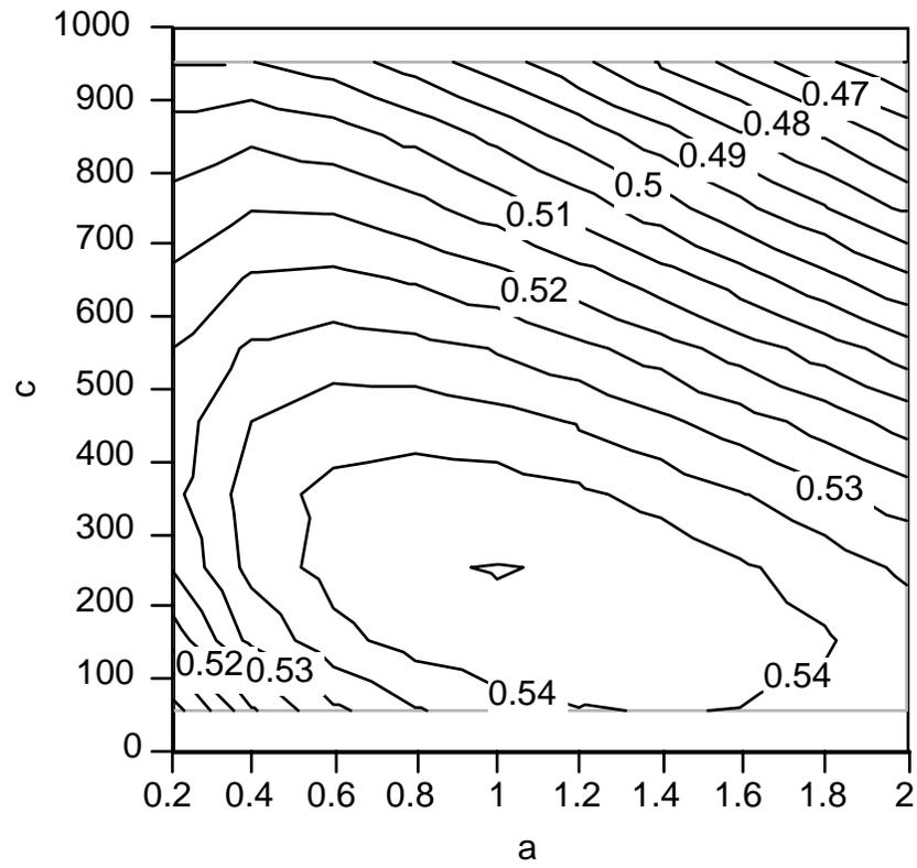
**Figure 5.1.21** Contour plot of the annual solar fraction of the base system if located in Seattle, WA.
