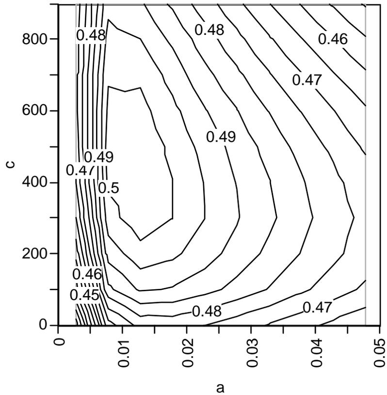
**Figure 6.1.9** Contour plot of the annual solar fraction of the modified system as a function of  $a$  and  $c$ . The system's collector-side and tank-side fluid is driven by PV pumping system.
