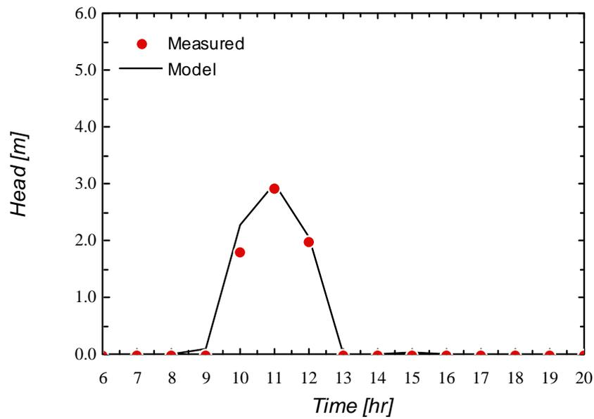
**Figure 3.4.6** Head of FSEC PV pumping system as a function of time. Data measured on September 3rd, 1987. Data reported by FSEC.
