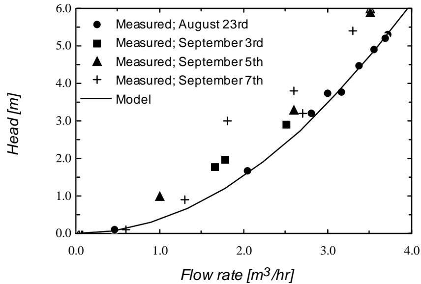
**Figure 3.4.17** FSEC system head for the four days as a function of the flow rate of FSEC system. Data reported by FSEC.
