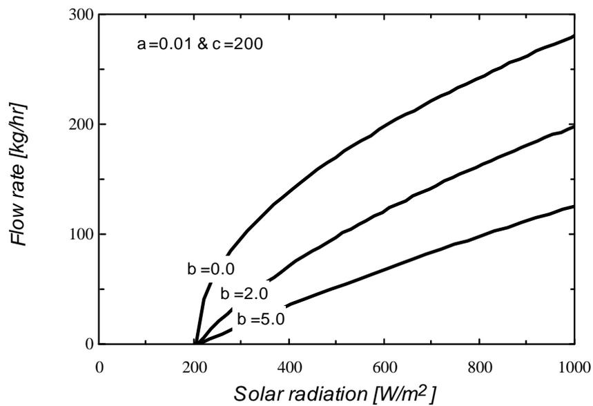
**Figure 4.3.5** The effect of the parameter  $b$  on the general flow rate profile of PV pumping systems.
