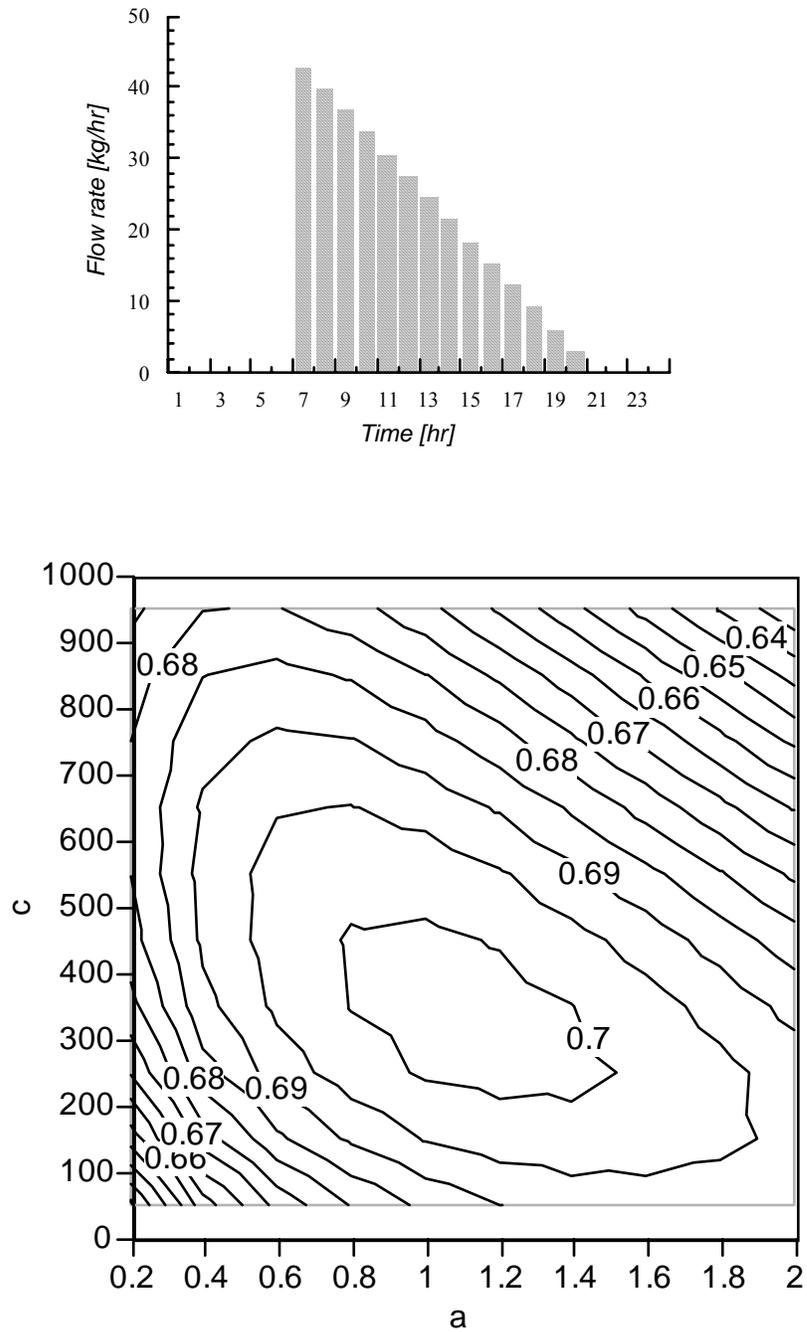
**Figure 5.1.10** Contour plot of the annual solar fraction of the base system as a function of the parameters  $a$  and  $c$ . The load profile is defined as a triangular
