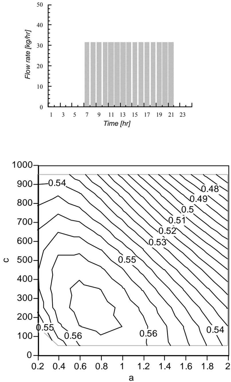
**Figure 5.1.13** Contour plot of the annual solar fraction of the base system as a function of the parameters  $a$  and  $c$ . The load profile is defined as a square function with a daily integral value of 440 kg of water.
