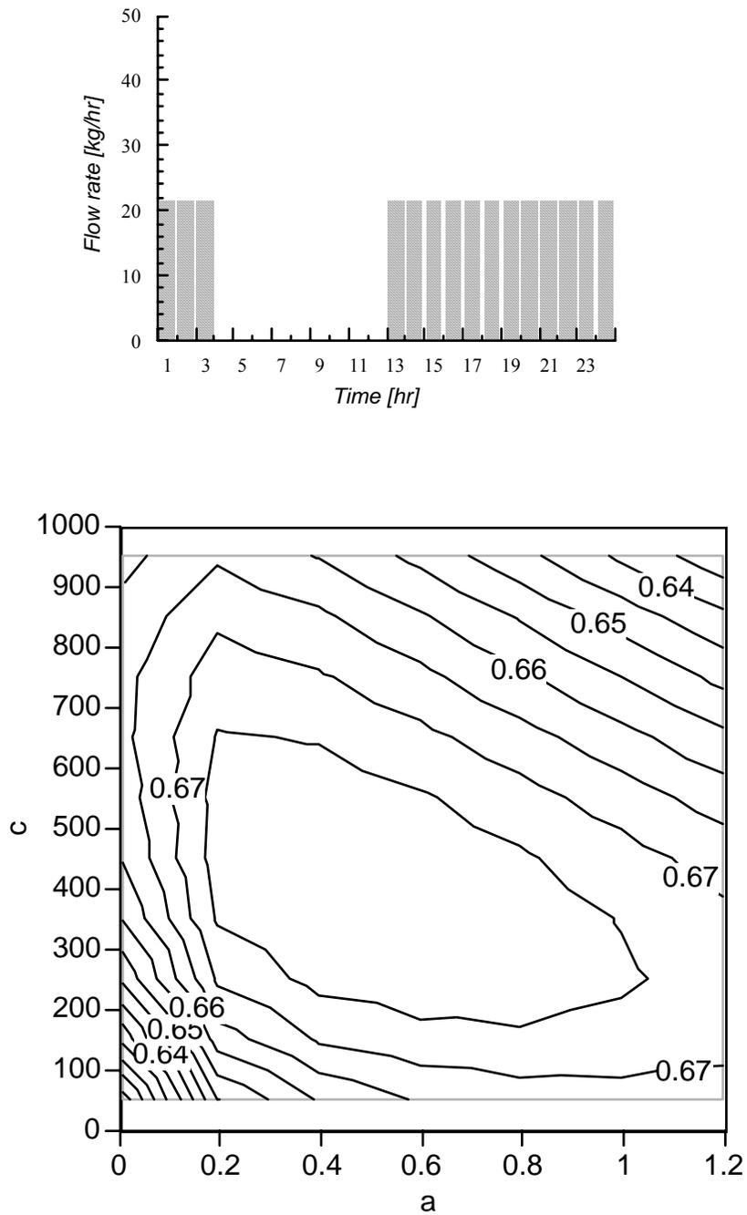
**Figure 5.1.17** Contour plot of the annual solar fraction of the base system as a function of the parameters  $a$  and  $c$ . The load profile has a time-lag of 6 hours from the standard system (Run # 4).
