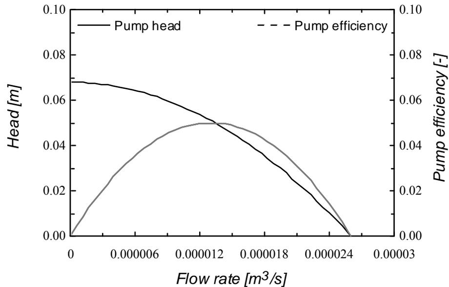
**Figure 5.2.2** The  $H-Q$  and the  $\eta-Q$  of the centrifugal pump used in phase two.
