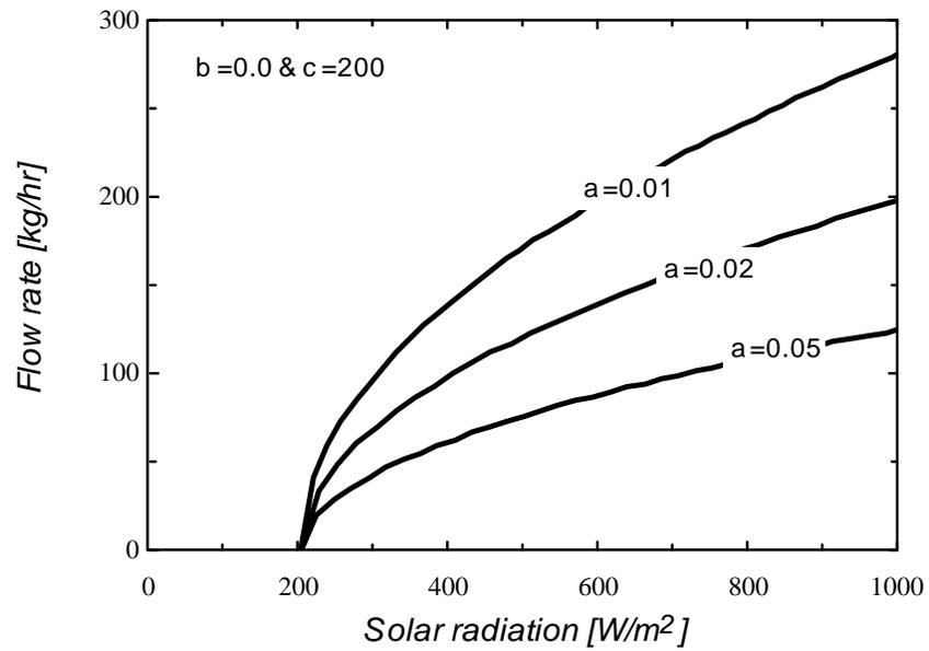
**Figure 4.3.4** The effect of the parameter  $a$  on the general flow rate profile of PV pumping systems.
