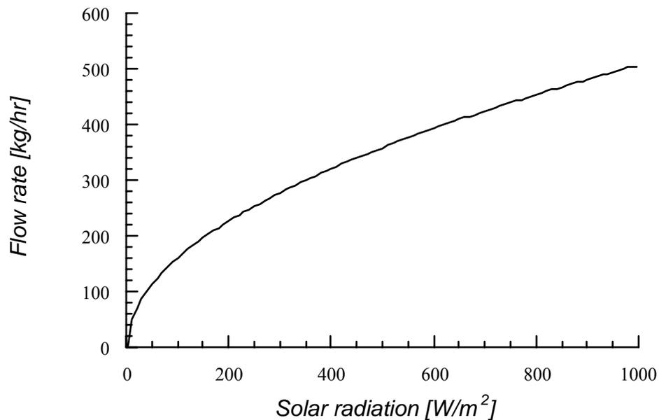
**Figure 6.1.3** The optimum flow rate profile of the base system.
