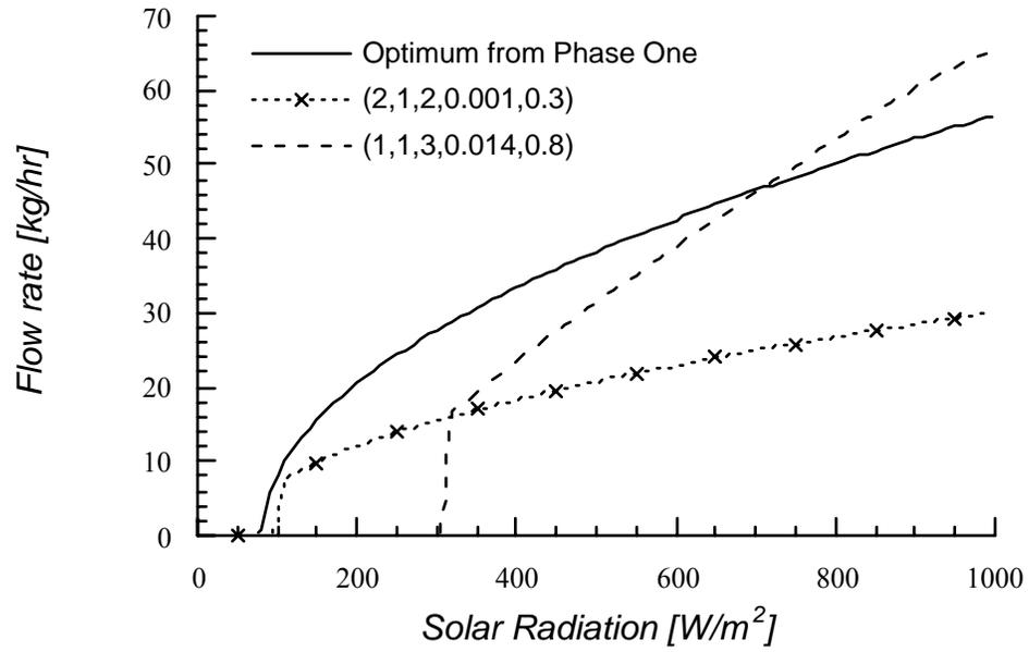
**Figure 5.2.9** The flow rate profile of two off-optimum PV pumping system compared to the optimum flow rate profile found in phase one.
