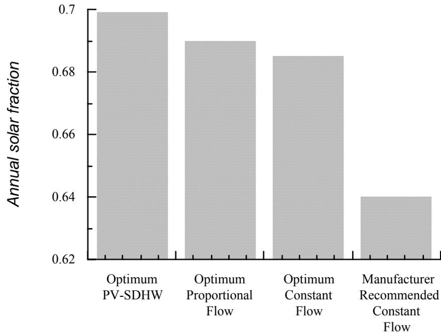
**Figure 5.2.12** The annual solar fraction of the optimum direct PV-SDHW system compared to three SDHW systems operating under different control strategies.
