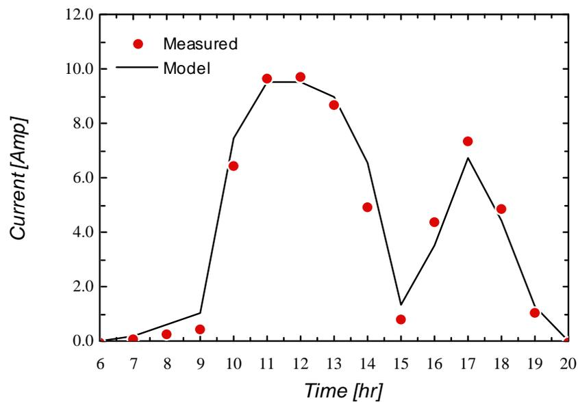
**Figure 3.4.16** Current of FSEC PV pumping system as a function of time. Data measured on September 7th, 1987. Data reported by FSEC.
