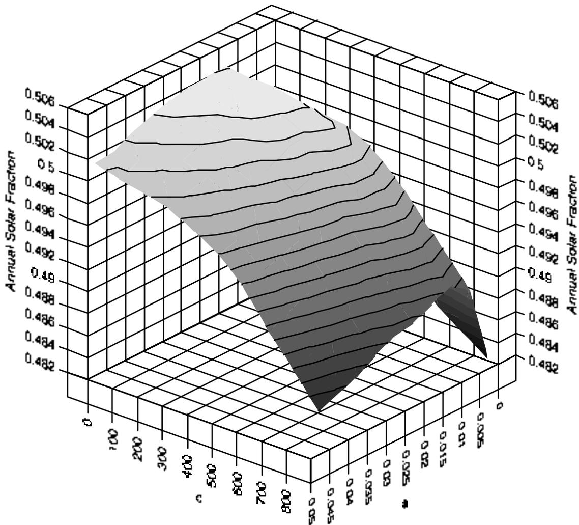
**Figure 6.1.4** Graph of the annual solar fraction as a function of  $a$  and  $c$ , for  $b$  equal zero.
