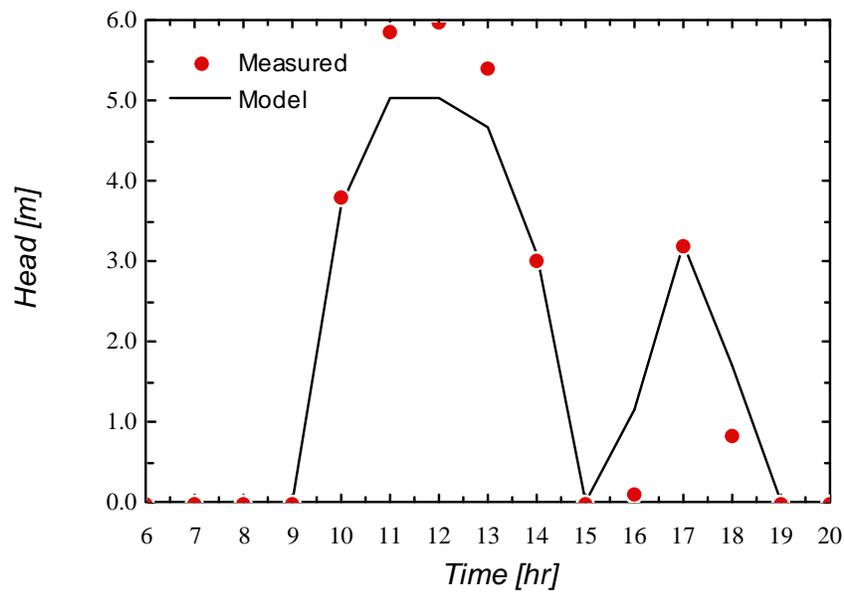
**Figure 3.4.14** Head of FSEC PV pumping system as a function of time. Data measured on September 7th, 1987. Data reported by FSEC.
