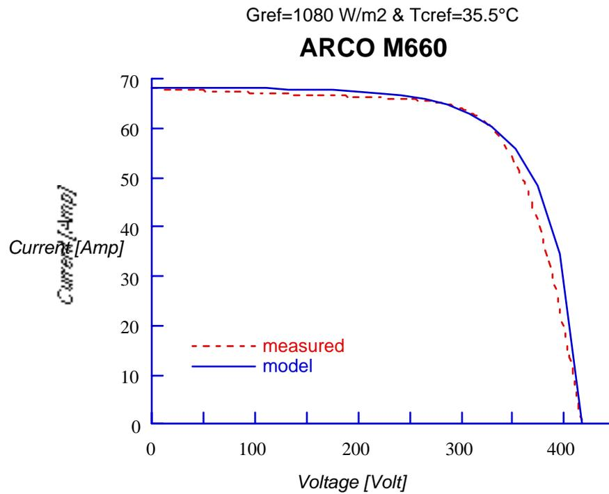
**Figure 3.1.1** Measured and calculated  $I$ - $V$  curve of a PV module at a reference condition of 1080 W/m<sup>2</sup> and 35.5 °C.
