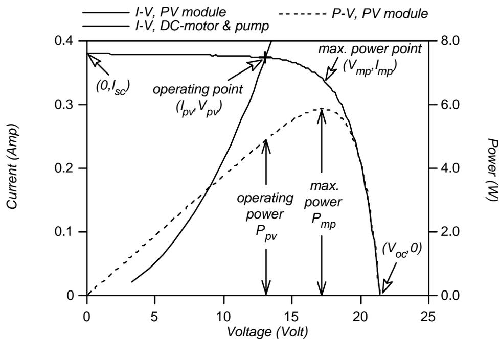
**Figure 1.2.2** The  $I$ - $V$  and  $P$ - $V$  curves of a PV module and the  $I$ - $V$  curve of a load comprising of a separately excited DC-motor coupled to a centrifugal pump along with the PV system operating point if the aforementioned components are directly coupled.
