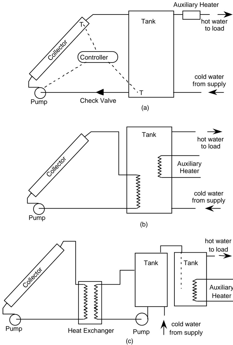
**1.2.5** Schematic drawings of common configurations of active SDHW systems. Adapted from Duffie and Beckman (1991).
