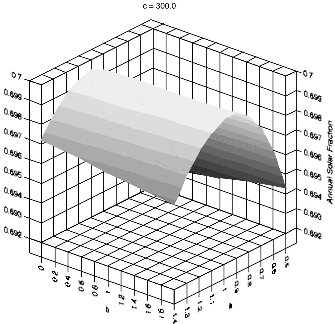
**Figure 5.1.5** Graph of the annual solar fraction of the base system as a function of the parameters  $a$  and  $b$ . The value of the parameter  $c$  is set to 300.
