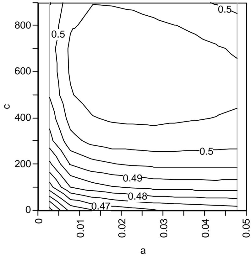
**Figure 6.1.7** Contour plot of the annual solar fraction of the modified system as a function of  $a$  and  $c$ . The system allows the tank-side pump to be ON only if the collector-side fluid is circulating.
