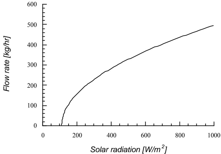
**Figure 6.1.10** The optimum collector-side and tank-side flow rate profile of the control-less system. The system's collector-side and tank-side fluid is driven by PV pumping system.
