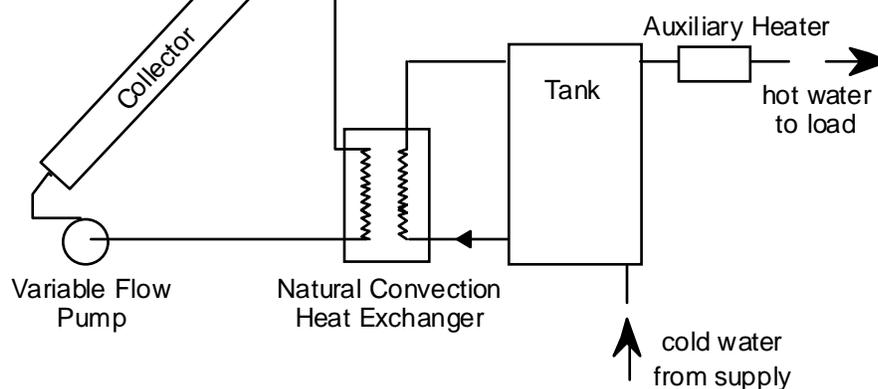
**Figure 6.2.1** Schematic drawing of the base system used in phase one.
