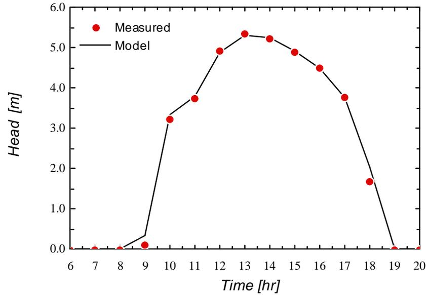
**Figure 3.4.2** Head of FSEC PV pumping system as a function of time. Data measured on August 23rd, 1987. Data reported by FSEC.
