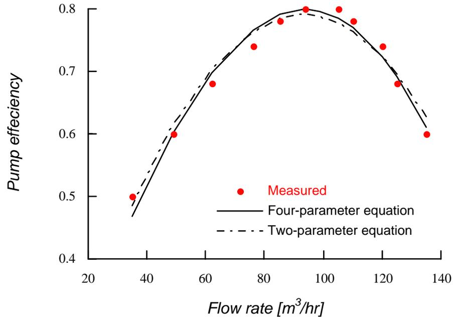
**Figure 3.1.5** Curve fitting a measured pump efficiency as a function of flow rate using the four-parameter model and the two-parameter model. Data adapted from ASHRAE (1983).
