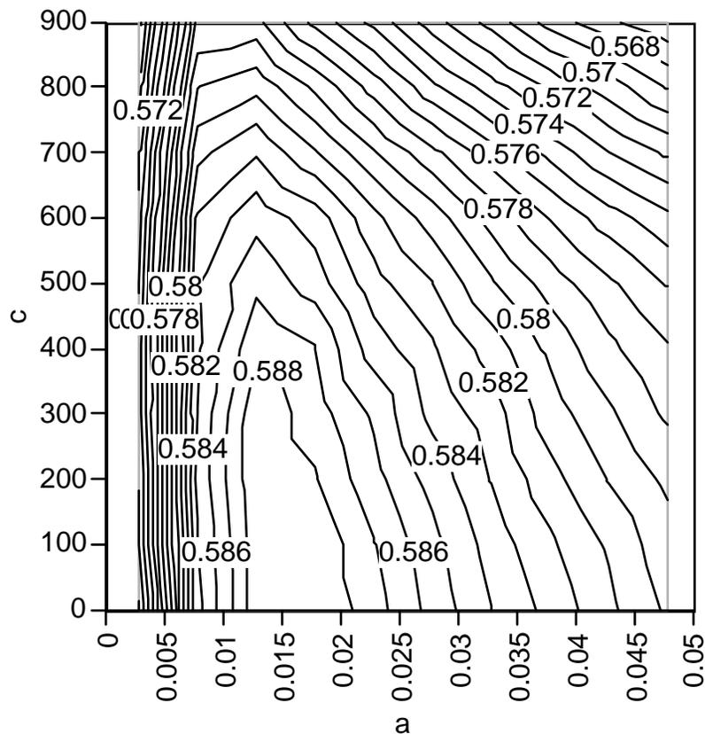
**Figure 6.1.14** Contour plot of the annual solar fraction as a function of  $a$  and  $c$  for a heat exchanger with higher effectiveness range.
