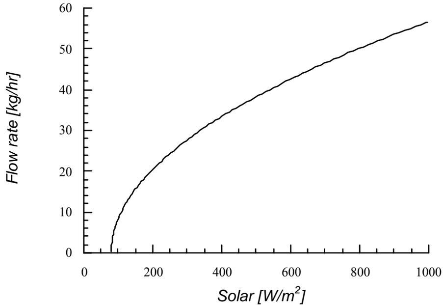
**Figure 5.1.3** The optimum flow rate profile of the base system.
