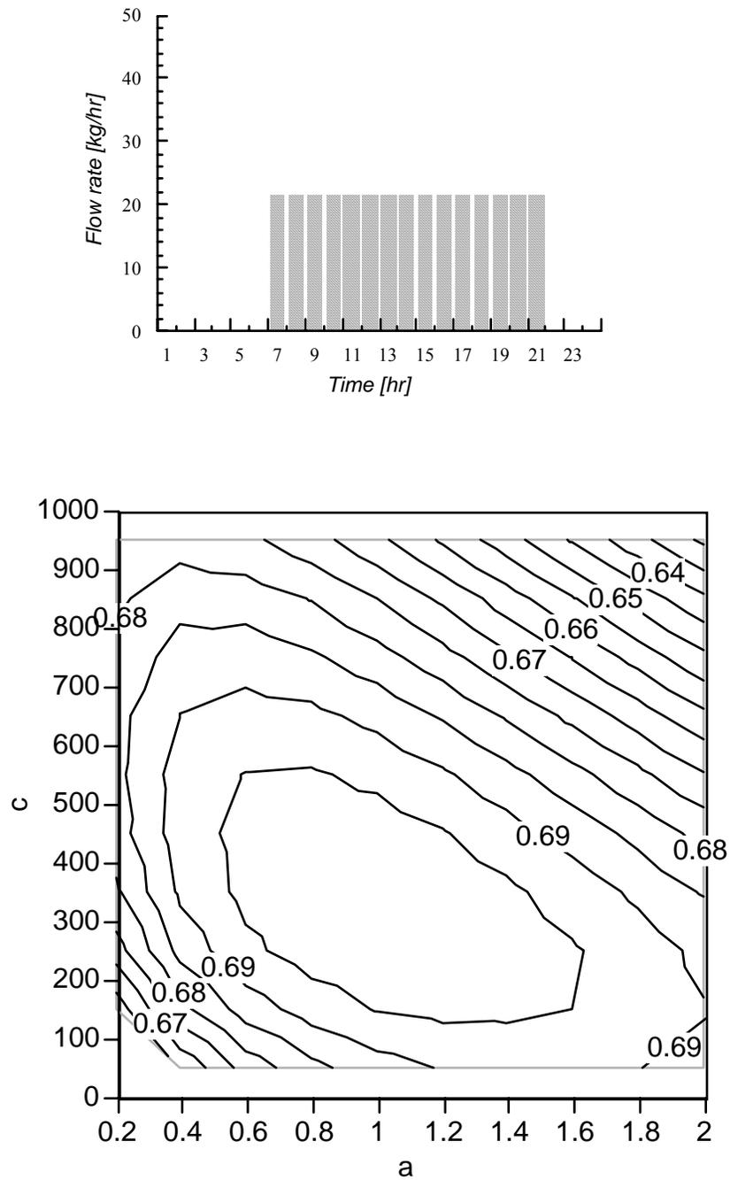
**Figure 5.1.9** Contour plot of the annual solar fraction of the base system as a function of the parameters  $a$  and  $c$ . The load profile is defined as a square function with a daily integral value of 300 kg of water.
