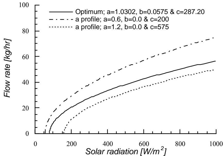
**Figure 5.1.8** The window of the optimum flow rate profiles that will yield an annual solar fraction of at least 0.69.
