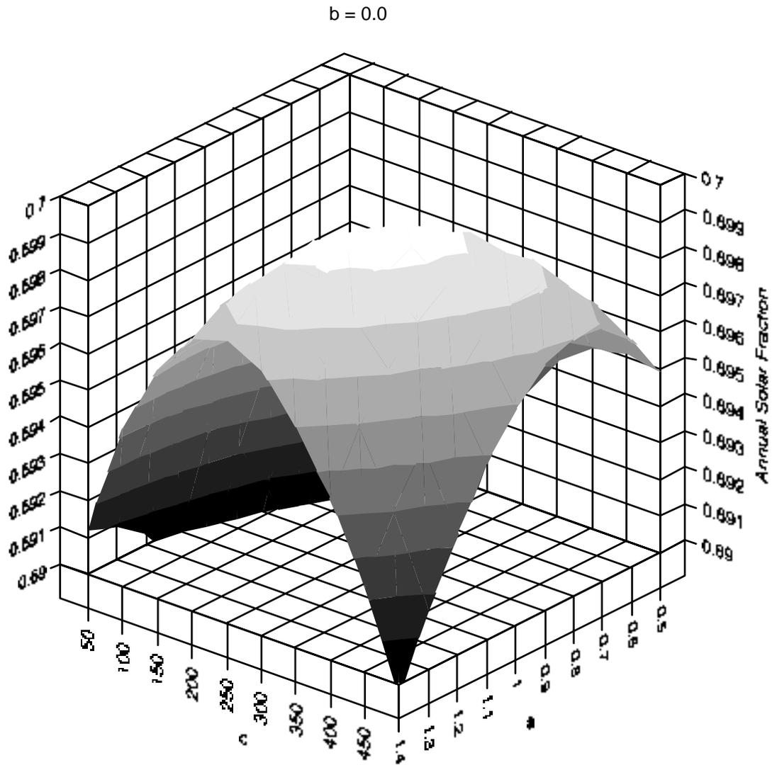
**Figure 5.1.6** Graph of the annual solar fraction of the base system as a function of the parameters  $a$  and  $c$ . The value of the parameter  $b$  is set to 0.
