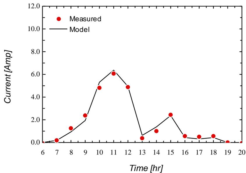
**Figure 3.4.8** Current of FSEC PV pumping system as a function of time. Data measured on September 3rd, 1987. Data reported by FSEC.
