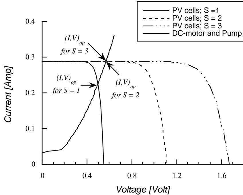
**Figure 5.2.8** Three  $I$ - $V$  curves of three PV cells (for  $S = 1, 2$  and  $3$ ) and the  $I$ - $V$  curve of the attached DC-motor-pump load.
