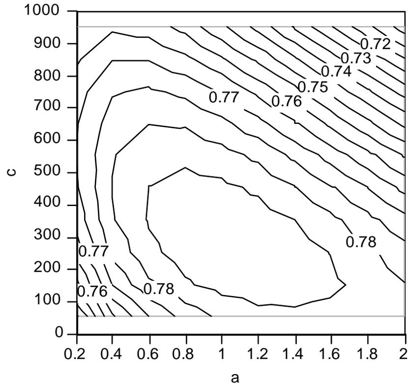
**Figure 5.1.23** Contour plot of the annual solar fraction of the base system if located in Washington, DC.
