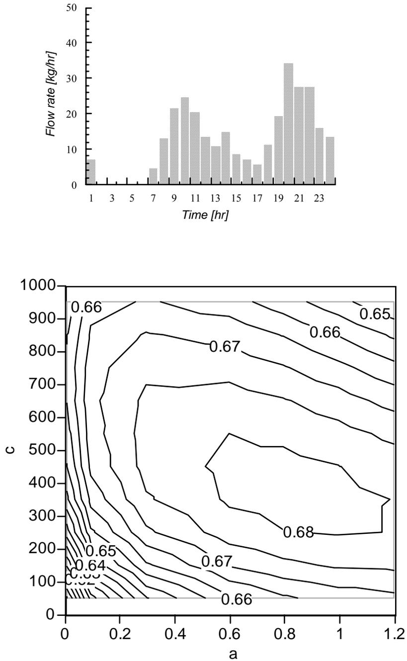
**Figure 5.1.12** Contour plot of the annual solar fraction of the base system as a function of the parameters  $a$  and  $c$ . The load profile is represented by the standard RAND flow profile with a total daily water draw of 300 kg.
