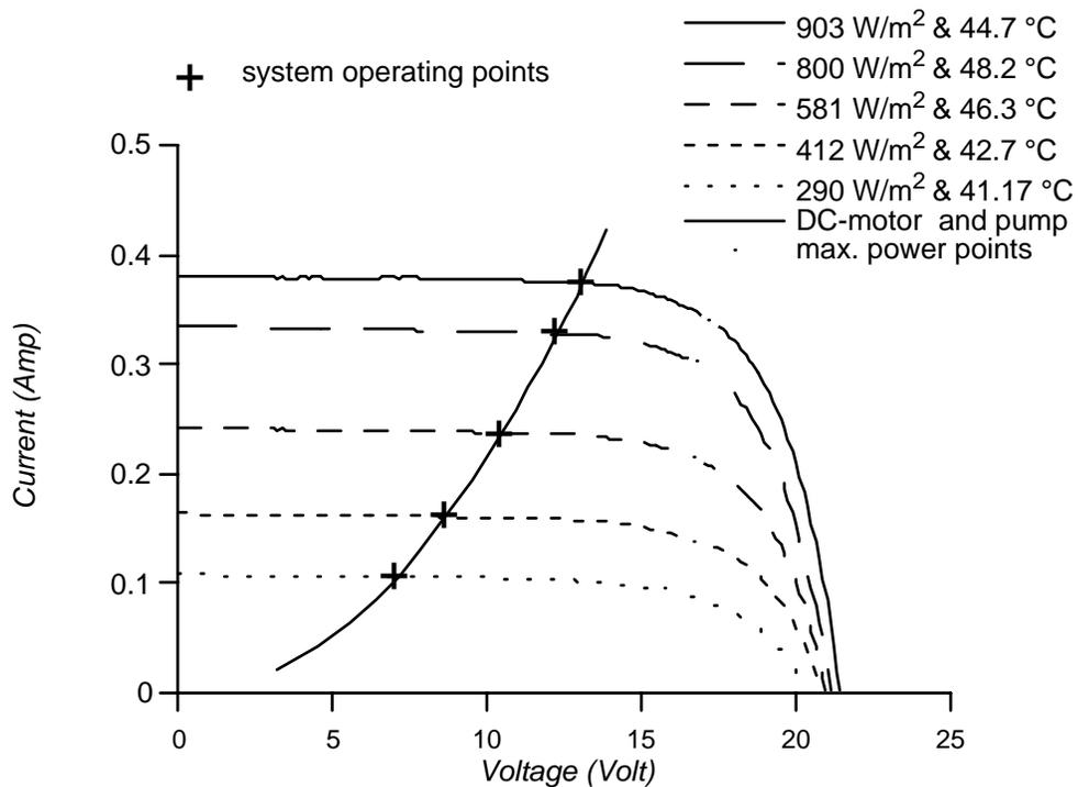
**Figure 1.2.3** The effect of solar radiation intensity and cell temperature on PV  $I$ - $V$  curves and PV system operating points.
