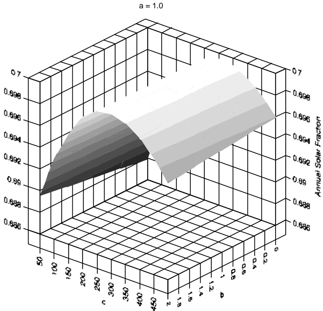
**Figure 5.1.4** Graph of the annual solar fraction of the base system as a function of the parameters  $b$  and  $c$ . The value of the parameter  $a$  is set to 1.
