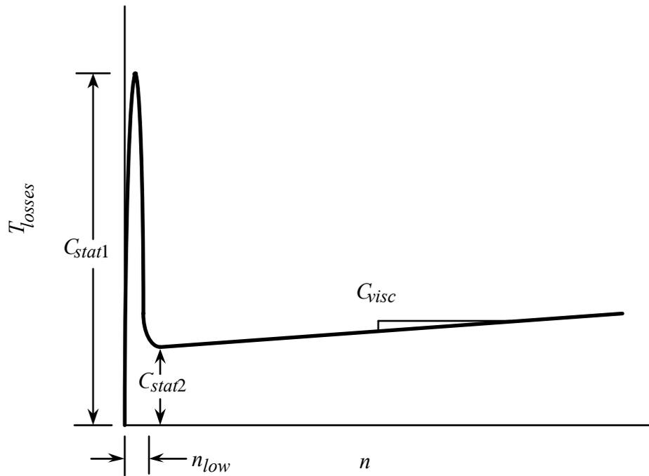
**Figure 3.1.3** The general torque losses profile as a function of the shaft speed. Drawing is not to-scale.
