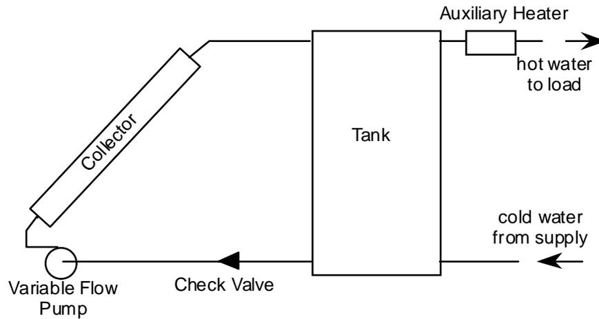
**Figure 5.1.1** Schematic drawing of the base system in phase one.
