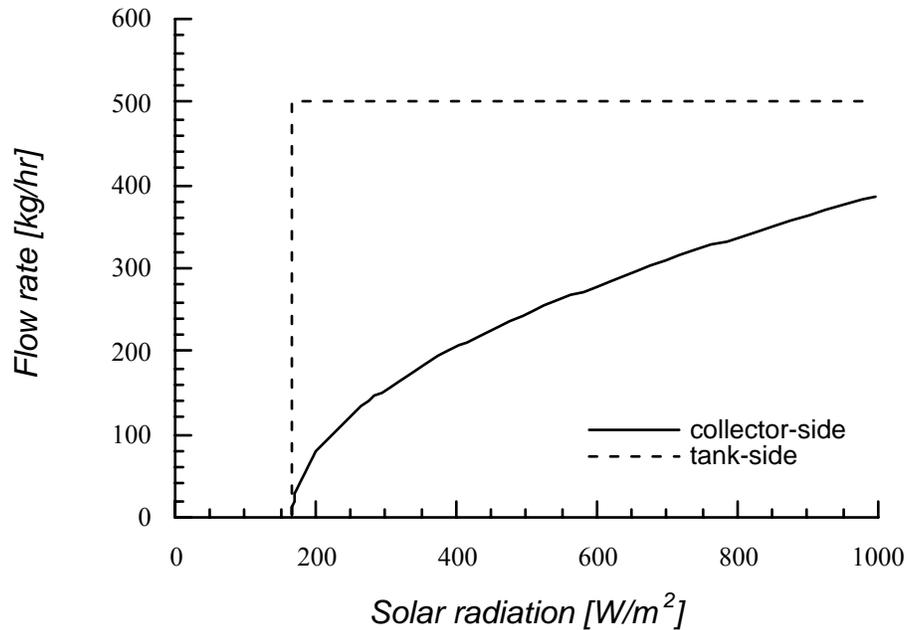
**Figure 6.1.8** The optimum collector-side flow rate profile of the modified system and the tank-side flow rate profile.
