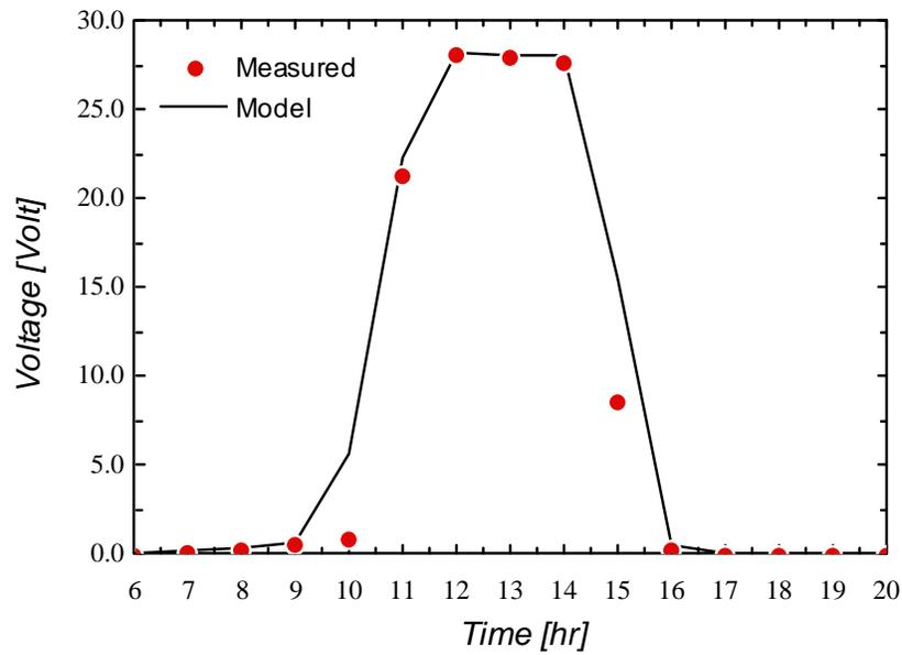
**Figure 3.4.11** Voltage of FSEC PV pumping system as a function of time. Data measured on September 5th, 1987. Data reported by FSEC.
