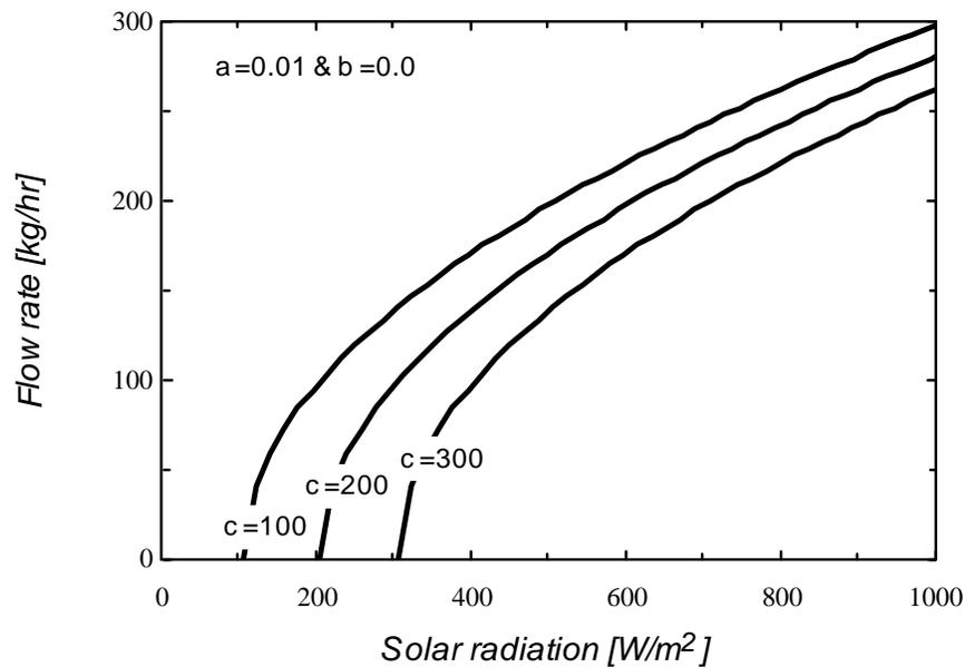
**Figure 4.3.6** The effect of the parameter  $c$  on the general flow rate profile of PV pumping systems.
