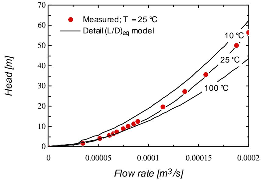
**Figure 3.1.7** Simulated  $H-Q$  curves of an SDHW system at three collector fluid temperatures compared to the measure  $H-Q$  data. The collector fluid is water.
