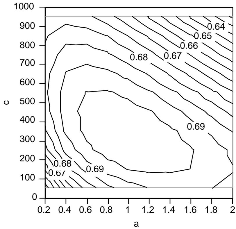
**Figure 5.1.20** Contour plot of the annual solar fraction of the base system if located in Madison, WI.
