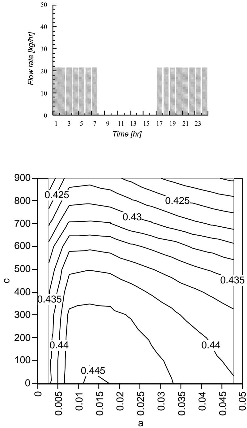
**Figure 6.1.12** The shifted load profile and the contour plot of the annual solar fraction of the base system as a function of the parameters  $a$  and  $c$ .
