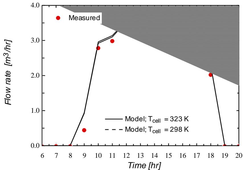
**Figure 3.4.18** The effect of the PV cell temperature on the flow rate of FSEC system. Data reported by FSEC.
