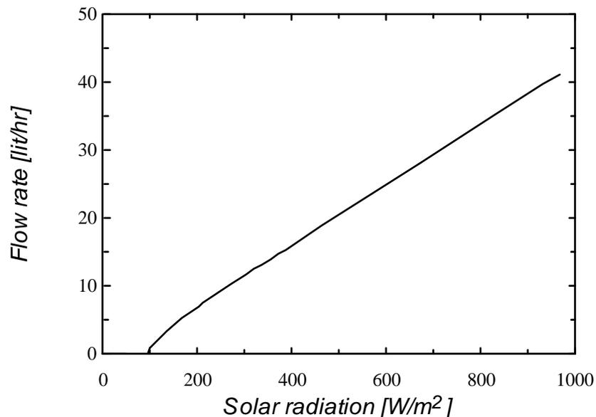
**Figure 2.3.1** Flow rate profile of the strategy of varying the flow proportionally to the utilizable radiation in Wuestling *et al.*'s SDHW system.
