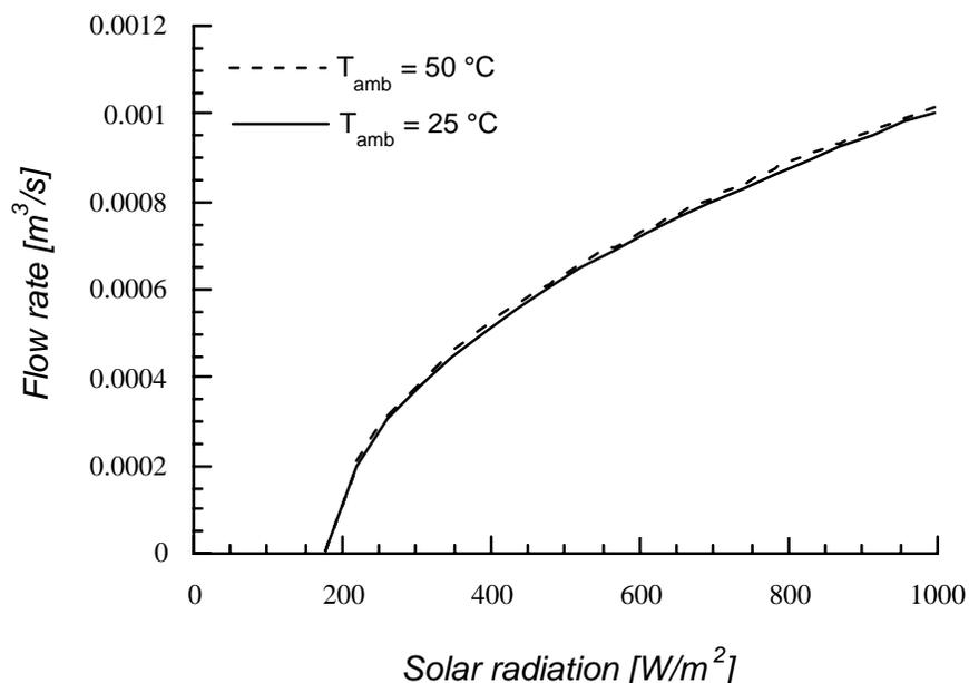
**Figure 1.2.4** Typical flow rate profiles of a direct-coupled PV pumping system.
