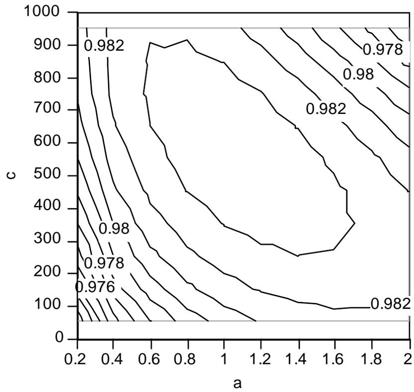
**Figure 5.1.22** Contour plot of the annual solar fraction of the base system if located in Albuquerque, NM.
