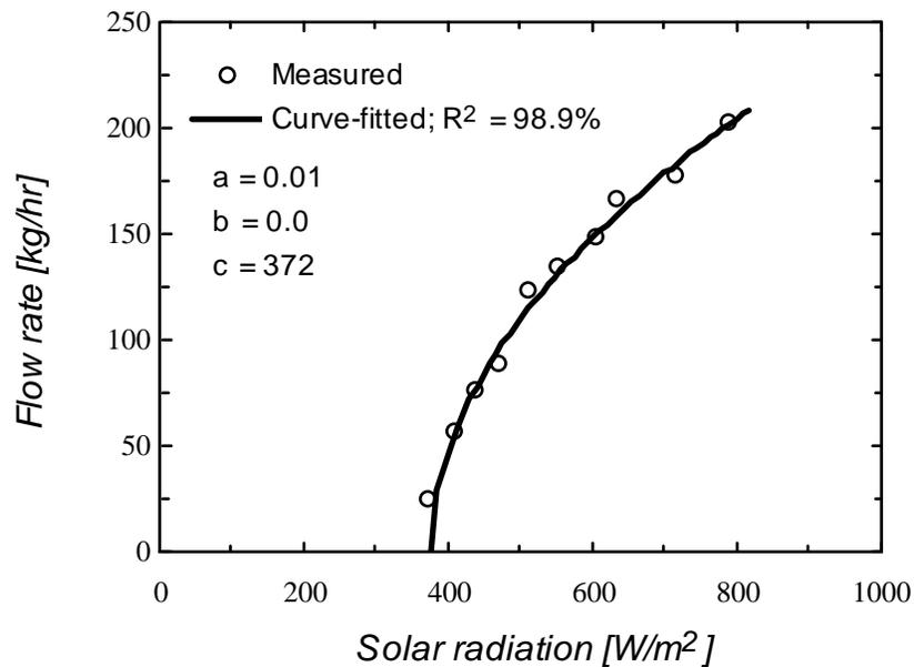
**Figure 4.3.1** Measured and curve-fitted flow rate profile of a PV pumping system. Data obtained from Litka and Chandra (1979).
