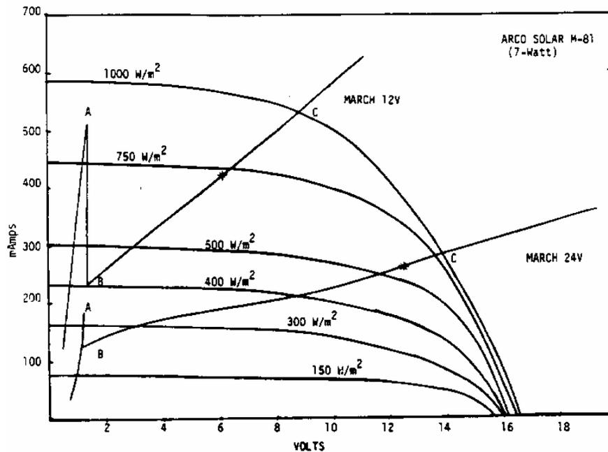
**Figure 3.1.2** I-V curves of a PV cells and two different DC-motor-pump loads. From Cromer (1984).
