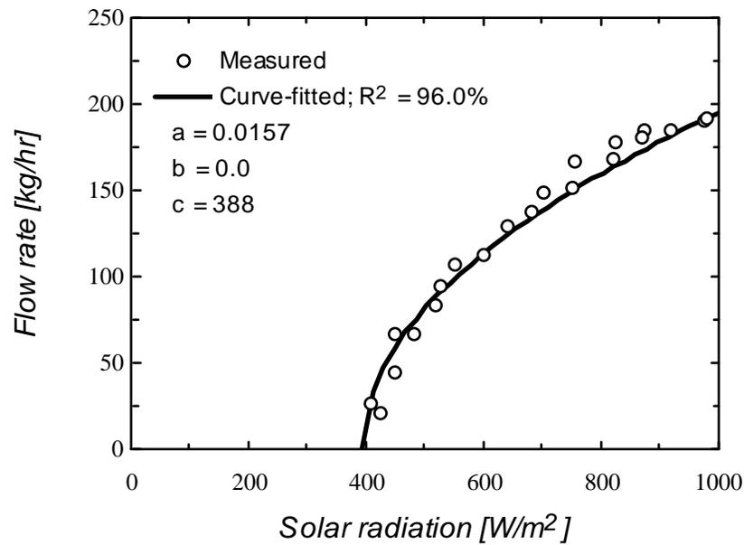
**Figure 4.3.2** Measured and curve-fitted flow rate profile of a PV pumping system. Data obtained from Cromer (1983).
