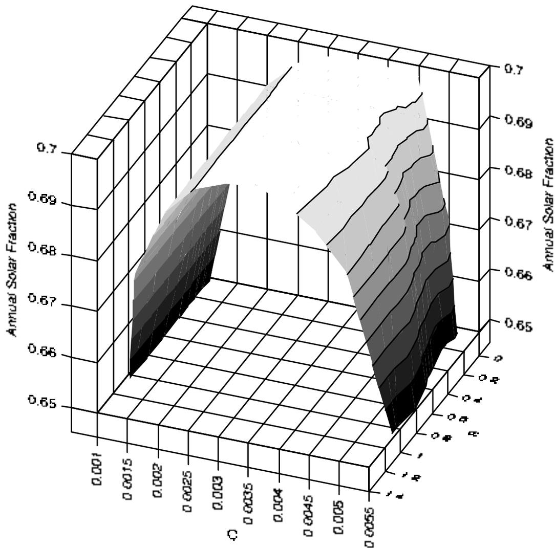
**Figure 5.2.11** The annual solar fraction of a PV-SDHW system as a function of  $C$  and  $R$ .  $Type = 2$ ,  $P = 1$  and  $S = 2$ .
