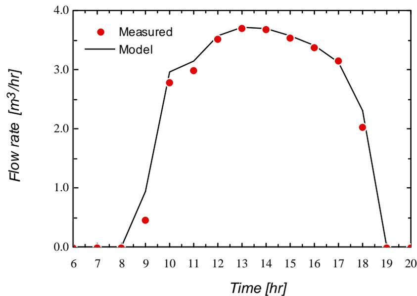
**Figure 3.4.1** Flow rate produced by FSEC PV pumping system as a function of time. Data measured on August 23rd, 1987. Data reported by FSEC.
