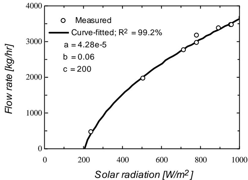
**Figure 4.3.3** Measured and curve-fitted flow rate profile of a PV pumping system. Data reported by FSEC (August 23rd, 1987).
