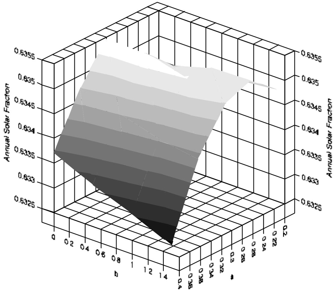
**Figure 6.2.4** Graph of the annual solar fraction as a function of  $a$  and  $b$ , for  $c$  equal zero.
