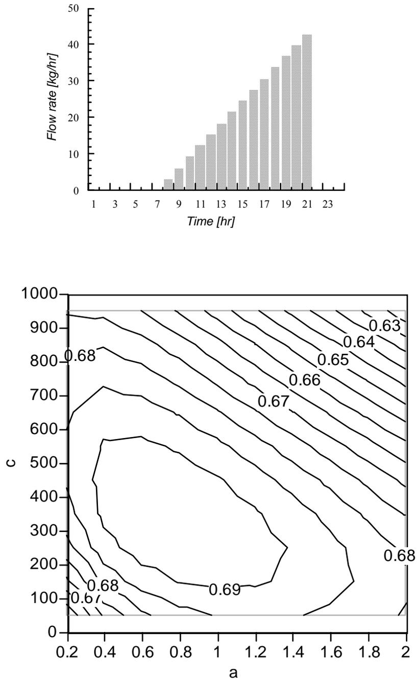
**Figure 5.1.11** Contour plot of the annual solar fraction of the base system as a function of the parameters  $a$  and  $c$ . The load profile is defined as a triangular
