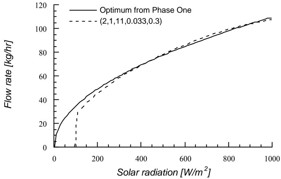
**Figure 6.2.8** The optimum flow rate found in phase one and the flow rate resulting from the optimum PV pumping system found in phase two.
