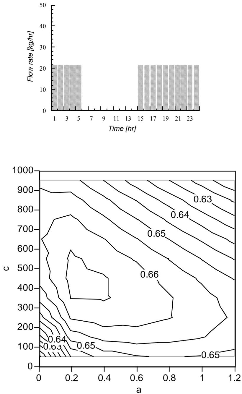
**Figure 5.1.18** Contour plot of the annual solar fraction of the base system as a function of the parameters  $a$  and  $c$ . The load profile has a time-lag of 8 hours from the standard system (Run # 5).
