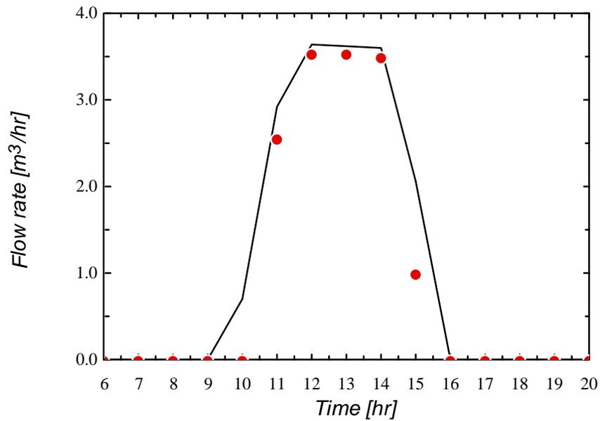
**Figure 3.4.9** Flow rate of FSEC PV pumping system as a function of time. Data measured on September 5th, 1987. Data reported by FSEC.
