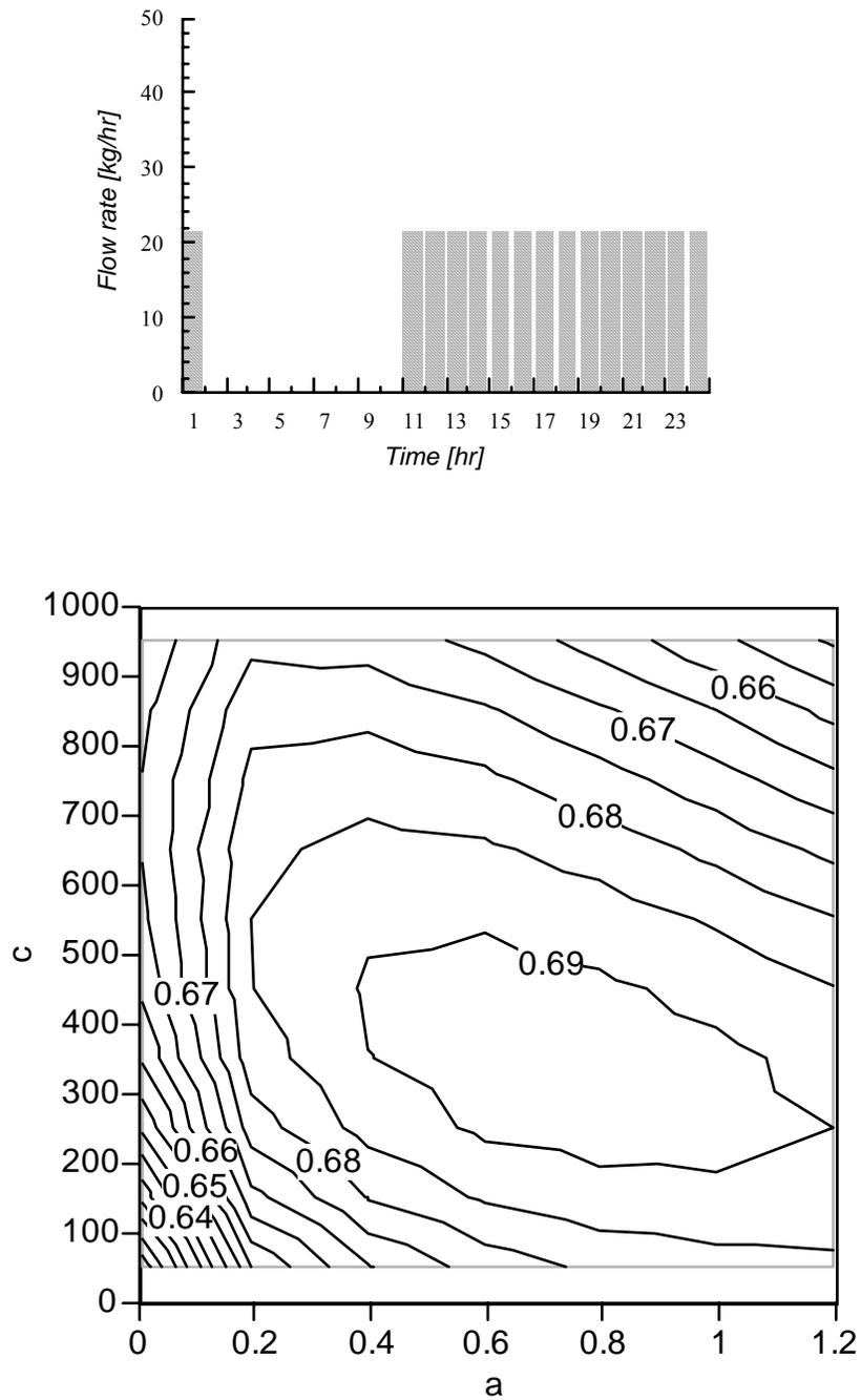
**Figure 5.1.16** Contour plot of the annual solar fraction of the base system as a function of the parameters  $a$  and  $c$ . The load profile has a time-lag of 4 hours from the standard system (Run # 3).
