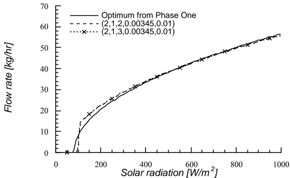
**Figure 5.2.7** The flow rate profile generated from the proposed optimum PV pumping system using  $S = 2$  and  $3$  compared to the optimum flow rate profile found in phase one.
