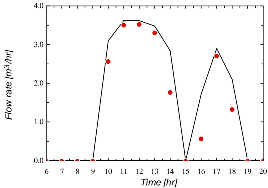
**Figure 3.4.13** Flow rate of FSEC PV pumping system as a function of time. Data measured on September 7th, 1987. Data reported by FSEC.
