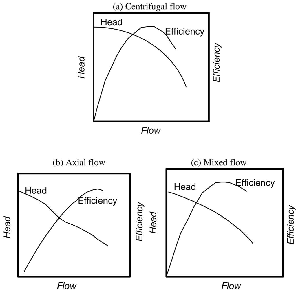
**Figure 3.1.4** The  $H-Q$  and  $\eta-Q$  curves for the rotary type pumps: (a) centrifugal flow; (b) axial flow; and, (c) mixed flow.
