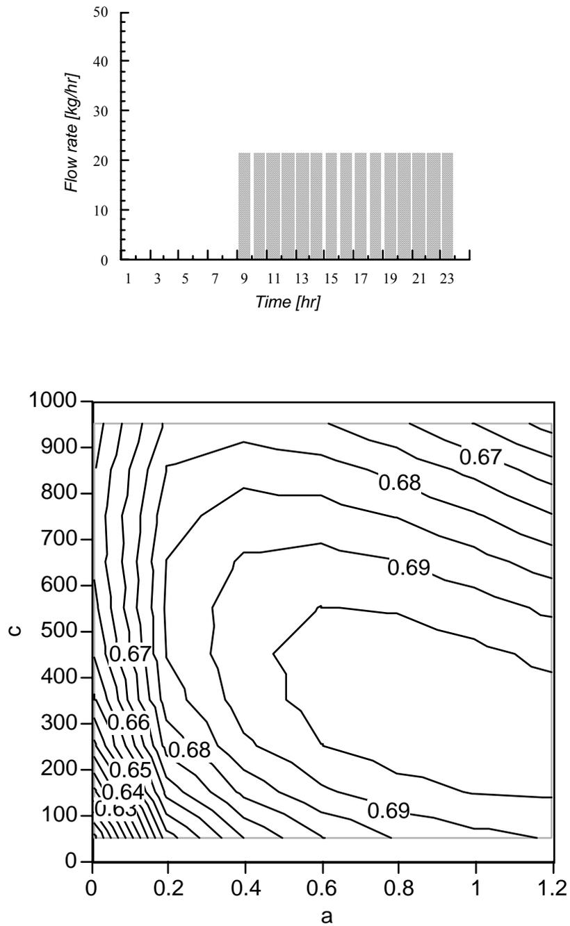
**Figure 5.1.15** Contour plot of the annual solar fraction of the base system as a function of the parameters  $a$  and  $c$ . The load profile has a time-lag of 2 hours from the standard system (Run # 2).
