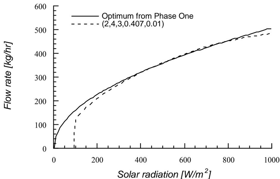
**Figure 6.1.17** The optimum flow rate profile found in phase one and the flow rate profile resulting from the optimum PV pumping system found in phase two.
