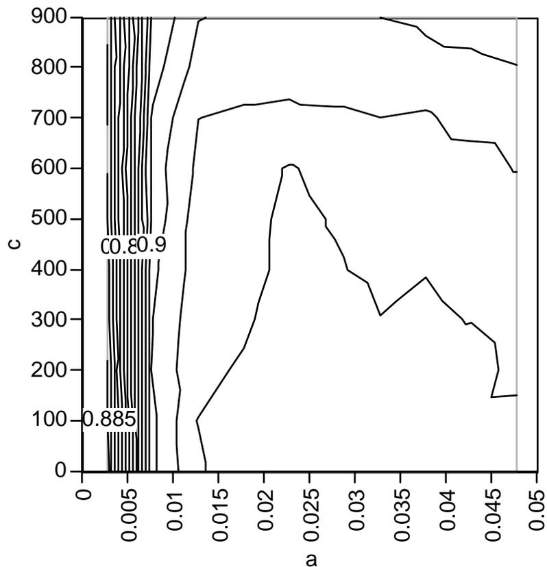
**Figure 6.1.13** Contour plot of the annual solar fraction of the system if located in Albuquerque, NM.
