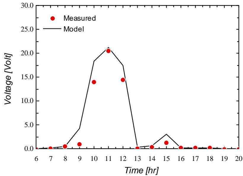
**Figure 3.4.7** Voltage of FSEC PV pumping system as a function of time. Data measured on September 3rd, 1987. Data reported by FSEC.
