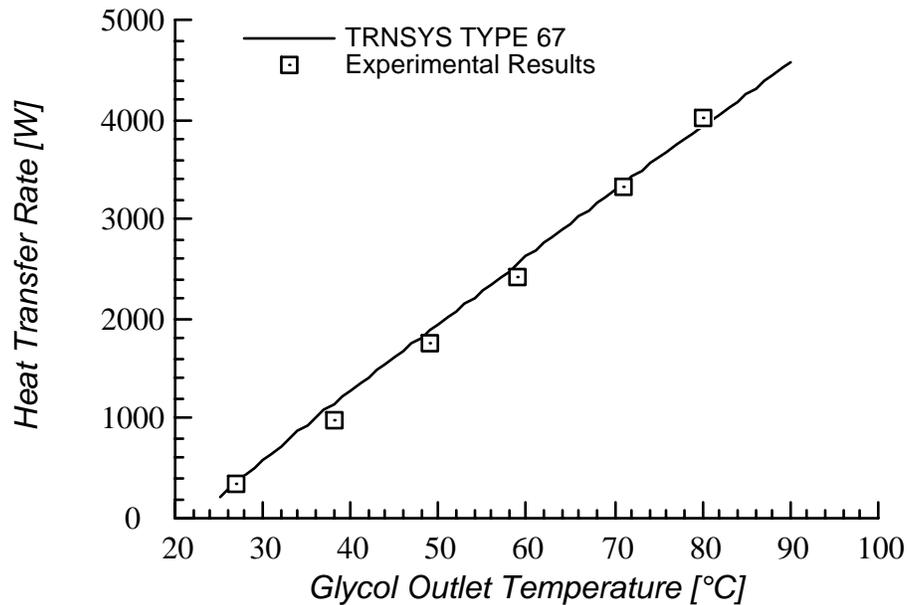
**Figure 3.2.1** Comparison of TRNSYS TYPE 67 results to Fraser's experimental results. From Avina (1994).
