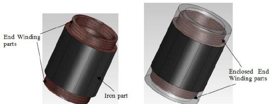
Fig.2.16. End winding cooling with magnetic fluid [72]
