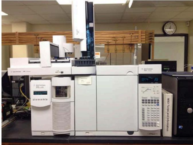
Figure 2.1  $1\mu\text{L}$  of the analyte will be injected into the Agilent gas chromatography mass spectrometry for analysis.
