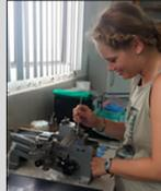
Figure 2 (right). Morgan Freeburg using the microtome to make microscope slides.
