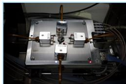
Newly installed 4-point probe system in a Hitachi 3400 N Scanning Electron Microscope
