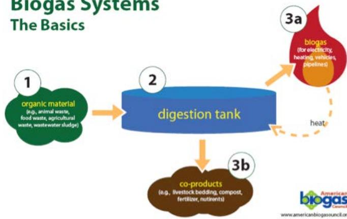
**Figure 2** The Anaerobic Digestion System (Source: American Biogas Council)
