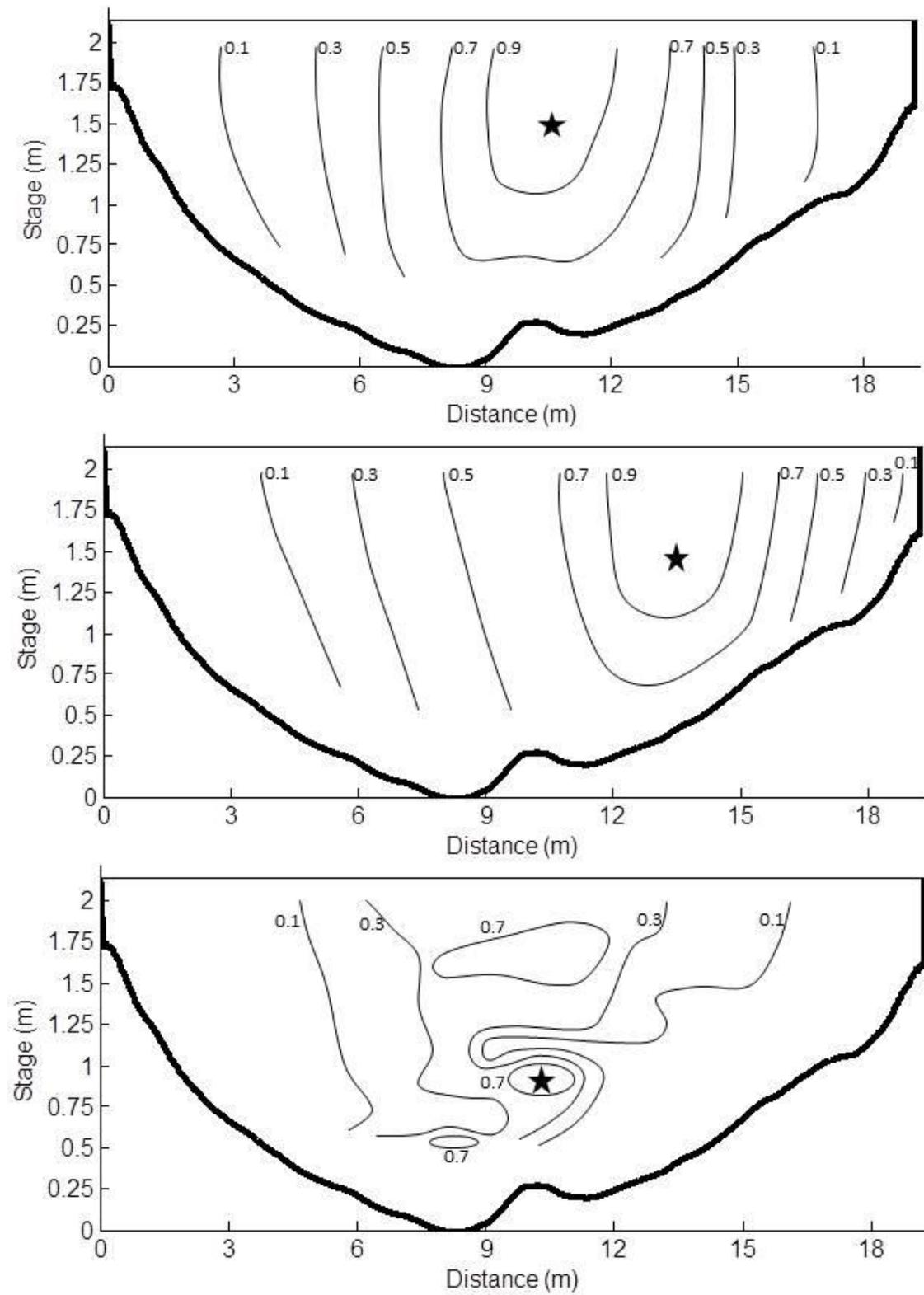
**Figure 7:** Relative velocity contours for positive flows (1 to 4 m<sup>3</sup>/s), negative flow (-5 to -6.5 m<sup>3</sup>/s), and low flows (0 to 1 m<sup>3</sup>/s).
