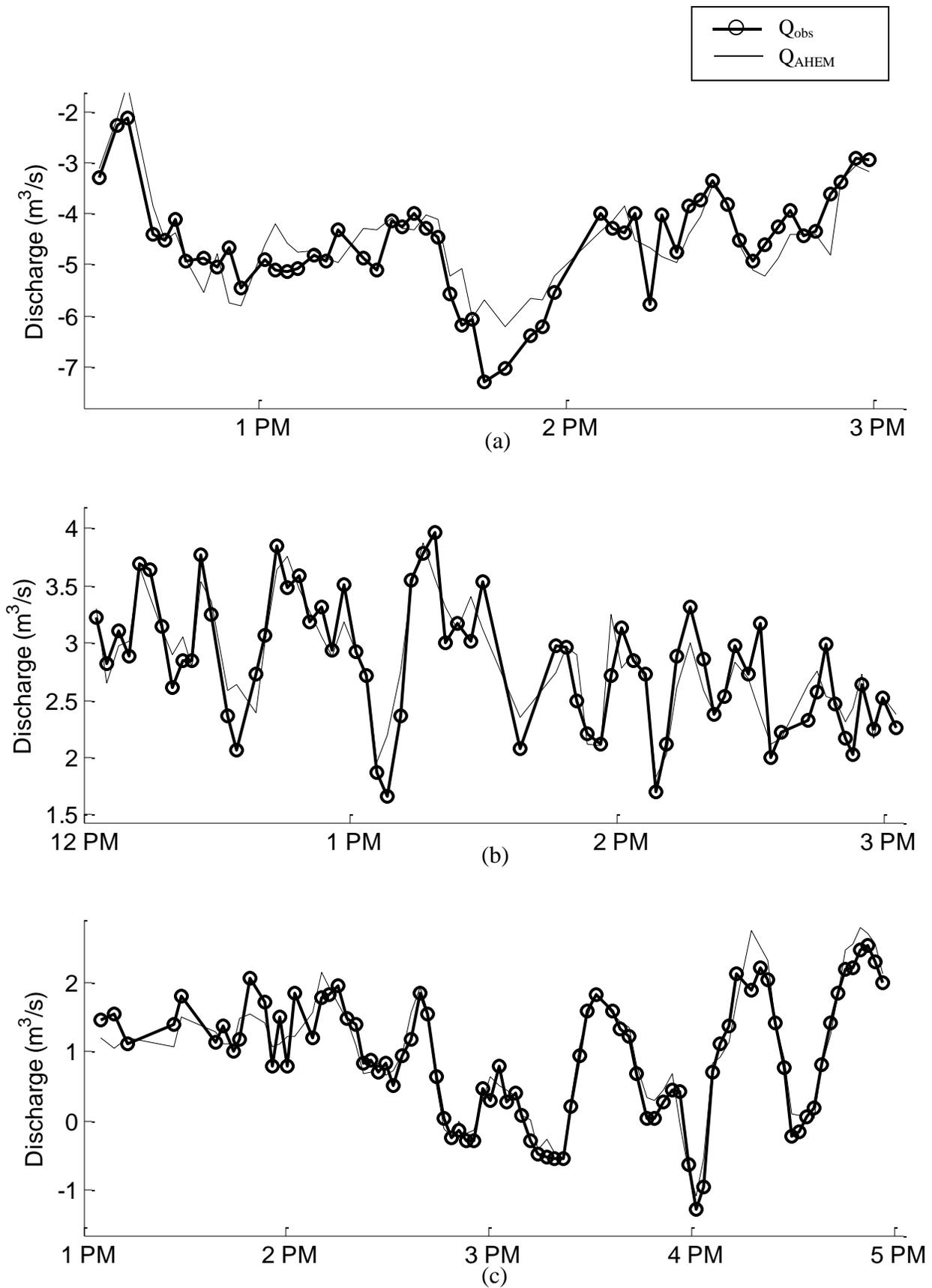
**Figure 9:** Measured and estimated discharge time series for three flow regimes: (a) negative, September 19<sup>th</sup>, (b) positive, October 15<sup>th</sup>, (c) transitional, October 24<sup>th</sup> (validation set)
