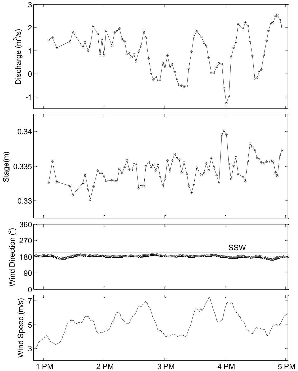
**Figure 4:** Discharge time series for a reverse flow event.
