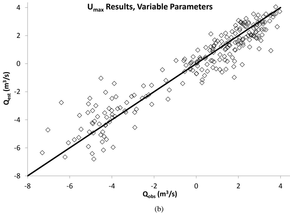
**Figure 12:**  $Q_{\text{est}}$  vs  $Q_{\text{obs}}$  when using conventional entropy with constant parameters (a) and variable parameters (b).
