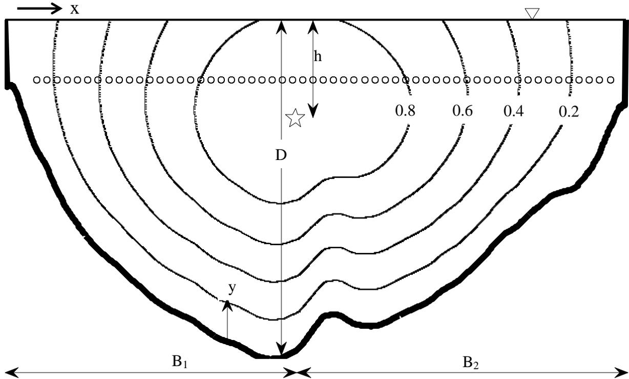
**Figure 1:** 2-D velocity distribution where  $M=-2$ ,  $\beta=1$ , and  $h/D=0.4$ . HADCP velocities are collected at the same depth and denoted with (o).
