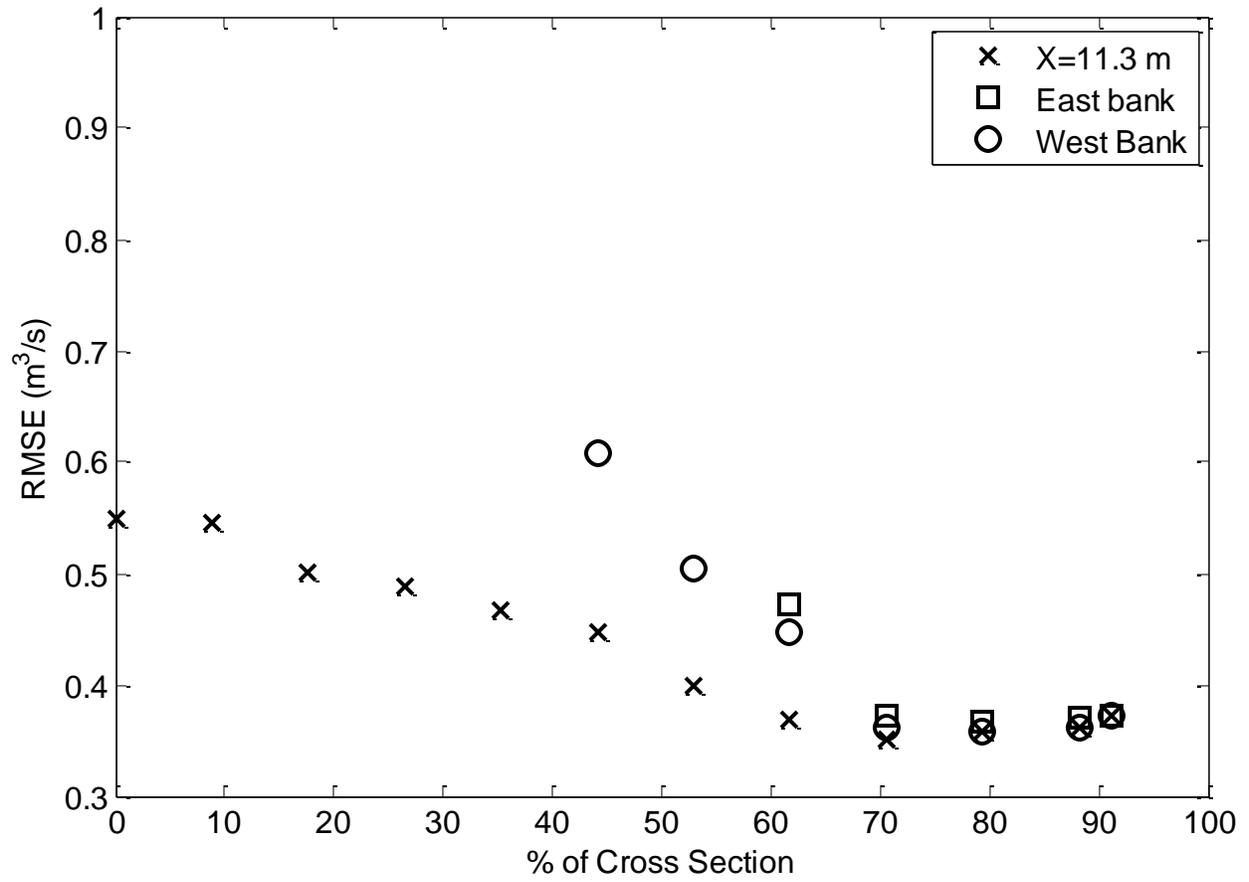
**Figure 13:** RMSE( $\text{m}^3/\text{s}$ ) is calculated as the percentage of measured cross section increases.
