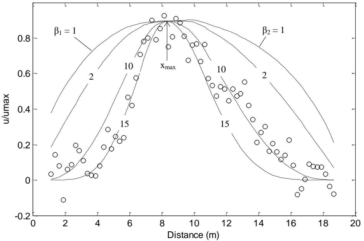
**Figure 2:** Example of fitting beta values to relative velocity measurements of the HADCP. An increase in beta will narrow the velocity distribution towards the maximum. For this example,  $\beta_1 = 15$  and  $\beta_2 = 10$ .
