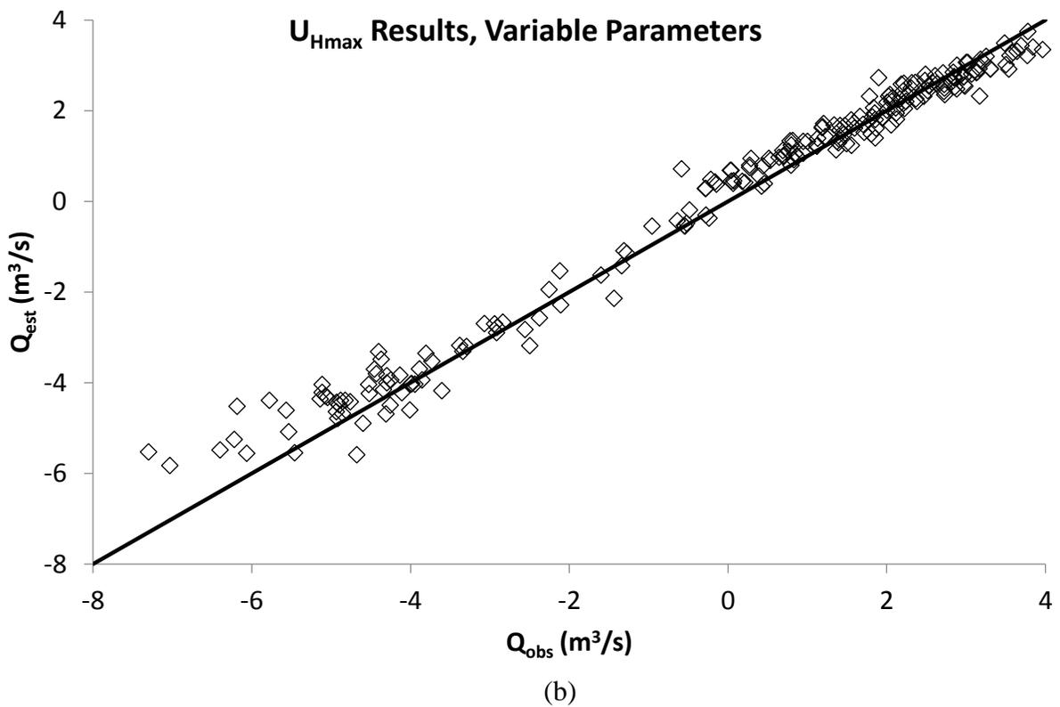
**Figure 11:**  $Q_{est}$  vs  $Q_{obs}$  when using AHM with the maximum HADCP velocity ( $U_{Hmax}$ ) and constant parameters (a) and variable parameters (b).
