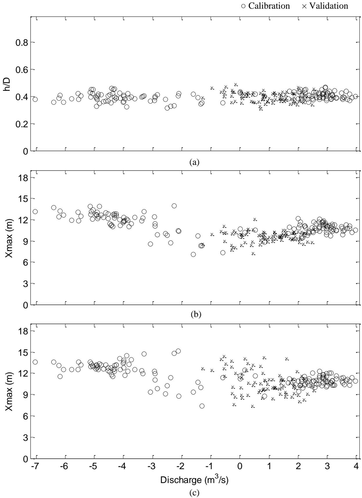
**Figure 6:** Plot of (a)  $h/D$  determined from VADCP data, (b)  $x_{\max}$  determined from HADCP data, (c)  $x_{\max}$  determined from VADCP data
