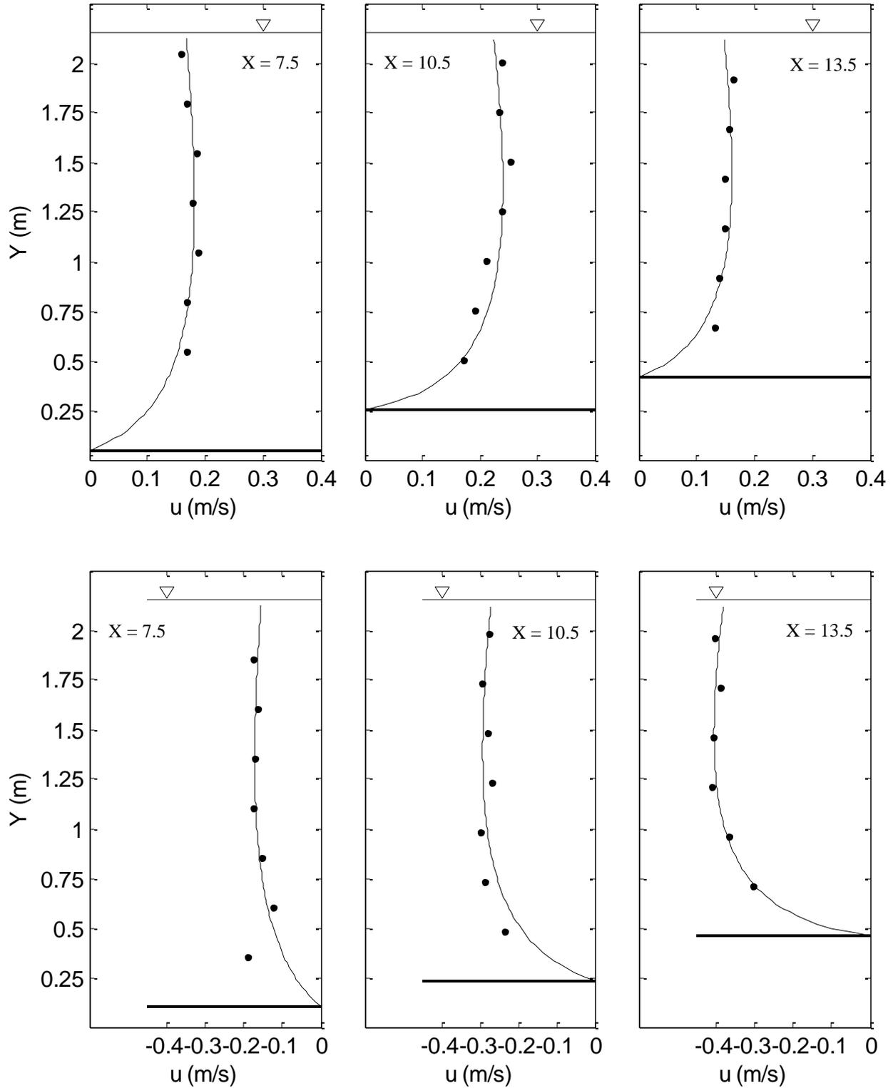
**Figure 5:** (Top) Fit velocity profiles for positive flows (top, 3 to 4 m<sup>3</sup>/s) and negative flows (bottom, -5 to -6.5 m<sup>3</sup>/s).  $M=2$ , and  $h/d = 0.4$  for all profiles.
