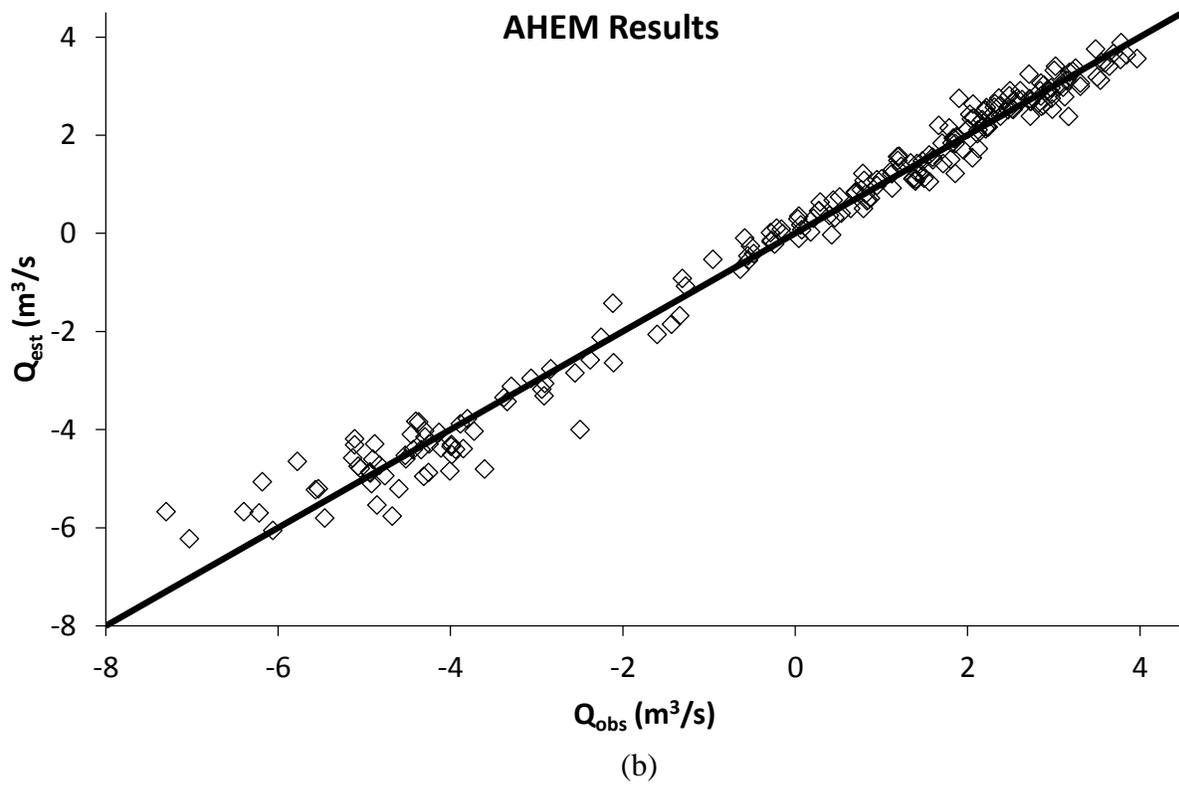
**Figure 10:**  $Q_{est}$  vs  $Q_{obs}$  when using the Index Velocity Method (a) and AHEM (b).
