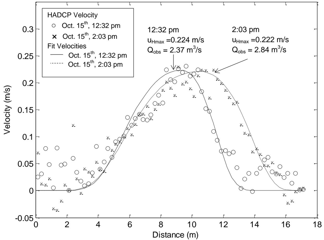
**Figure 8:** An example of an observed change in horizontal velocity distribution. Maximum velocities are similar, but discharges change significantly. Assuming a constant ratio between  $u_{max}$  and  $\bar{u}$  would not be appropriate for this case.
