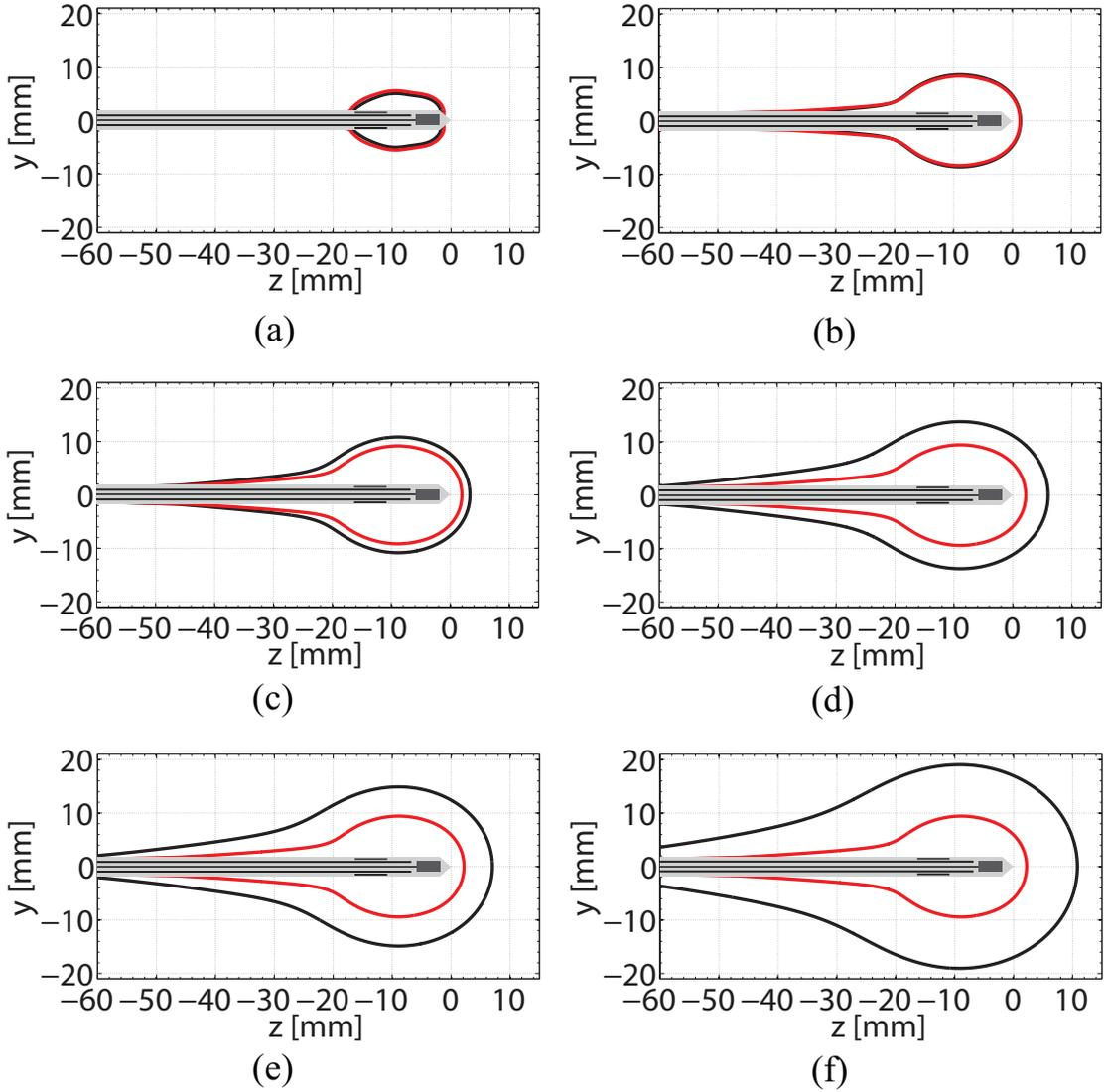
Figure 3: Transient thermal simulations show the expanding heating zone of the 10 GHz antenna at (a) 10 seconds, (b) 1 min., (c) 2 min., (d) 4 min., (e) 5 min., and (f) 10 min. The black contour represents the 60°C boundary from the *ex vivo* simulation (no metabolic heat generation or blood perfusion). The red contour represents the 60°C boundary from the *in vivo* simulation (including the effects of metabolic heat generation and blood perfusion).
