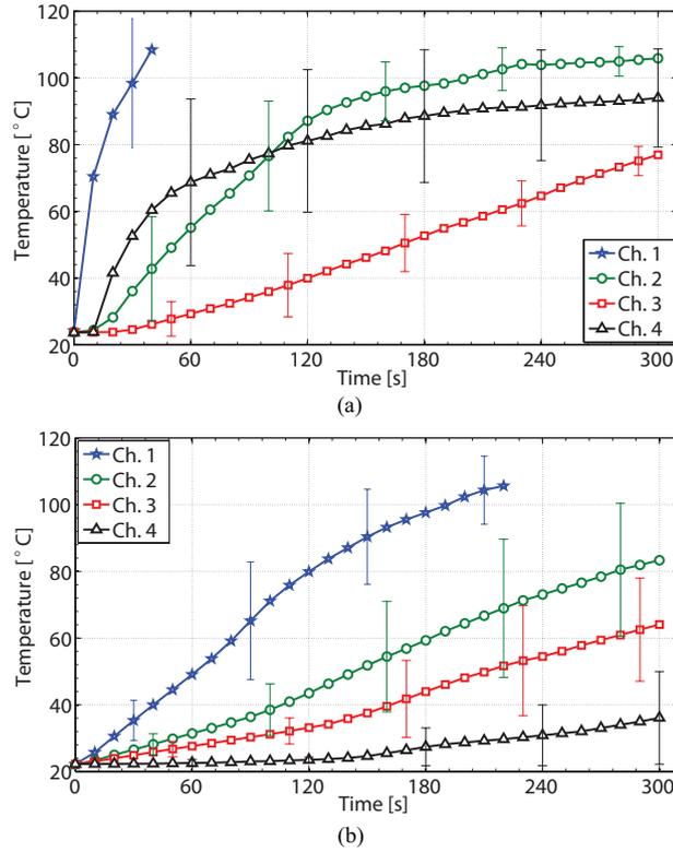
Figure 8: Average temperature values recorded at each channel during the first 5 minutes of all of the (a) 10 GHz and (b) 1.9 GHz ablation experiments. The bars show standard deviations. When a temperature level recorded by any of the sensors reached  $120^\circ$ , that sensor was removed from the ablation zone to avoid damaging it. Therefore, the data plotted for Ch. 1 is terminated before 5 minutes.
