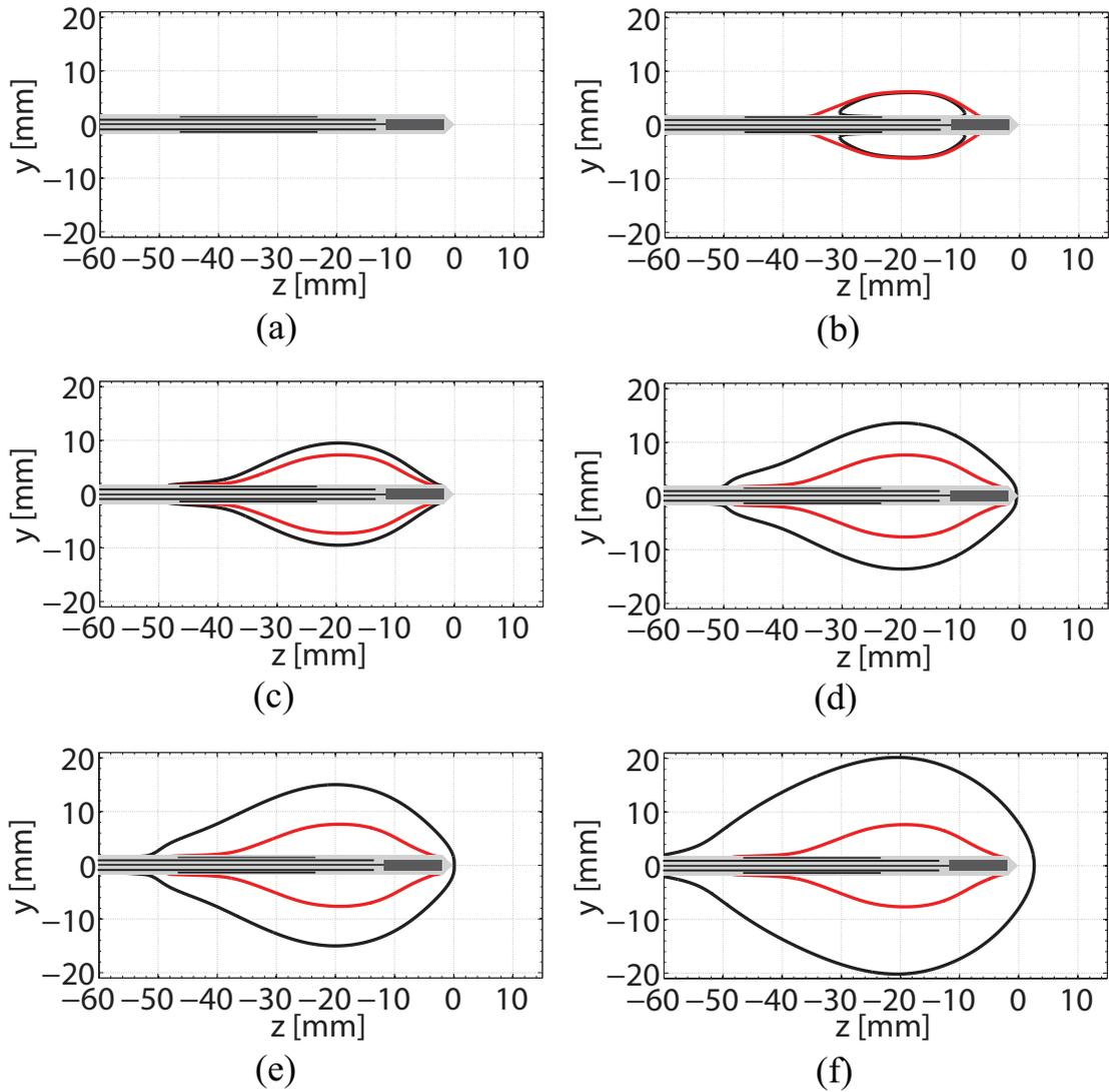
Figure 4: Transient thermal simulations show the expanding heating zone of the 1.9 GHz antenna at (a) 10 seconds, (b) 1 min., (c) 2 min., (d) 4 min., (e) 5 min., (f) 10 min. The black contour represents the 60°C boundary from the *ex vivo* simulation. The red contour represents the 60°C boundary from the *in vivo* simulation.
