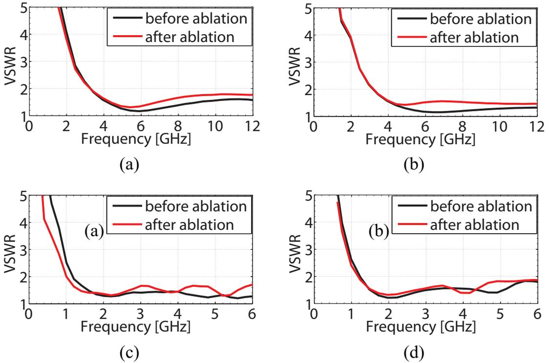
Figure 5: VSWR measurement results of (a) 10 GHz FSD antenna in 5-min.-ablation experiment, (b) 10 GHz FSD antenna in 10-min.-ablation experiment, (c) 1.9 GHz antenna in 5-min.-ablation experiment, and (d) 1.9 GHz antenna in 10-min.-ablation experiment.
