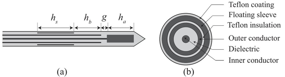
Figure 1: Topology of the floating sleeve dipole (FSD) antenna used in the ablation experiments. (a) Side view. (b) Cross-sectional view. The outer diameters of the various layers are as follows: inner conductor = 0.515 mm, dielectric = 1.676 mm, outer conductor = 2.2 mm, Teflon insulator = 2.5 mm, floating sleeve = 3.2 mm, Teflon coating = 3.5 mm.
