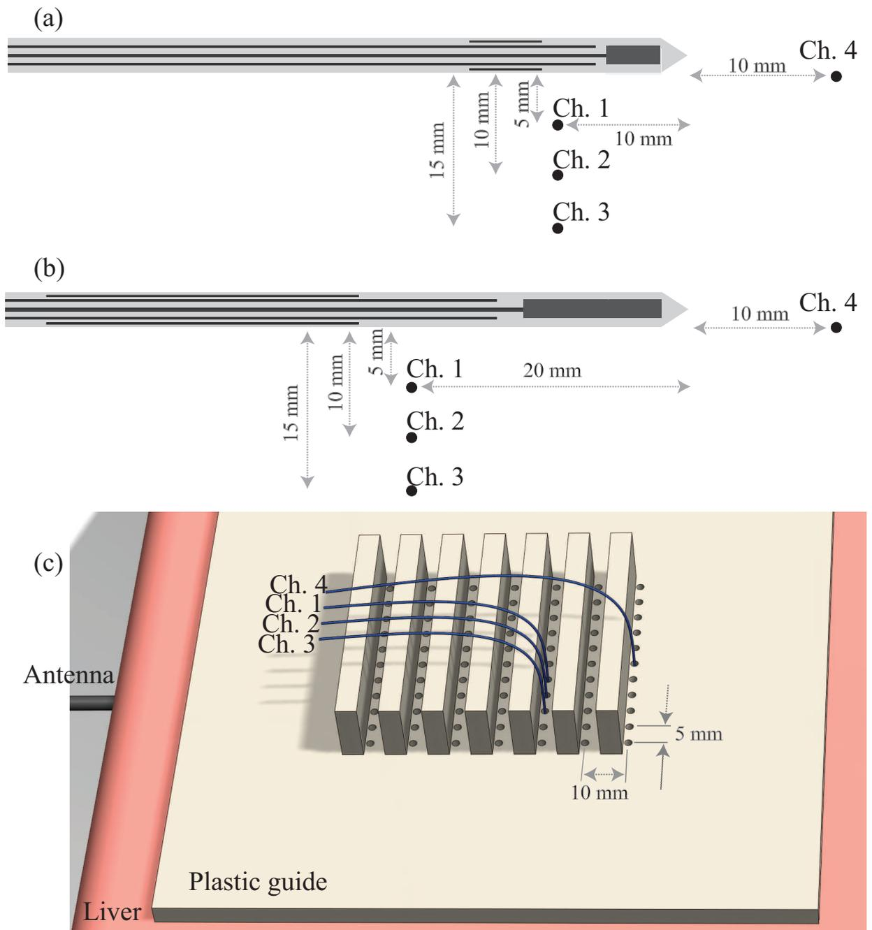
Figure 6: Positions of the four temperature probes. (a) Cross-sectional view (horizontal plane) of the 10.0 GHz antenna. (b) Cross-sectional view (horizontal plane) of the 1.9 GHz FSD antenna. (c) 3D view of the plastic guide used to position the probes.
