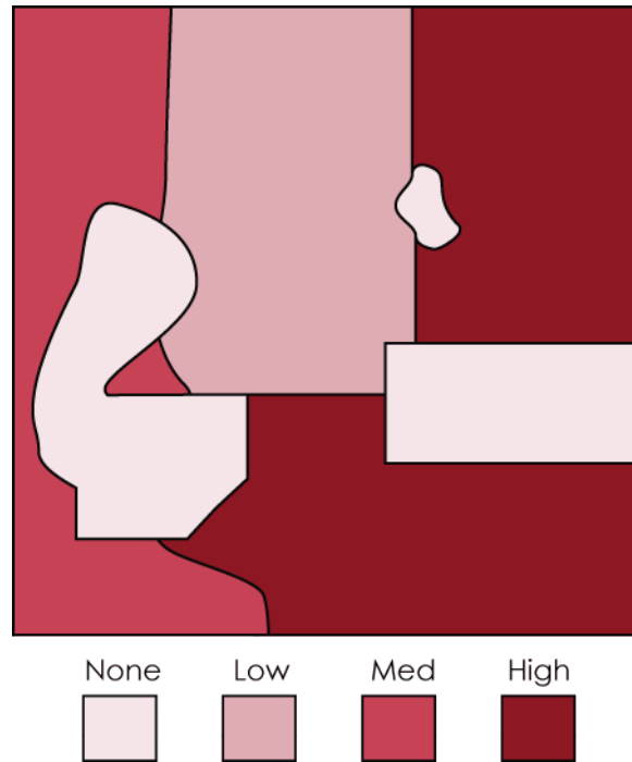
Figure 5: Dasymetric Map displayed with boundaries between adjacent polygons of the same category dissolved.
