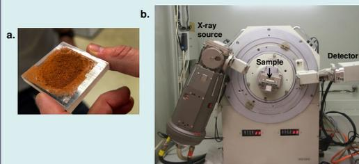
Figure 4: Photos of (a) mounted powder sample, and (b) the D500 Powder X-Ray Diffractometer.
