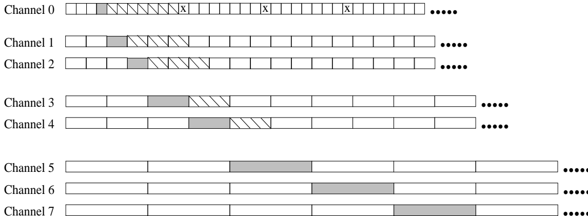
Figure 1. Example Skyscraper Transmission Schedule. ( K = 8 ; W = 8 )
