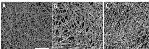
**Fig. 3: Scanning electron microscopy images of randomly oriented encapsulated poly ( $\epsilon$  caprolactone) nanofiber scaffolds. Scaffolds containing (A) 0.1% retinoic acid (w/w); (B) 0.2% retinoic acid (w/w) and (C) 0.3% retinoic acid (w/w). Scale bar is  $5\ \mu\text{m}$ .**
