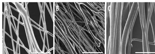
**Fig. 4: Scanning electron microscopy images of aligned encapsulated poly ( $\epsilon$  caprolactone) nanofiber scaffolds. Scaffolds containing (A) 0.1% retinoic acid (w/w); (B) 0.2% retinoic acid (w/w) and (C) 0.3% retinoic acid (w/w). Scale bar is  $4\ \mu\text{m}$ .**
