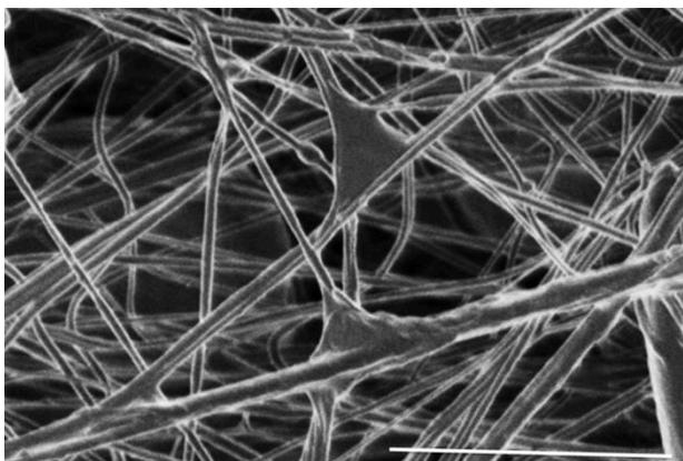
**Fig. 8: Scanning electron microscopy image of randomly oriented poly ( $\epsilon$  caprolactone) nanofibers containing 0.2 % retinoic acid (w/w) after 30 days of release studies. Scale bar is 4  $\mu$ m.**
