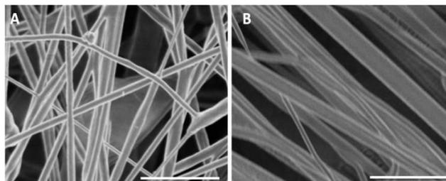
**Fig. 2: Scanning electron microscopy images of blank poly ( $\epsilon$  caprolactone) nanofiber scaffolds. (A) randomly oriented and (B) aligned poly ( $\epsilon$  caprolactone) nanofibers. Scale bar is  $4\ \mu\text{m}$ .**
