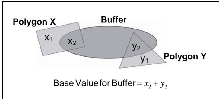
**Figure 3-4 Example illustrating the derivation of base values from overlaying polygons onto a buffer defined around a STH segment**
