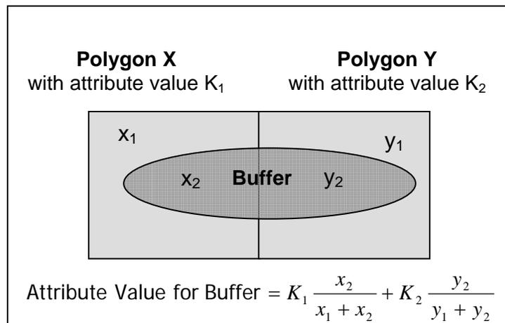
**Figure 3-6 Example illustrating the derivation of base values from overlaying zonal data onto a buffer defined around a STH segment**
