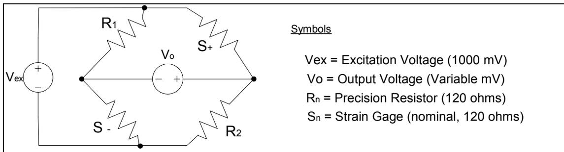
Figure 8. Schematic of Electrical Circuit showing connections that cancel bending strain.
