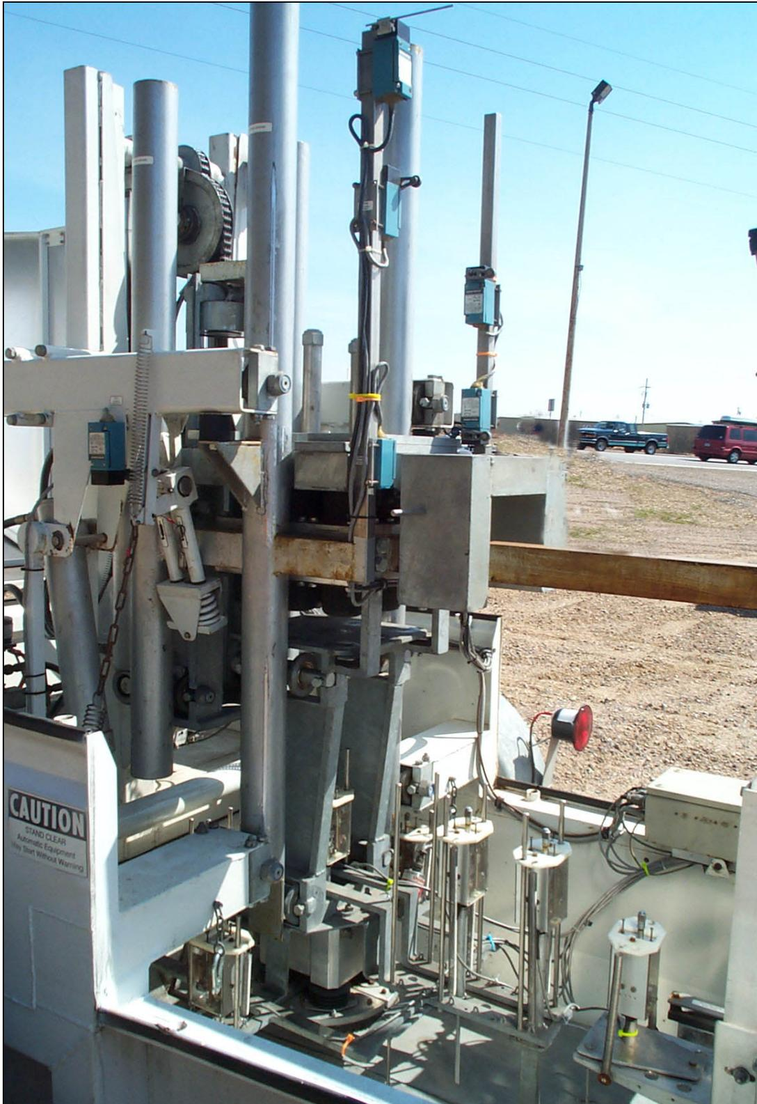
Figure 12. Left Side View with respect to Front of the FWD Showing LVDTs and Segmented Plate.
