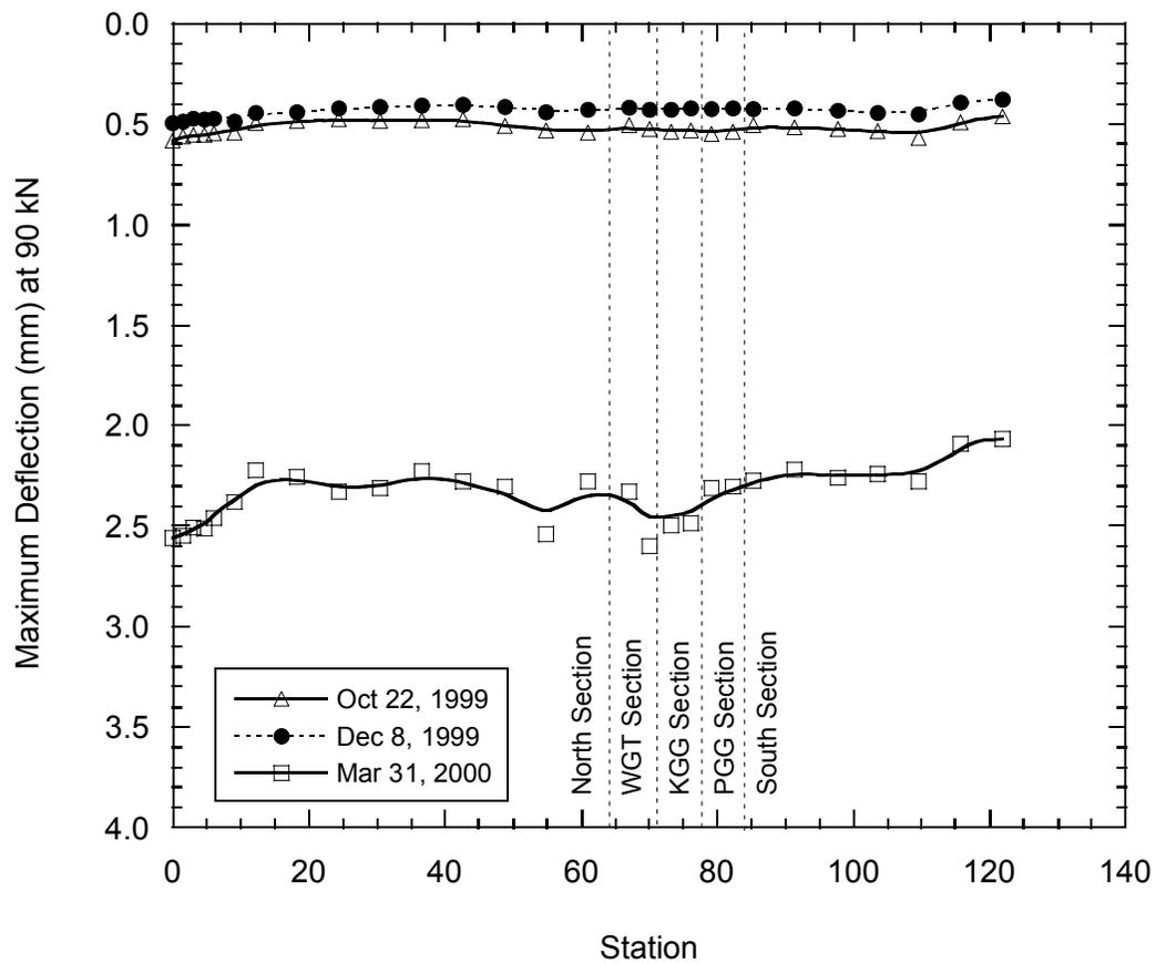
Figure 14. Maximum Deflection From Falling Weight Deflectometer Tests After Construction, Winter, and following Spring.
