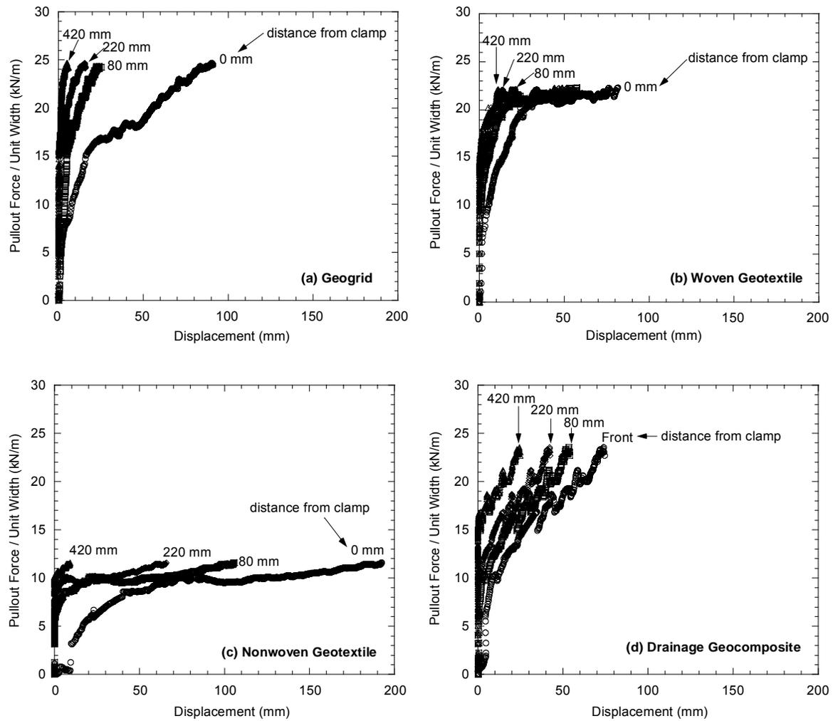
Fig. 3. Pull-out force vs. displacement at various points along the geosynthetic: (a) geogrid, (b) woven geotextile, (c) non-woven geotextile, and (d) drainage geocomposite.
