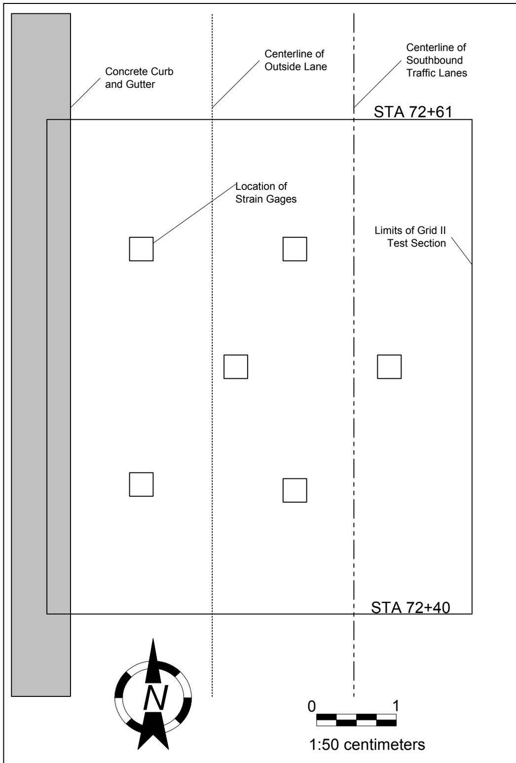
Figure 6. KGG Section Showing Strain Gage Location and Orientation.
