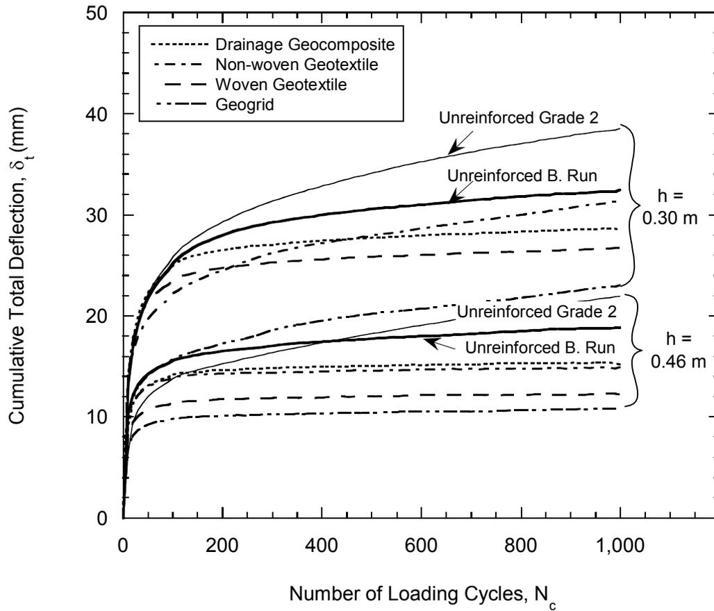
Fig. 5. Cumulative total deflection ( $\delta_t$ ) under the loading plate of the LSME as a function of number of load cycles for working platforms having thickness ( $h$ ) of 0.30 m or 0.46 m. Geosynthetic-reinforced working platforms were constructed with Grade 2 gravel.
