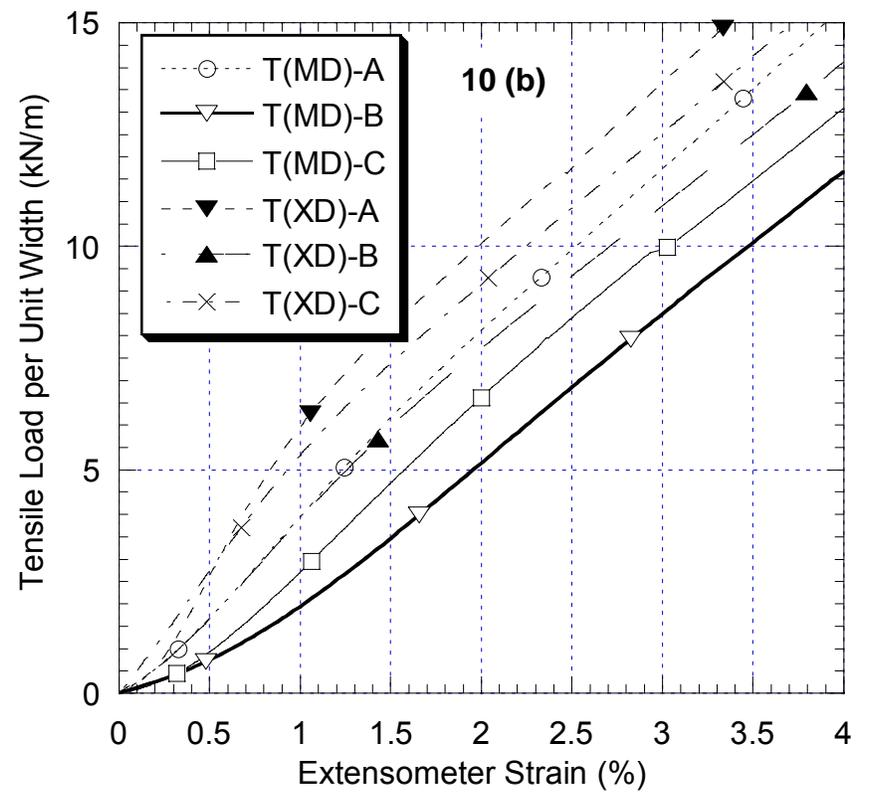
Figure 10a and 10b. Calibration and Correlation for Geotextile
