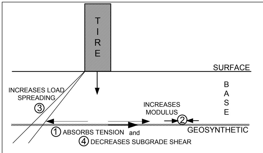
Figure 3. Lateral Restraint Function Showing Four Mechanisms of Improvement.
