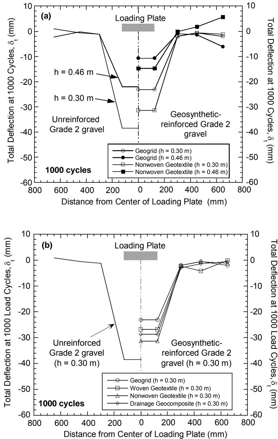
Fig. 6. Effect of layer thickness (a) and type of geosynthetic (b) on total deflection basins at 1000 load cycles.
