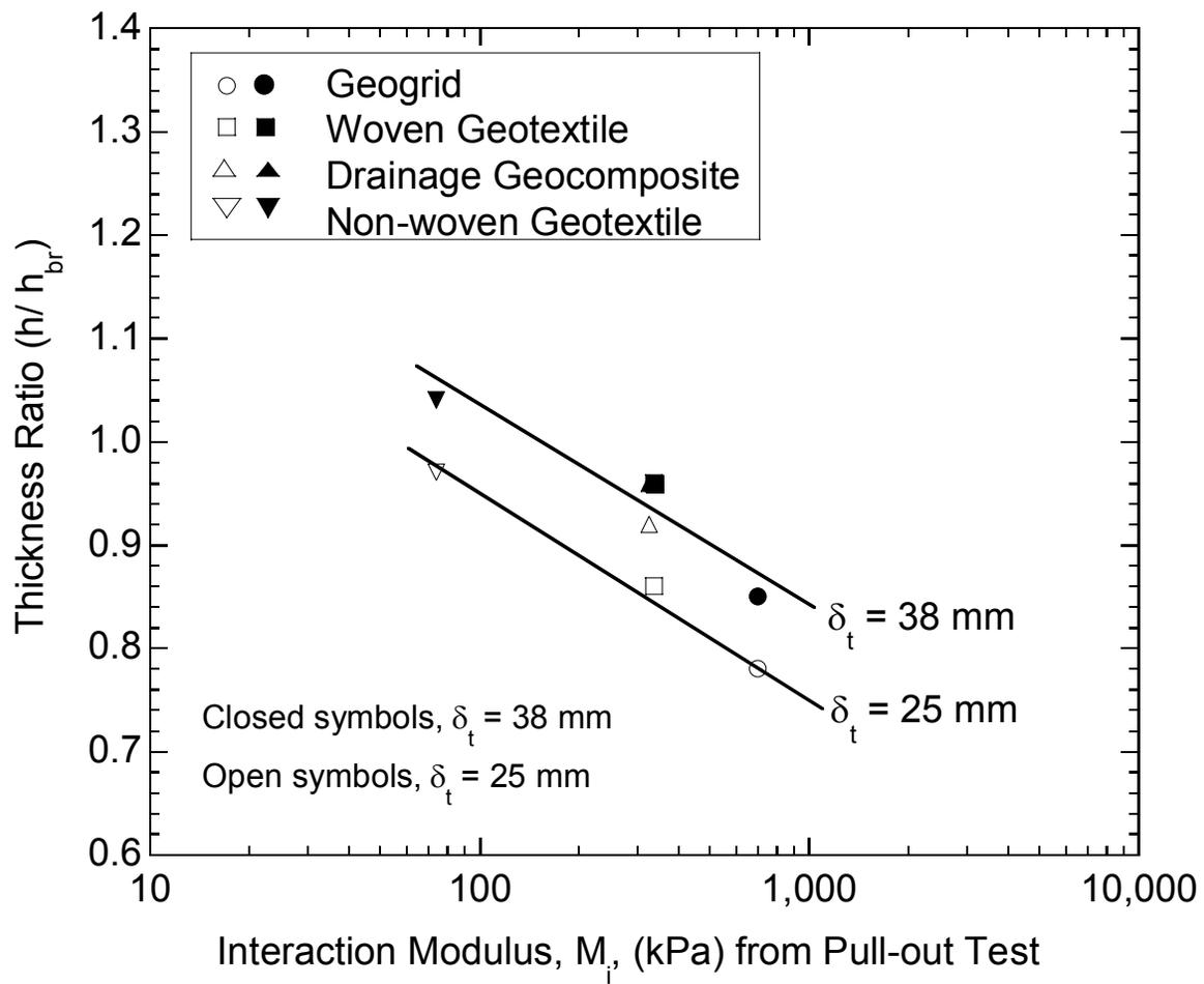
Fig. 9. Relationship between thickness ratio and interaction modulus for total deflections (at 1000 cycles) of 25 and 38 mm.
