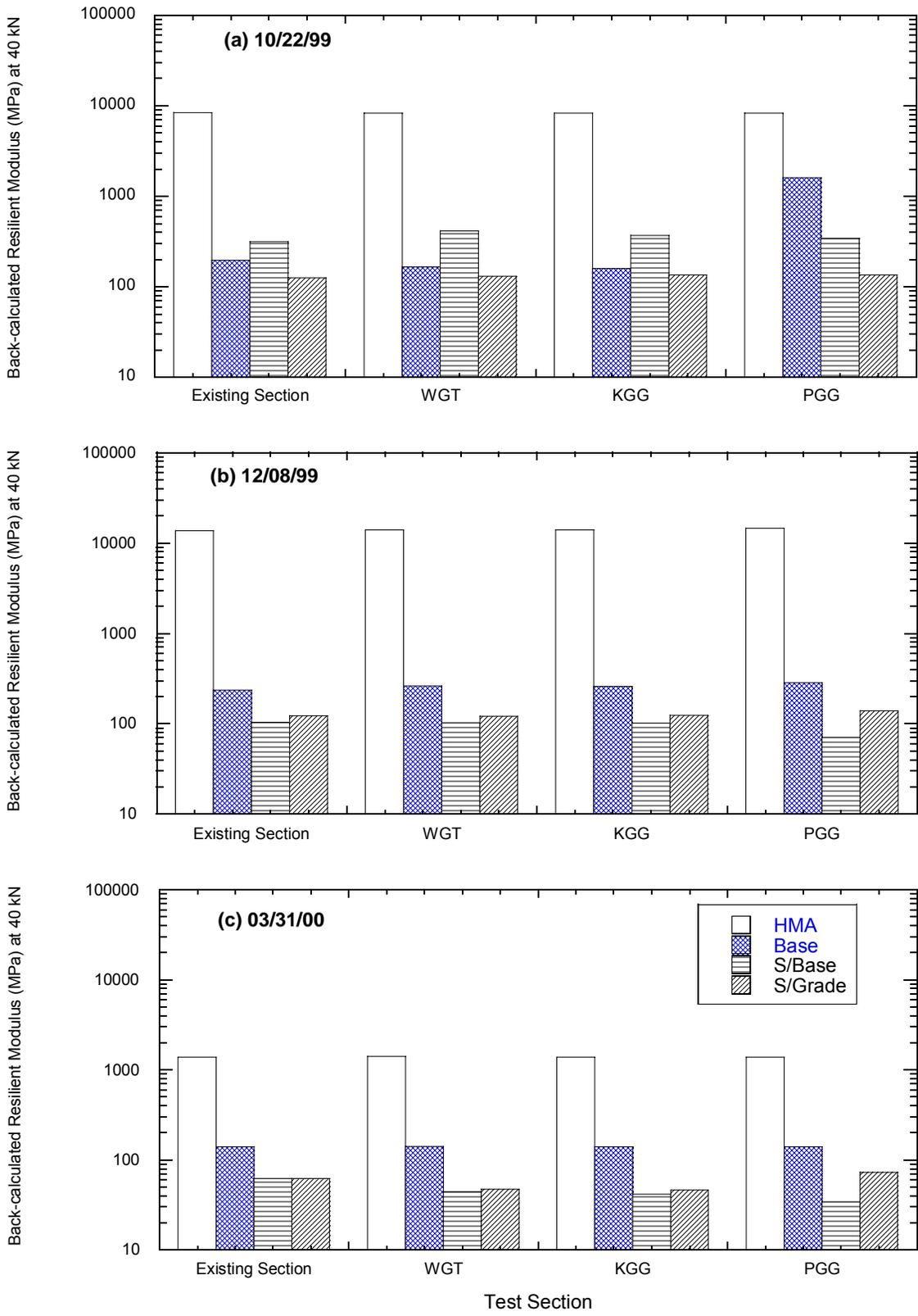
Figure 16. Back-calculated Modulus at 40 kN For Each Layer along USH 45 Test Sections.
