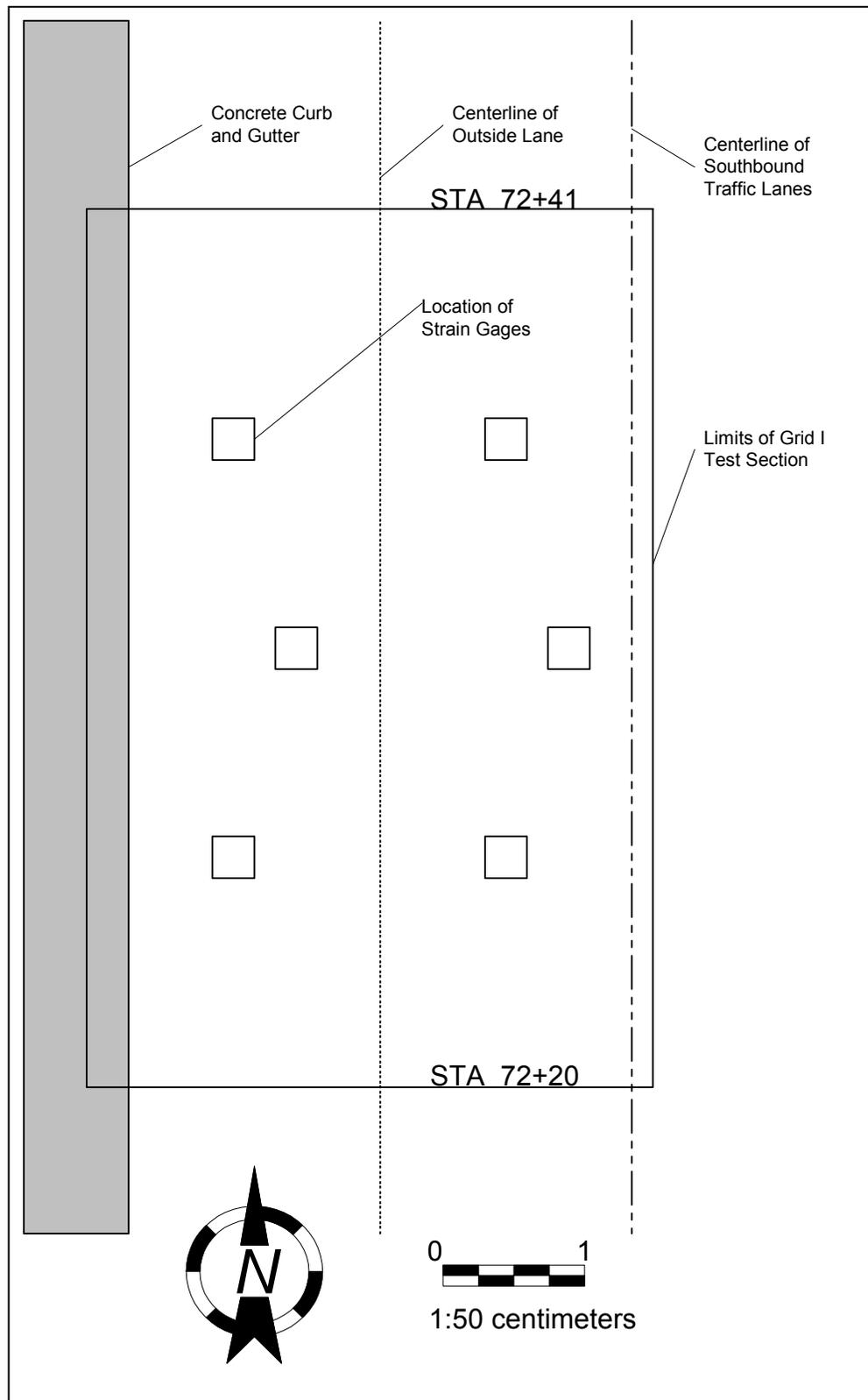
Figure 5. PGG Section Showing Strain Gage Location and Orientation.
