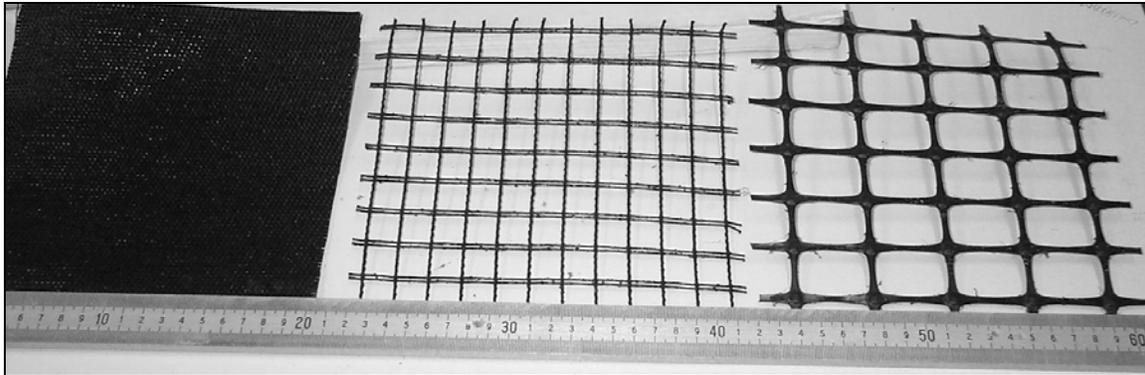
Figure 1. Picture of Geosynthetics: PGG, KGG, and WGT From Right to Left.
