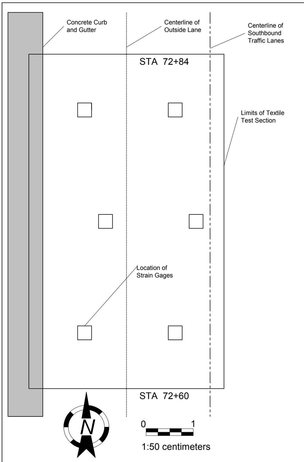
Figure 7. WGT Section Showing Strain Gage Location and Orientation.
