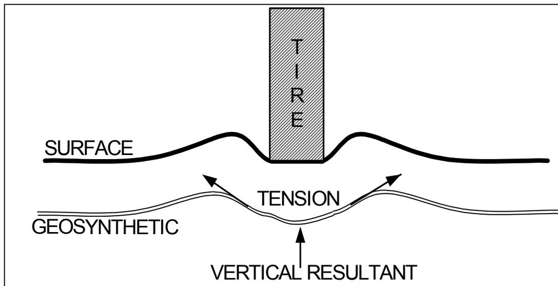
Figure 4. Tensioned Membrane Function Showing Displacement and Resultant Force.
