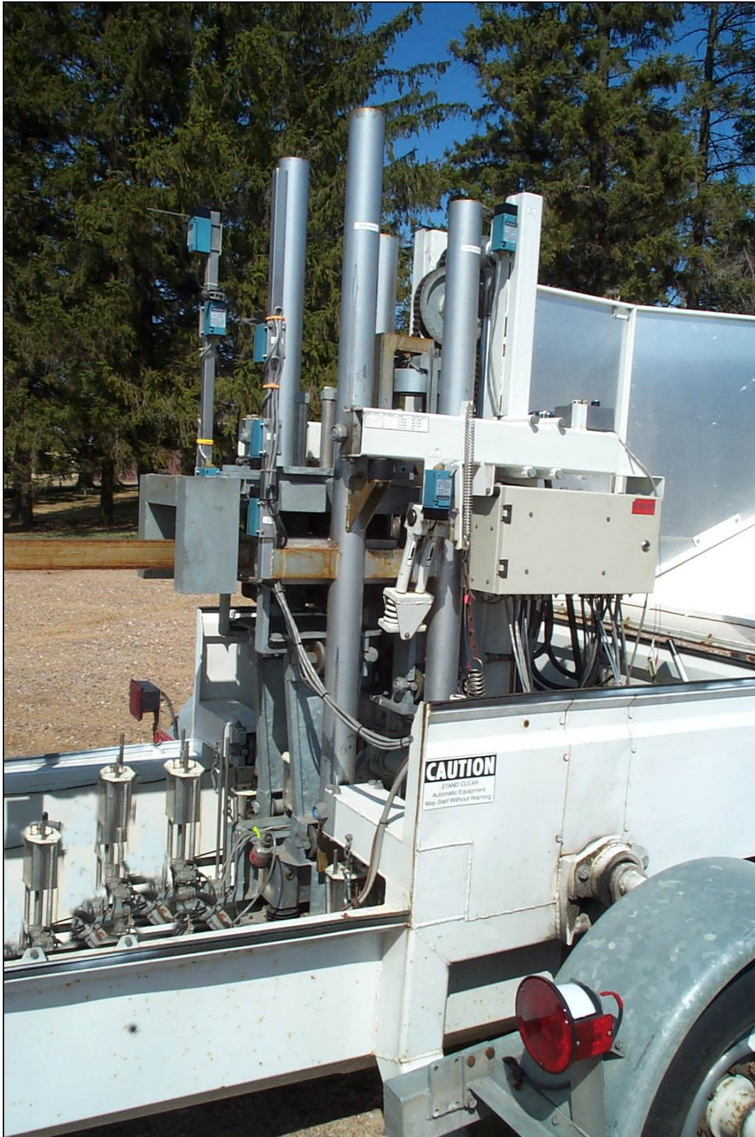
Figure 11. Right-hand Side View with respect to Front of the FWD Showing LVDTs and Load Frame.
