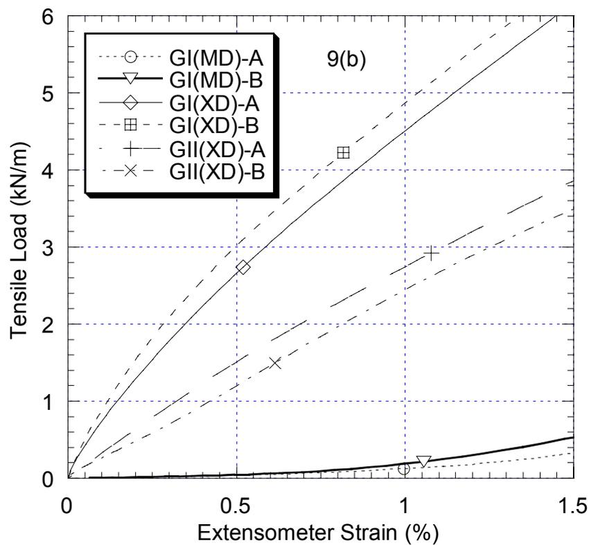
Figure 9a and 9b. Calibration and Correlation for Geogrids
