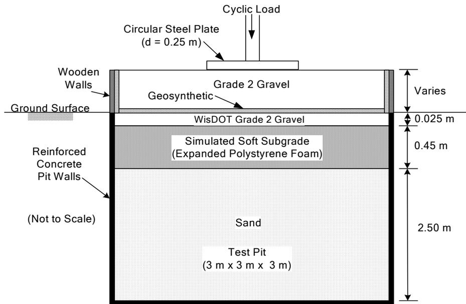
Fig. 4. Schematic of large-scale model experiment (LSME).
