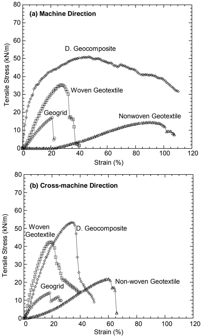
Fig. 2. Force-elongation curves from wide-width tensile tests on the geosynthetics: (a) machine direction and (b) cross-machine direction.
