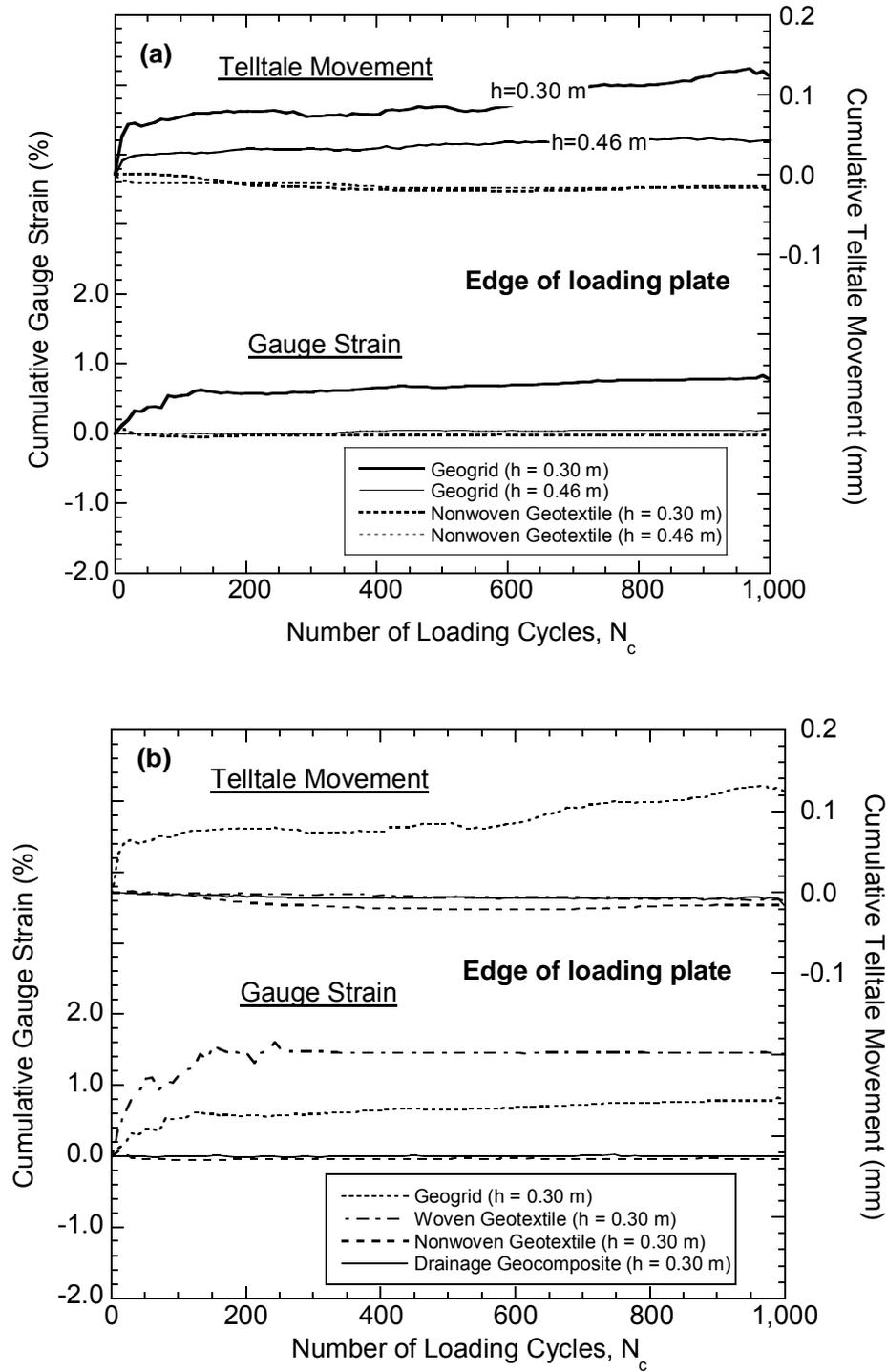
Fig. 7. Effect of layer thickness (a) and type of geosynthetic (b) on gage strain and telltale movement at the edge of the loading plate as a function of number of load cycles
