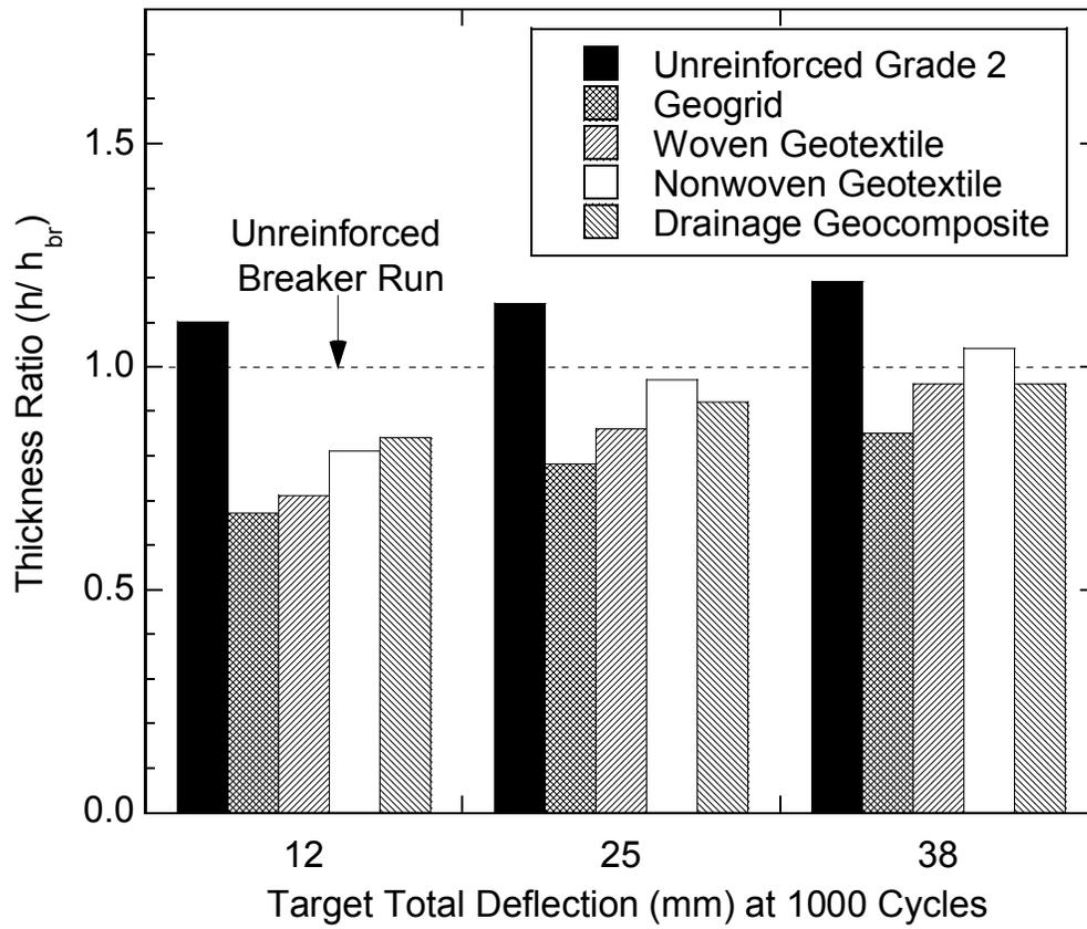
Fig. 8. Thickness ratio for each of the working platforms for total deflections (at 1000 cycles) of 12, 25, and 38 mm.
