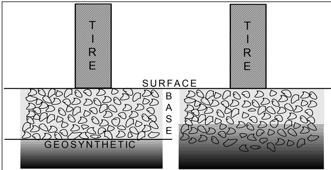
Figure 2. Separation Theory: separated (unmixed), left and mixed, right
