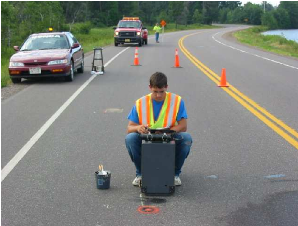
Figure 4.4 Conducting Air Permeameter Test with ROMUS Device
