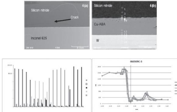
Fig. 4(a) Overview of a  $\text{Si}_3\text{N}_4/\text{Cu-ABA/W/Cu-ABA/Mo/Cu-ABA/Inconel}$  joint, (b) & (c)  $\text{Si}_3\text{N}_4/\text{Cu-ABA}$  interface and the corresponding elemental composition, and (d) Knoop microhardness distribution across the joint.
