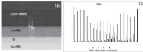
Fig. 3 (a) An optical photomicrograph of a multilayer  $\text{Si}_3\text{N}_4/\text{Cu-ABA}/\text{W}/\text{Cu-ABA}/\text{Ta}/\text{Cu-ABA}/\text{Inconel}$  joint showing interlayers and superimposed microhardness profiles, and (b) & (c) show the  $\text{Si}_3\text{N}_4/\text{Cu-ABA}$  interface together with the elemental composition at point markers of Fig. 3b.
