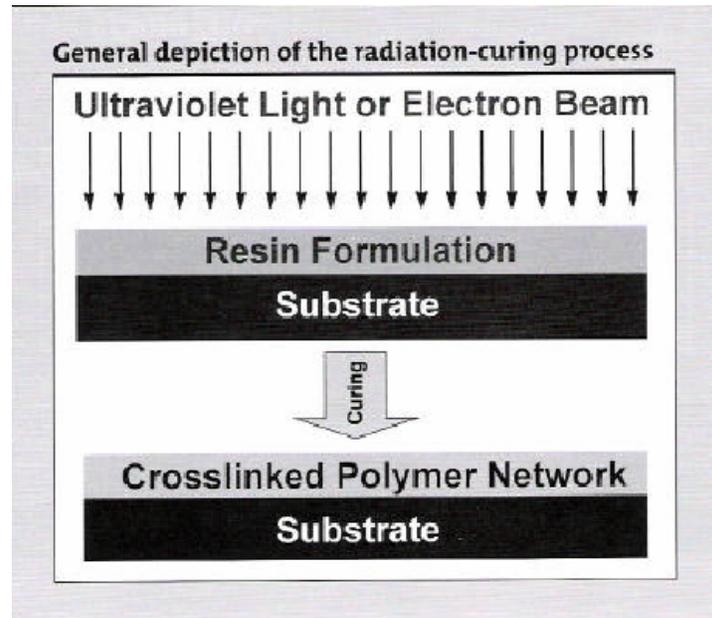
**Figure 2.** Radiation-Curing Process (Miller, 2005).
