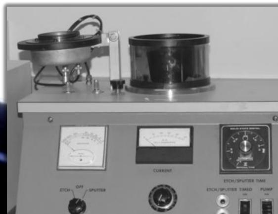
Figure 2: Sputter coater machine used to coat insects in metal prior to viewing through electron microscopes
